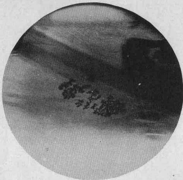
Figure 30 A Colombian emerald with a very unusual but interesting air-filled fracture exhibiting a dendritic pattern.
