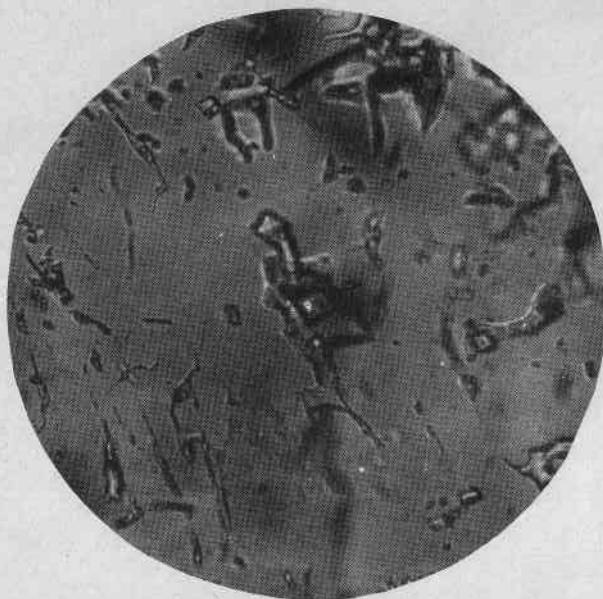
Figure 28 A Colombian emerald having an abundant distribution of smallest three-phase inclusions. The three-phase inclusions are most interesting, as they are cavities which contain the three phases of matter at once, that is, one or more crystals and one or more gas bubbles are bedded in liquid which fills the cavity.
