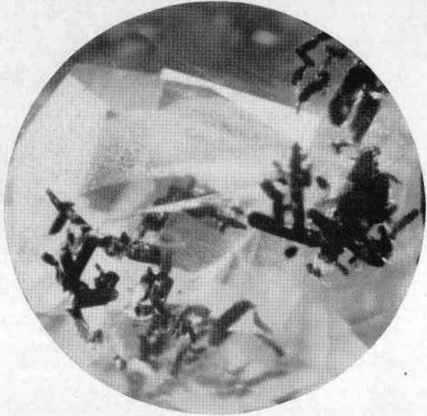
Figure 23 Burma ruby with in- clusions of coarse ru- tile needles.
