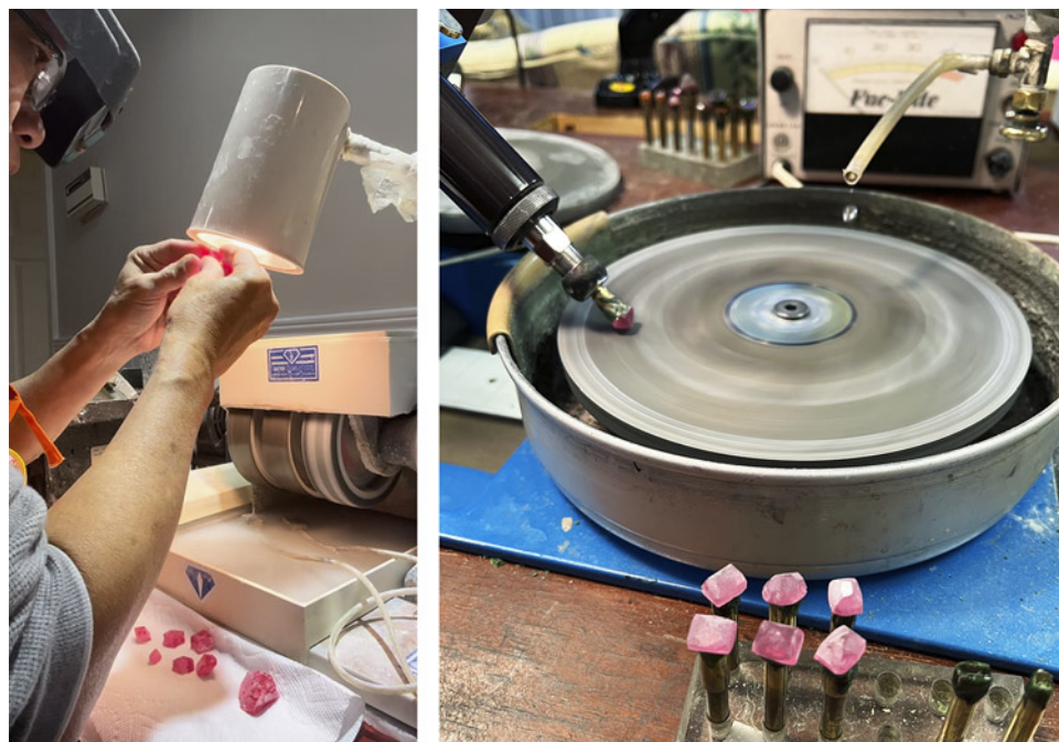
Figure 3. Converting a parcel of rhodochrosite rough into finished gems, from inspecting and grinding the rough (left) to the preformed and dopped rough (right). Courtesy of Ben Kho.
