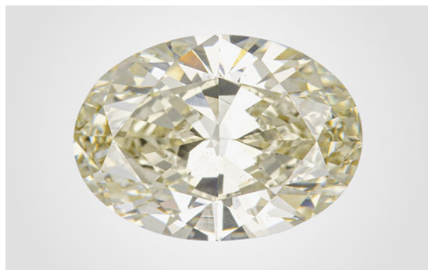
Figure 6. This 3.07 ct HPHT-treated CVD-grown diamond received a color grade of brownish greenish yellow, with the causes of color including isolated nitrogen and SiV - centers. Photo by Diego Sanchez.
