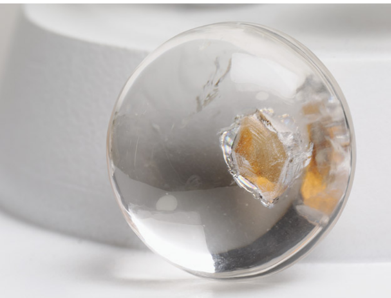
Figure 6. This orange inclusion in quartz (left) with a striated bipyramidal structure was identified as lithiophilite (right). Photos by Wingtak Lui (left) and Liyan He; field of view 13.0 mm (right).
