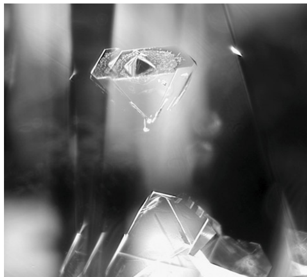
Figure 2. Left: Viewed from the pavilion of the 2.57 ct diamond, this transparent crystal inclusion with mirror image reflection resembles the profile of a faceted diamond under darkfield lighting. Image captured in monochrome; field of view 0.88 mm. Right: Using fiber-optic lighting, the crystal inclusion that appears opaque in the left image is displayed as a yellow octahedron; field of view 0.40 mm. Photomicrographs by Yagnesh Vyas (left) and Hemal Trivedi (right).
