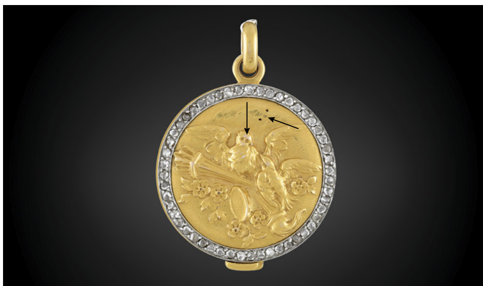
Figure 5. In this gold-plated pendant submitted as 18K solid gold, the base layer tested 10K and the top layer tested 18K. Arrows show where the gold plating has rubbed off due to use. Photo by Diego Sanchez.
