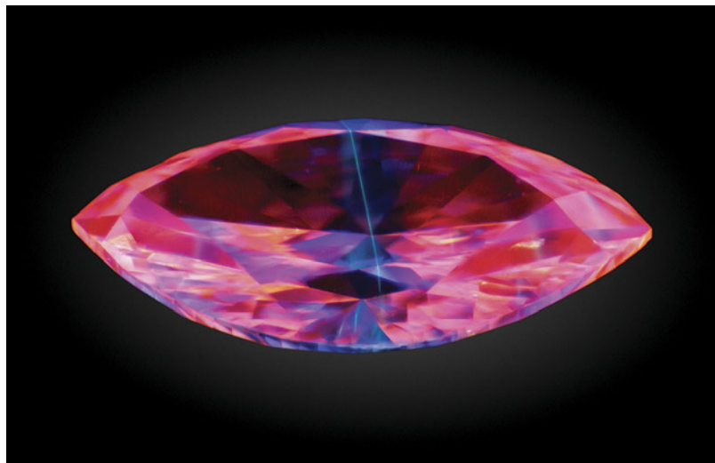
Figure 20. Deep-UV imaging of the 0.07 ct multilayered laboratory-grown diamond ( 4.20 \times 2.26 \times 1.27 mm) showing fluorescence of a thin blue-green layer between two pink-orange CVD layers. Image by Sean O'Neal.
