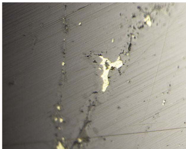
Figure 3. Left: A surface-reaching fracture in gadolinite observed with fiber-optic illumination. The fracture is filled with a reflective material. Right: The same fracture observed under reflective lighting. The yellowish fracture-filling material shows a metallic luster. Photomicrographs by Yusuke Takamura; field of view 1.04 mm.
