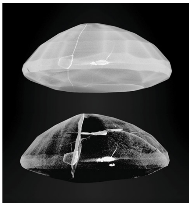
Figure 6. 3D rendering of a lead glass-filled ruby, with different contrast highlighting the opaque lead glass areas inside the gem.
