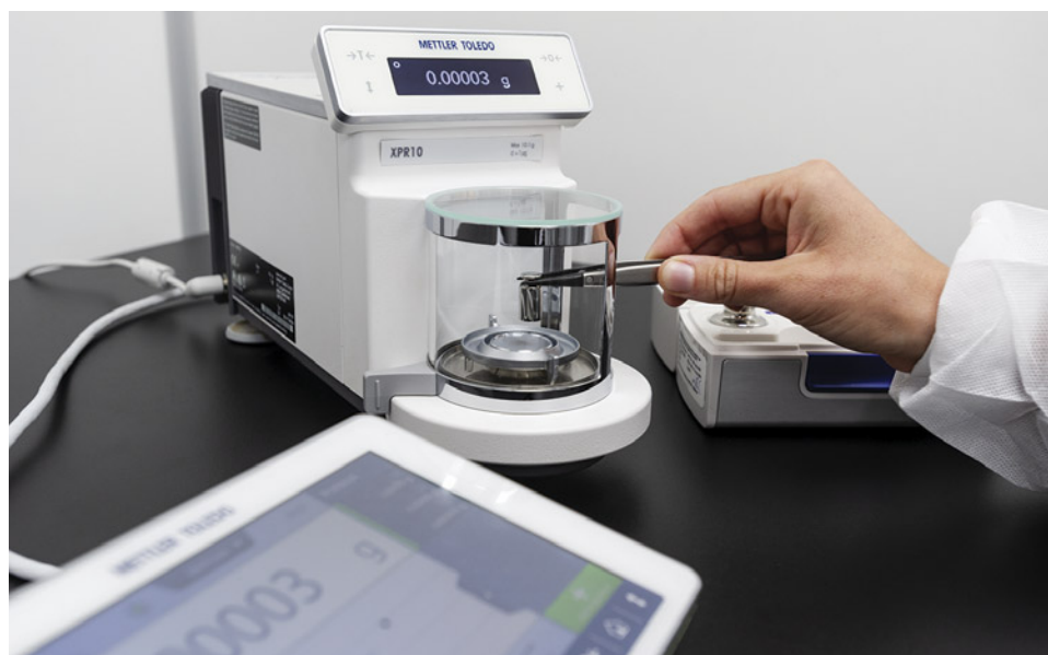
Figure 5. A GIA metrologist uses a calibrated standard to verify instrument performance. Photo by Kevin Schumacher.
