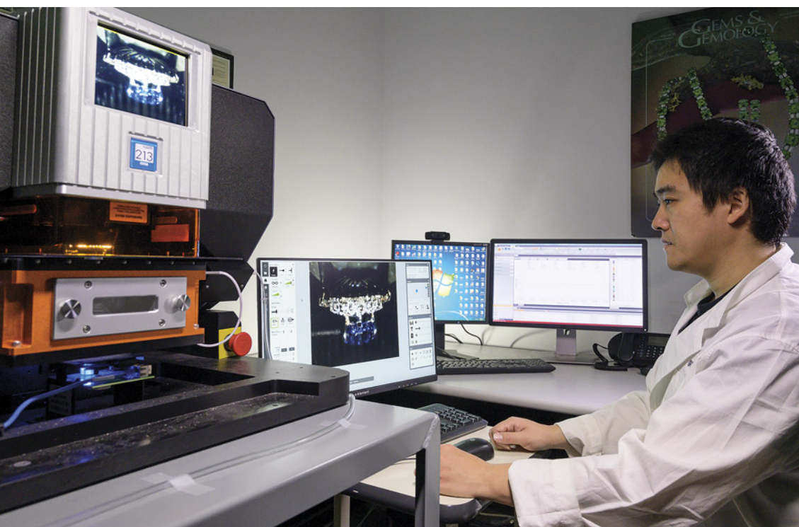
Figure 12. GIA’s laser ablation–inductively coupled plasma–mass spectrometry (LA-ICP-MS) system for chemical analysis of small spots on the surface of polished gemstones. Photo by Kevin Schumacher.
