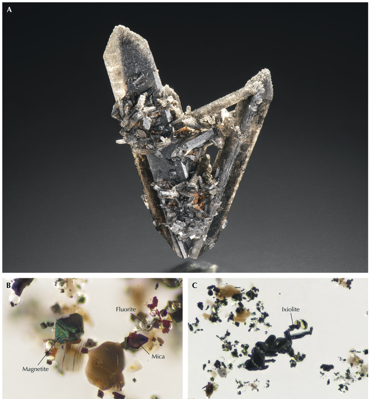
Figure 19. A: A black topaz crystal specimen from the Thomas Mountains in Utah, measuring 24.80 \times 17.92 \times 12.29 mm. Photo by Kevin Schumacher. B: Inclusions of black magnetite, colorless fluorite, and flaky mica in the black topaz. C: Clusters of tabular ixiolite. From Muyal et al. (2019); fields of view 0.288 mm (B) and 0.36 mm (C).
