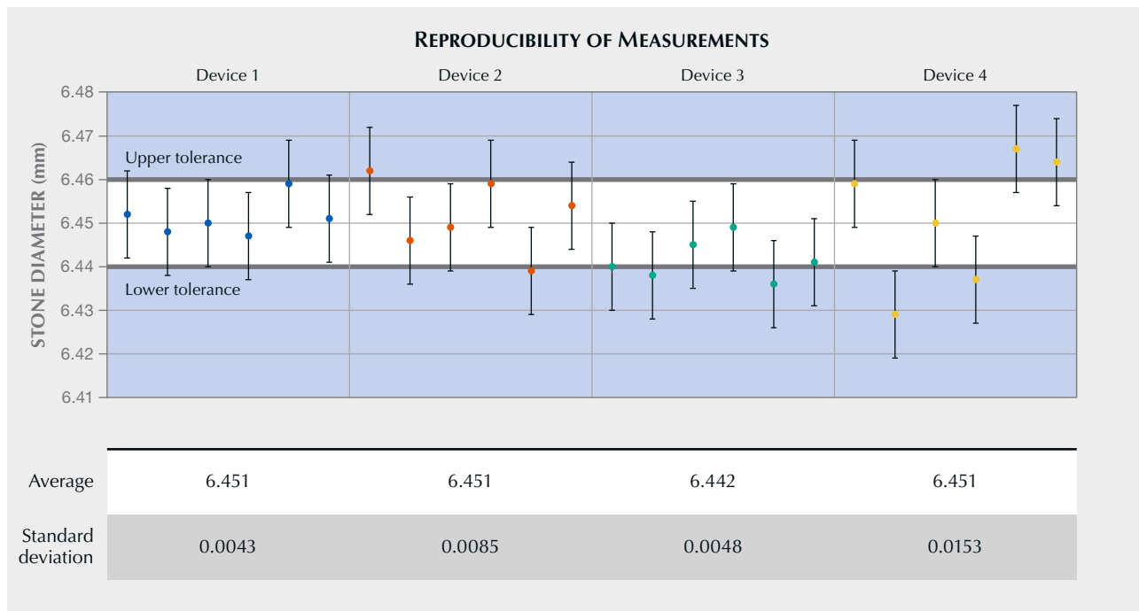
Figure 3. These four examples demonstrate the reproducibility of measurements for the maximum diameter of the same reference stone. Each device yields the same average value (within tolerance), but the four devices are not equally reliable. For Device 1, all six measurements are within the set tolerance of \pm 0.010 . Device 2 shows greater variability and might need attention if the issue persists. Device 3 shows a small standard deviation, but the noticeable decline in the values suggests a calibration problem. For Device 4, the variability is unacceptably large.
