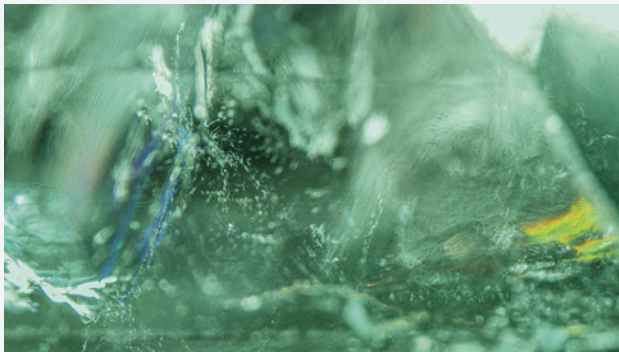
Flash effect seen in feathers, providing evidence of clarity enhancement; field of view 2.90 mm.
