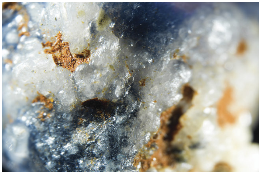
Figure 5. A resin imitation of matrix on the surface of a laboratory-grown sapphire. Field of view 7.19 mm.
