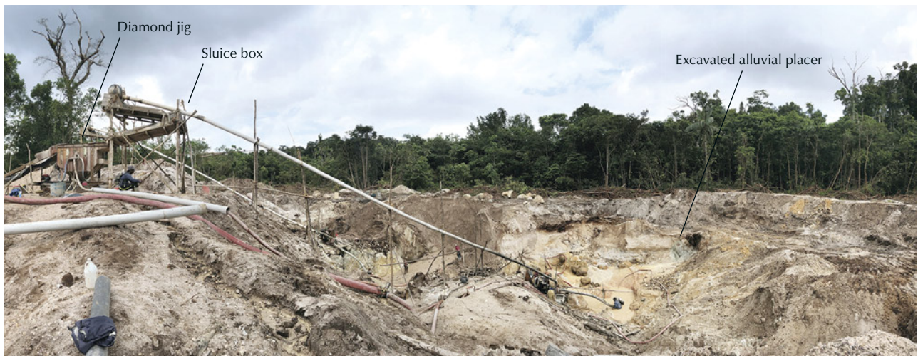
Figure 12. A typical small- to medium-scale diamond mining operation in Guyana using a diamond jig attached to a sluice box. Photo by Roy Bassoo.
