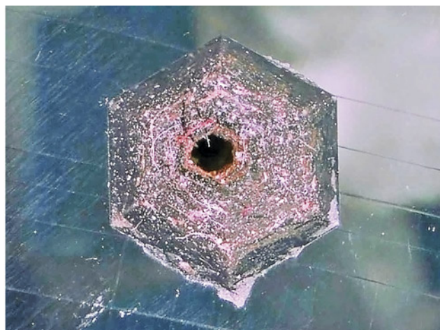
Figure 3. The etch features of the crystal: two hexagonal dissolution cavities connected by a hexagonal etch channel. The channel (left) is about 4 cm long and empty throughout, and the openings have a hexagonal funnel shape (right). Photomicrographs by Chao Liu (left; field of view 23 mm) and Ting Zheng (right; field of view 6.25 mm).
