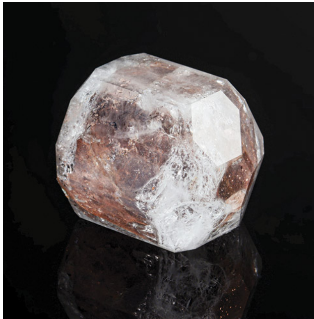
Figure 12. Doubly terminated flux synthetic beryl crystal, measuring 32.45 × 30.36 × 25.29 mm. Photo by Annie L. Haynes.
