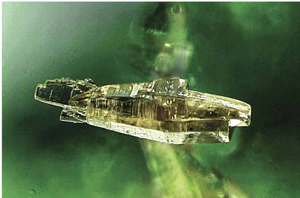
Figure 11. Parasite inclusions in emerald are a diagnostic indicator of a Colombian origin. Photomicrograph by Jonathan Moyal; field of view 0.82 mm.
