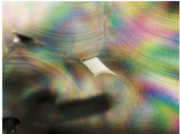
Figure 14. This fluid inclusion contains mostly a gaseous phase. It is trapped at the intersection of curved botryoidal growth zones and presents high-order interference colors obvious between crossed polarizers. Photomicrograph by U. Hennebois; field of view 1 mm.
