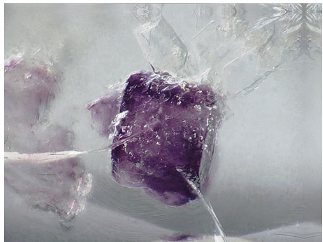
Figure 12. Purple fluorite cube, identified by micro-Raman spectroscopy, in a hyalite. Photomicrograph by U. Hennebois; field of view 1.2 mm.
