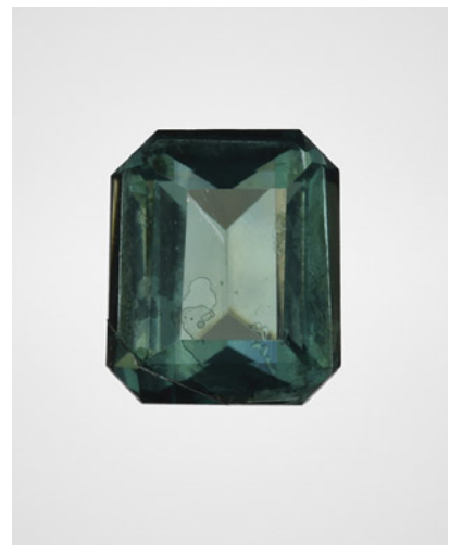
Figure 13. Flattened gas bubbles caught in the break of a filled fracture are visible face up in this 1.43 ct repaired grandidierite.
