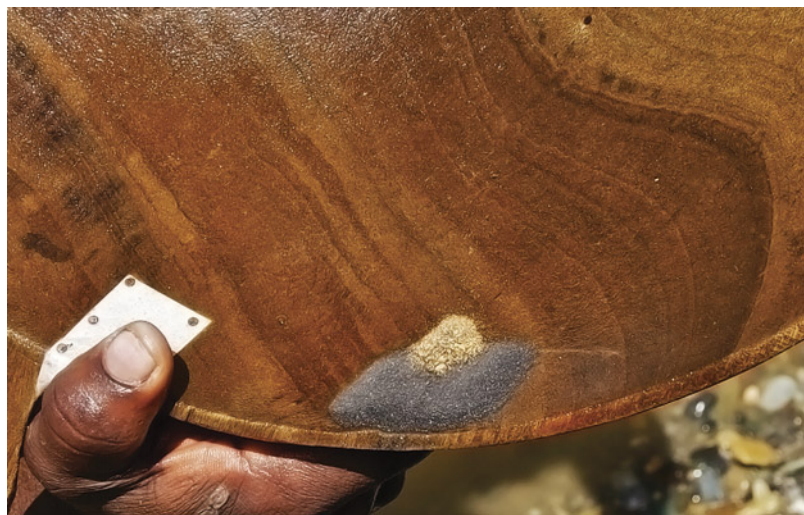
Figure 53. Gold and dense black sands in a traditional wooden batea, shown by a Colombian miner at Oro Verde. Typically, mercury is used to separate the two materials. Photo courtesy of Toby Pomeroy.
