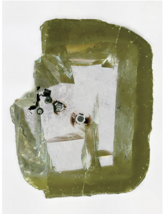
Figure 72. The polished slab of the diamond containing davemaoite showing the round spots where the grains were excavated for LA-ICP-MS analysis. Photo by Aaron Celestian.
