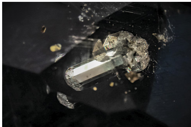
Figure 2. A hexagonal apatite inclusion with interference colors in smoky quartz, viewed in cross-polarized illumination. Photomicrograph by Nattapat Karava; field of view 6.3 mm.
