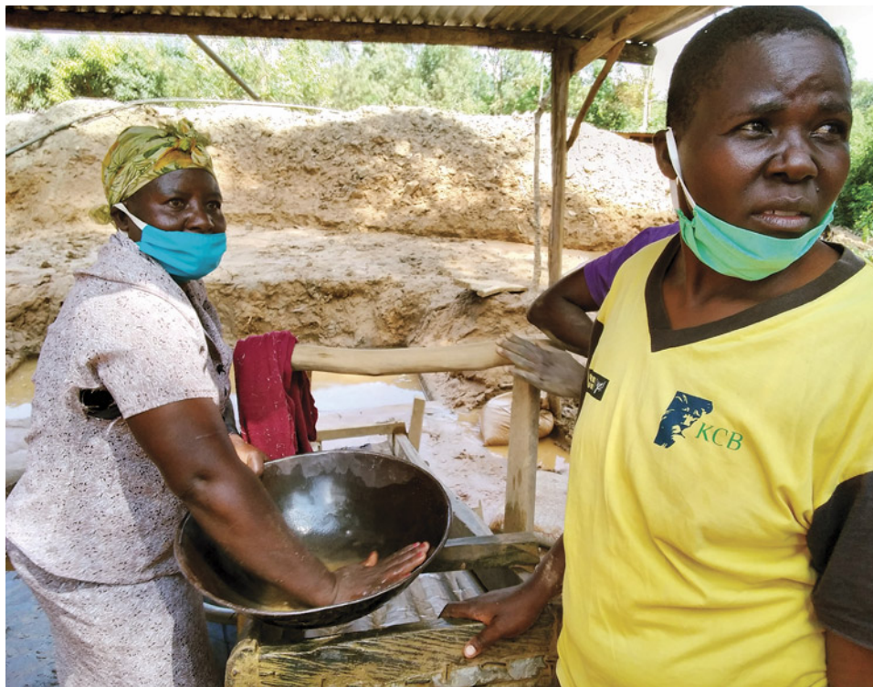
Figure 54. In this photo from November 2020, Kenyan miners in Kakamega County press amalgam in a pan to remove excess water. Amalgam is a mixture of mercury and gold produced by adding mercury to concentrated gold ores. This method puts miners in direct contact with mercury, a potent neurotoxin that can be absorbed through the skin. Photo courtesy of Ruth Epwoka.
