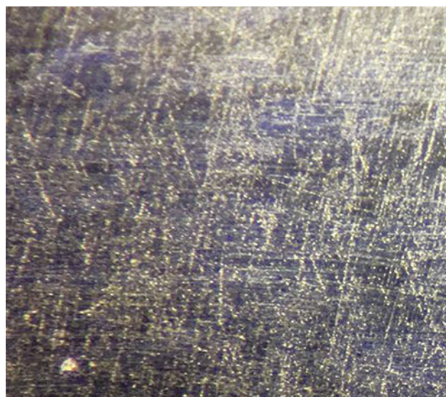
Figure 69. Needle-like inclusions arranged in four directions, viewed here from the top of the stone, created the asterism effect in the Vietnam topaz. Photomicrograph by Le Ngoc Nang.
