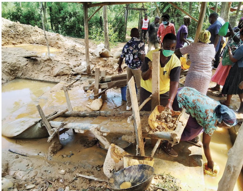
Figure 55. Miners wash the gold ores and use a sluice to collect gold within the slurry. Sluices are one of the most common tools used in artisanal and small-scale mining to concentrate gold. This simple configuration can capture ~20–70% of gold based on ore type, water flow, feed rate, and other specifications geometalurgists determine through research. Photo courtesy of Ruth Epwoka.
