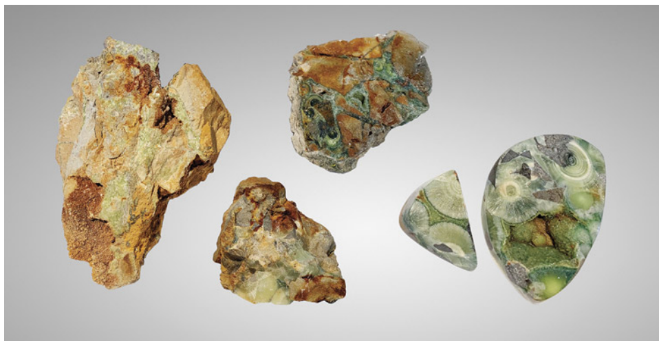
Figure 30. Left to right: Wavellite rough before treatment, stabilized rough, a slab of stabilized rough with all the waste host rock trimmed off, and two pieces of polished stabilized wavellite cabochons (89 and 405 ct, respectively). Photo by Tao Hsu; courtesy of Unconventional Lapidarist.
