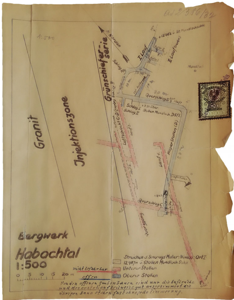
Figure 17. One piece of evidence introduced in legal proceedings in 1932 was a map of the Habachtal mine apparently prepared by copying and coloring the map drawn by Anton Hager Jr. in 1924 and updated in 1926. The C gallery (red) was not accessible at the time, while the D gallery (blue) could be accessed. File “Beryl-emerald-Habachtal,” Montanbehörde West, Salzburg.
