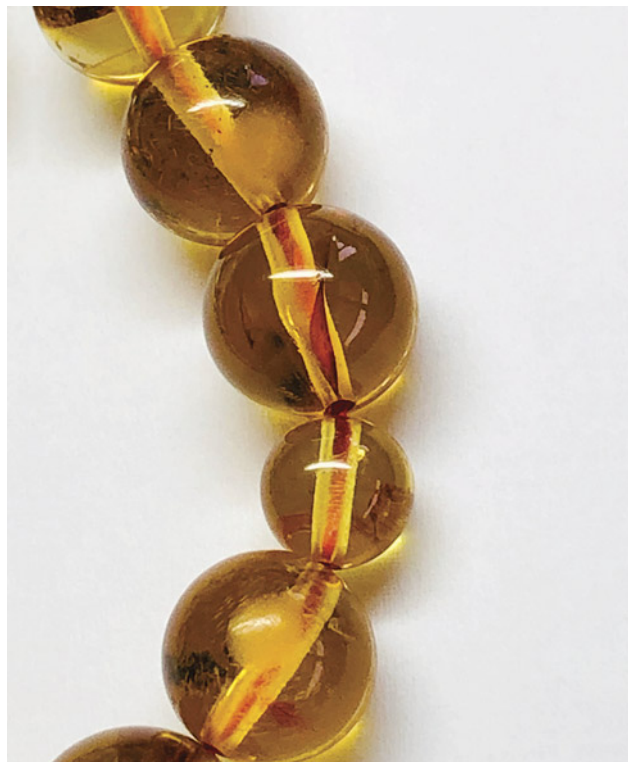
Figure 82. Epoxy resin is easily detected in the amber of this rosary. Photo by Nazar Ahmed Ambalathveettil.
