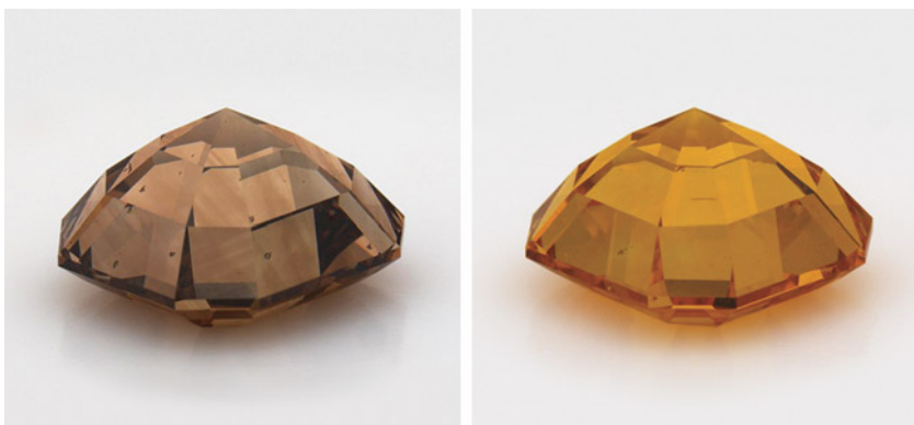
Figure 2. Table-down images showing the diamond before HPHT treatment (left) and after (right).
