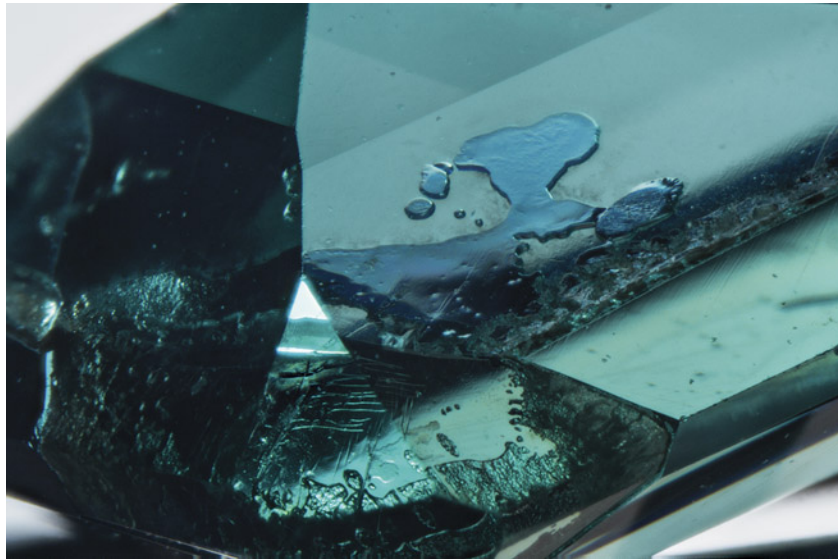
Figure 14. Flattened gas bubbles caught in the filling of the large fracture that breaks continuously through the entire pavilion and some of the crown. Field of view 4.79 mm.
