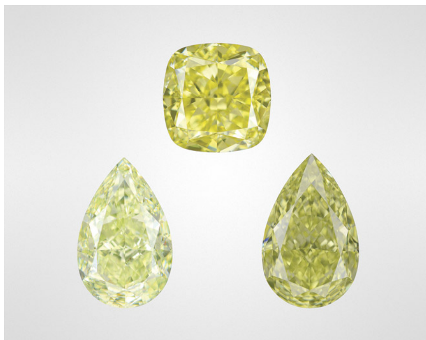
Figure 6. Large gem diamonds with strong color saturations resulting from nickel-related impurities. Top: 5.02 ct Fancy Intense green-yellow cushion. Bottom left: 5.03 ct Fancy yellow-green pear. Bottom right: 5.06 ct Fancy Intense green-yellow pear.
