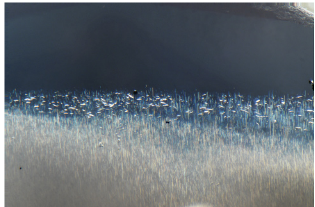
Figure 2. A myriad of inclusions at the boundary between the dense, silky core and the unincluded rim. Photomicrograph by Jonathan Moyal; field of view 1.76 mm.
