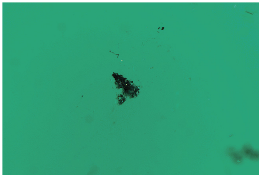
Figure 8. Opaque black grains were also observed, consistent with inclusions observed in emeralds from Colombia. Field of view 1.26 mm.
