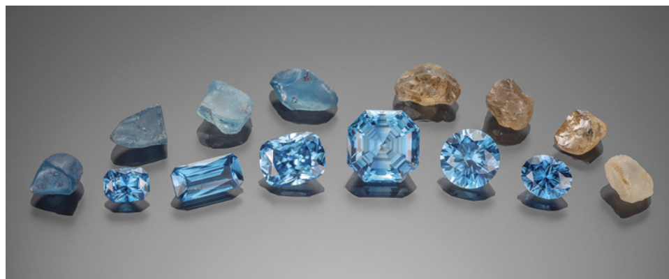
Figure 10. This suite of zircons, reportedly from Malawi, shows unheated brown starting material, examples of rough material after heat treatment, and six examples of faceted stones (the largest stone weighs 7.70 ct). Photo by Diego Sanchez; courtesy of Phoenix Gems.
