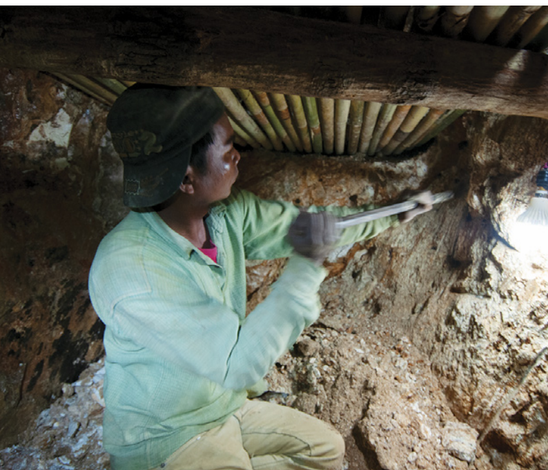
Figure 9. There are a few sapphire mines in Mogok where people extract the blue gems directly from the host rock. Following underground tunnels, they trace gem-rich zones. In many places, the rock is fairly weathered and manual tools are sufficient. On rarer occasions, blasting is required in the sapphire mines. Photo by Wim Verriest.
