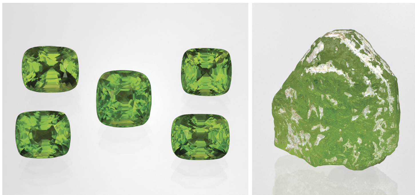
Figure 1. Left: Five faceted peridot samples from the Pyaung-Gaung mine in Mogok, Myanmar, weighing 5.18–7.52 ct, were examined in this study. Right: This 15.0 × 16.9 × 6.5 mm rough crystal showing a rhombus-shaped tabular habit and rounded faces, with minor white carbonate and talc, is also from the Pyaung-Gaung mine. Photos by T. Sripoonjan.
