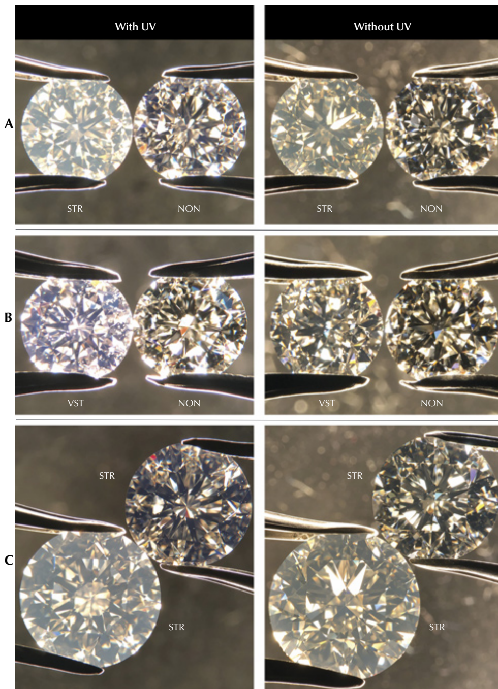
Figure 10. Sets of diamonds with different UV intensities were examined and imaged under microscope darkfield illumination, with and without UV content.
