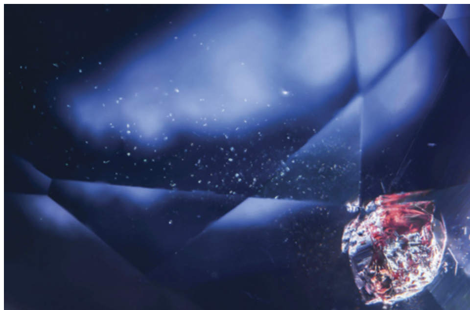
Figure 4. This sapphire contains a beautiful garnet inclusion and a trail of dust-like rutile particles. Photomicrograph by Michaela Stephan; field of view 4.79 mm.
