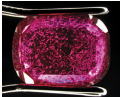
Figure 16. Densely distributed amphibole inclusions in ruby. Field of view 9.40 mm.
