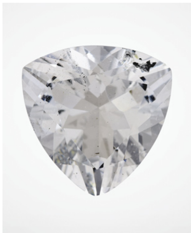
Figure 9. This 7.17 ct colorless sodalite was remarkably transparent and contained interesting fluid inclusions. Photo by Sean-Andrew Z. Pyle.
