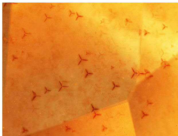
Figure 9. A group of windmill-like inclusions with orange color concentrations observed in sphalerite. Photomicrograph by Ungkhana Atikarnsakul; field of view 3.1 mm.
