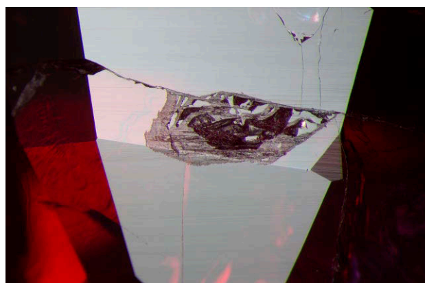
Figure 2. A large area of a foreign substance cut through on the surface of a ruby from the Montepuez area of Mozambique. This substance infilled not only this cavity but also many narrow fissures in the stone. Micro-Raman analysis identified it as böhmite. Dark-field + diffuse overhead illumination. Photomicrograph by Richard W. Hughes; field of view 3 mm.
