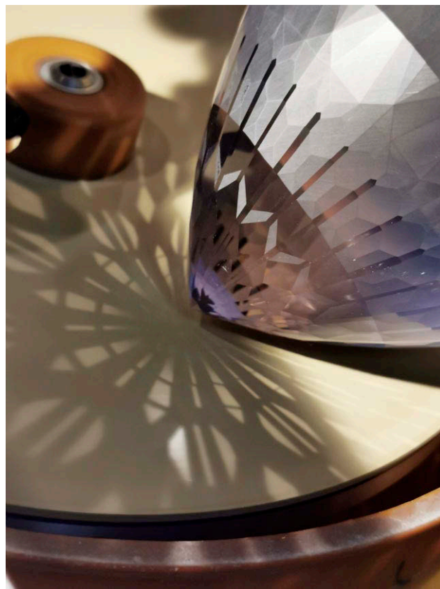
Figure 13. The polishing step on the stone's pavilion begins to show the intricate optical effects of the completed piece. Photo by Victor Tuzlukov.
