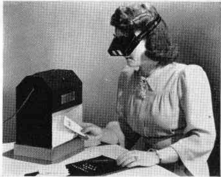
Figure 2 Grading a group of stones on the Diamolite
