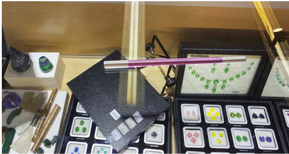
Figure 52. Synthetic ruby rod grown by the flame-fusion technique showing chromium-free ends. Photo by Jennifer Stone-Sundberg; courtesy of RusGems.
