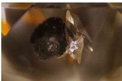
Figure 1. This 0.70 ct natural diamond contained an inclusion of wollastonite and CaSiO 3 -breyite with a large disk-like graphitic fracture due to exhumation from the mantle. Field of view 1.15 mm.
