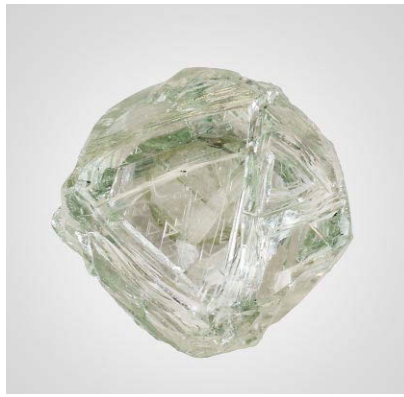
Figure 5. The 0.62 ct green “Matryoshka” diamond ( 4.8 \times 4.9 \times 2.8 mm) from Siberia has an internal open cavity connected by two small channels to the outside. The surface is covered by etched trigons and striations. A small diamond crystal can move freely inside the cavity.
