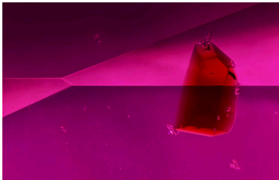
Figure 10. Viewed with darkfield illumination, a transparent brownish red crystal inclusion clearly stands out, even in a ruby matrix. This is believed to be the first staurolite inclusion found in corundum. Photomicrograph by E. Billie Hughes; field of view 2 mm.
