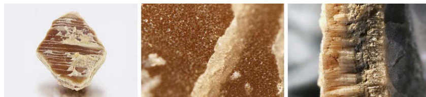
Figure 27. Left: Clear striations are visible on the back of the shell blister (measuring approximately 24.4 \times 18.6 \times 6.5 mm). Center: Cellular crystal growth patterns are evident on the back of the shell blister. Right: Columnar growth structures are prominent with the cross section of the shell fragment.
