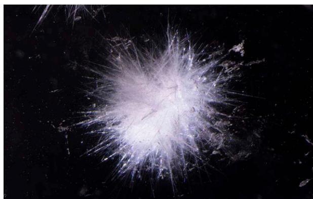
Figure 2. Clusters of white radial needles of the mineral bavenite were seen in this 233.60 ct quartz. Photomicrograph by Nathan Renfro; field of view 13.43 mm. Courtesy of Mike Bowers.
