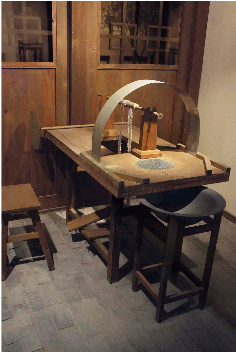
Figure 2. A restoration of a fourth-generation table-type iron rotary machine. The artisan sits at the table and carves the jade using the rotary tool and abrasive sands, driven by the foot treadle. Photo by Mingying Wang, from Tianjin Museum.
