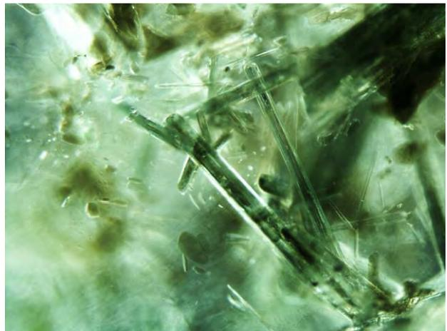
Figure 28. Greenish rod-like inclusions identified as amphibole in Zambian emerald. Photomicrograph by Nattida Ng-Pooresatien; field of view 1.6 mm.
