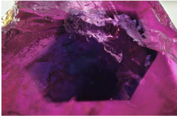
Figure 10. This deep blue hexagonal core is a telltale sign of an unheated Mong Hsu ruby's provenance. However, unheated Mong Hsu rubies are rarely encountered in the trade. Photomicrograph by Jonathan Moyal; field of view 4.79 mm.
