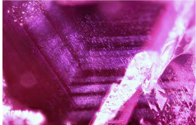
Figure 22. Fine particulate clouds arranged in a hexagonal pattern are often seen in Afghan rubies. Photomicrograph by Jonathan Moyal; field of view 1.8 mm.
