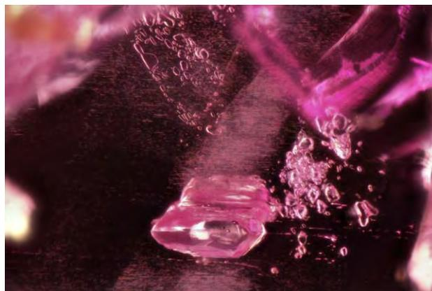
Figure 5. Dense concentrations of silk accompanied by rounded calcite crystals suggest a Burmese origin. Photomicrograph by Jonathan Moyal; field of view 1.99 mm.
