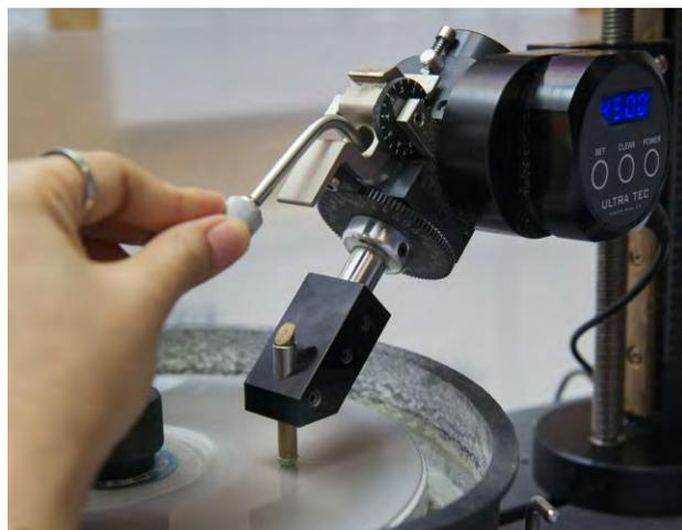
Figure 12. Before a sample can be analyzed, it must be prepared. This preparation involves polishing large, flat windows on the stone with a minimum of polish lines. This can be achieved using precision cutting machines. Photo by Nuttapol Kitdee.
