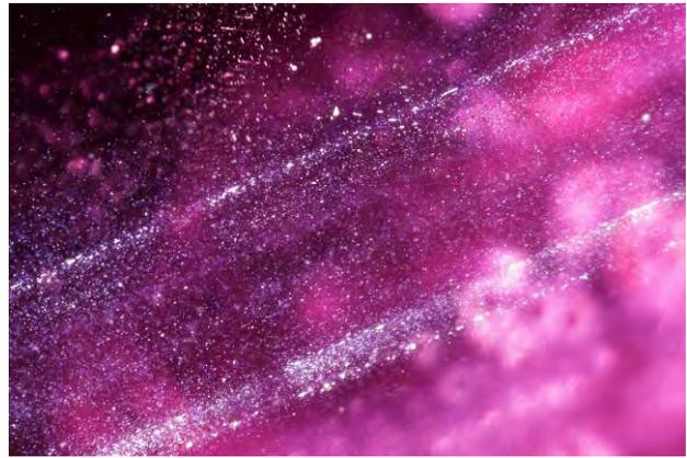
Figure 30. Small, often dusty groups of particles without a well-defined geometric pattern can be observed in Tajik rubies, but they may be difficult to distinguish from those seen in Afghan rubies. Photomicrograph by Charuwan Khowpong; field of view 2.5 mm.
