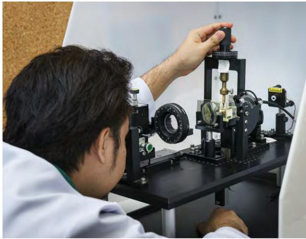
Figure 13. Selected samples with very high clarity are often aligned to the c-axis using this custom-built instrument. Aligning all samples allows for a precise characterization of the wavelength absorption in certain directions and guarantees that different samples can be compared. Photo by Nuttapol Kitdee.
