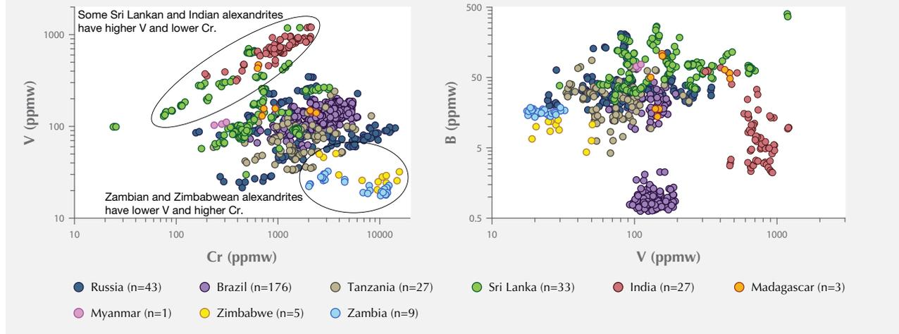
Figure 10. Cr-V and V-B plots prove very useful in validating the origin of Indian, Zambian, and Zimbabwean alexandrites. The Indian stones, along with some of the Sri Lankan specimens, have the highest V/Cr ratios. The Zambian and Zimbabwean stones have the lowest V/Cr ratios.
