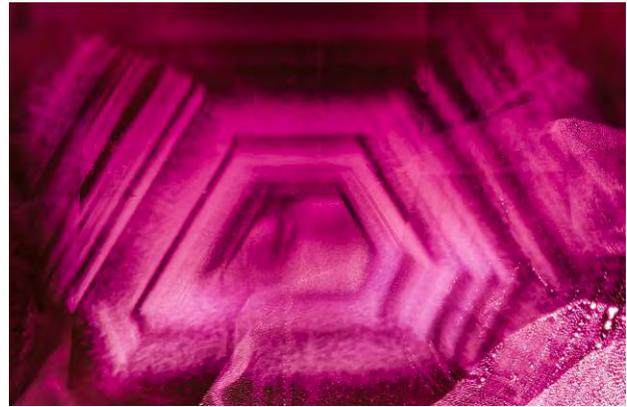
Figure 11. Heated Mong Hsu rubies are often identified by dense hexagonal white clouds in their cores. Photomicrograph by Nathan Renfro; field of view 2.97 mm.
