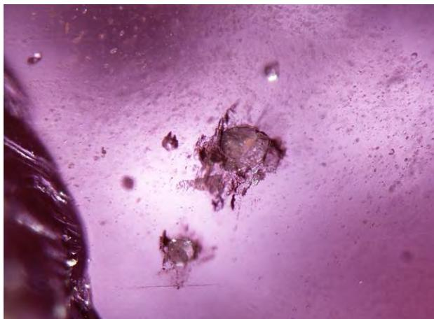
Figure 49. Amphibole inclusions are found in Mozambique as well as Madagascar rubies (shown here). In Madagascar rubies, amphibole tends to take on an elongate, rod-like morphology, although similar morphology can be encountered in Mozambique stones. Care should be taken when using these inclusions as an indicator of origin. Photomicrograph by Victoria Liliane Raynaud-Flattot; field of view 1.04 mm.
