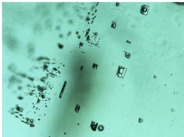
Figure 53. Irregular fluid inclusions in this Ethiopian emerald were initially interpreted as an indicator of Zambian origin. Photomicrograph by Ungkhana Atikarnsakul; field of view 1.3 mm.
