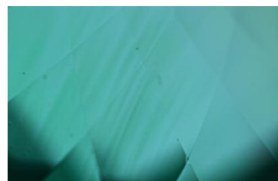
Figure 26. Subtly curved color zoning was seen in this vibrant blue-green synthetic sapphire, confirming its flame-fusion origin. Field of view 5.33 mm.
