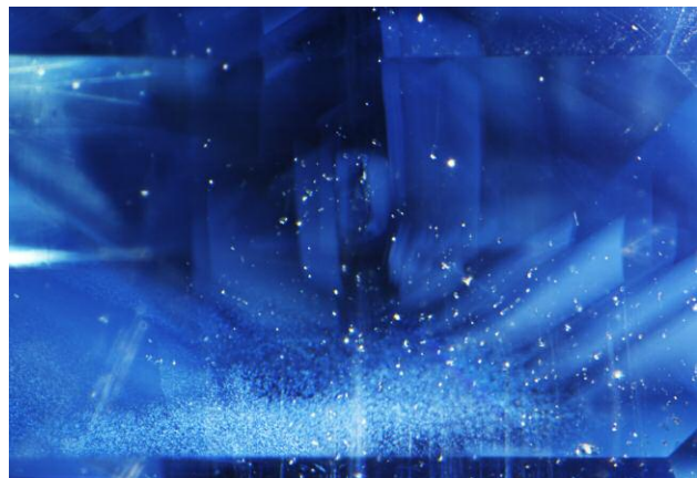
Figure 62. Zircon crystals scattered throughout angular milky clouds were more prominent in these sapphires compared to other high-Fe sapphires. Photomicrograph by Jessa Rizzo; field of view 4.7 mm.
