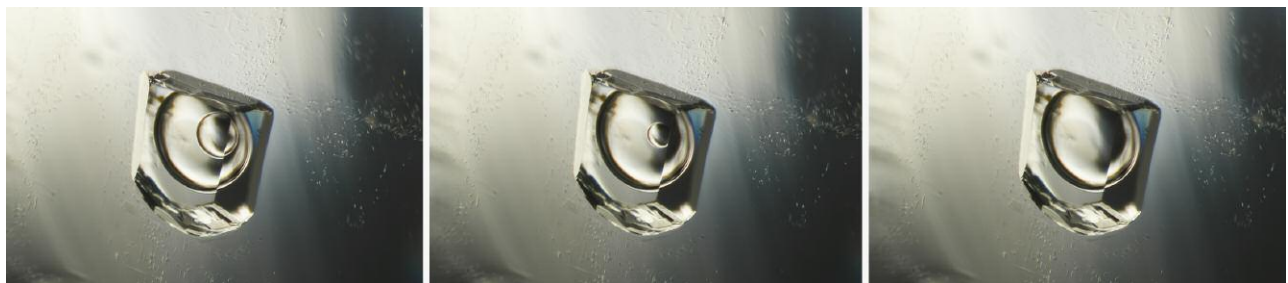
Figure 3. Photo series of a prismatic multiphase inclusion displaying a "double bubble" of gas within gas at room temperature (left). The smaller bubble shrinks by about half after approximately 45 seconds of exposure to the microscope well light (center) and completely homogenizes after about a minute (right). Photomicrographs by Hollie McBride; field of view 2.34 mm.
