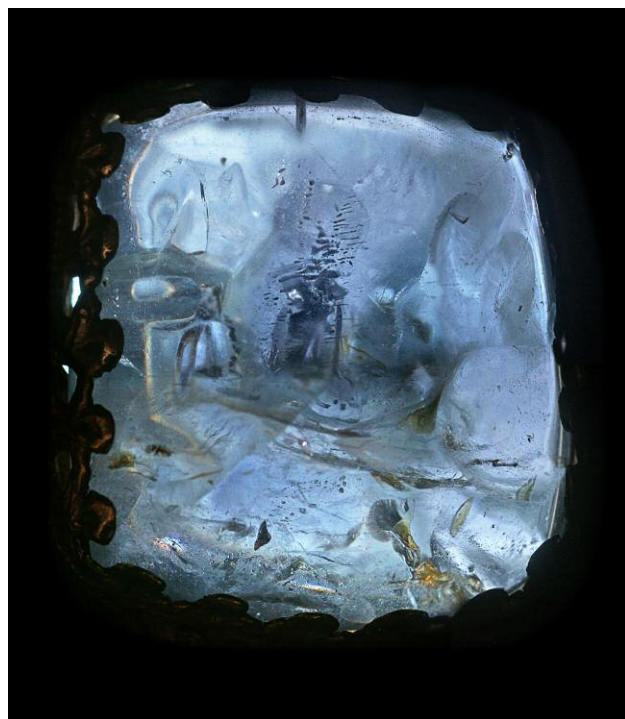
Figure 6. A composite image from four magnified photos of the large center sapphire (38 × 32 mm) on the back of the reliquary, seen through a trinocular microscope in transmitted light. Photos by G. Panczer and M.S. Krzemnicki.
