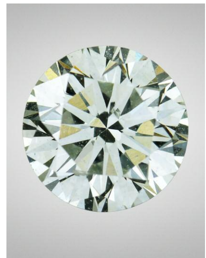
Figure 22. This 0.50 ct HPHT synthetic diamond, color equivalent to Faint Green, owed its color to nickel impurities.
