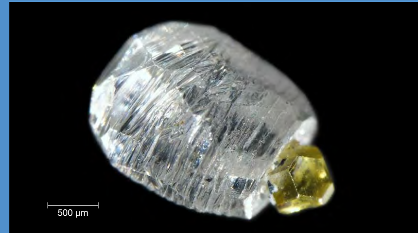
HPHT synthetic diamond crystals as small as a millimeter across are produced in China. Most are grown on {001} cube faces of tiny yellow HPHT synthetic seeds.
