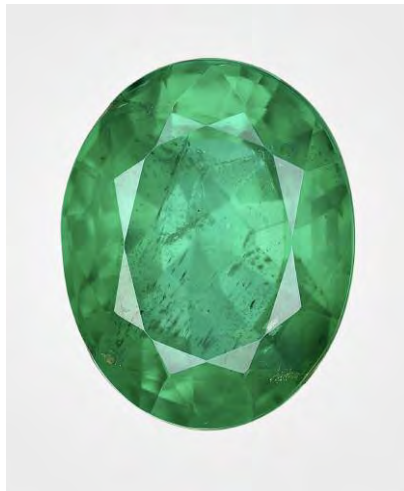
Figure 2. Face-up, the assemblage displayed natural inclusions underneath the table. Large bubbles are also visible at the corners of the beryl core, a warning sign for the observant viewer.
