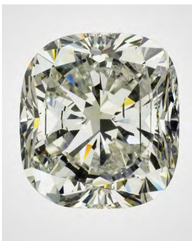
Figure 29. This 15.32 ct cushion modified brilliant, with grades equivalent to H color and I_1 clarity, is the largest HPHT synthetic diamond graded by GIA.
