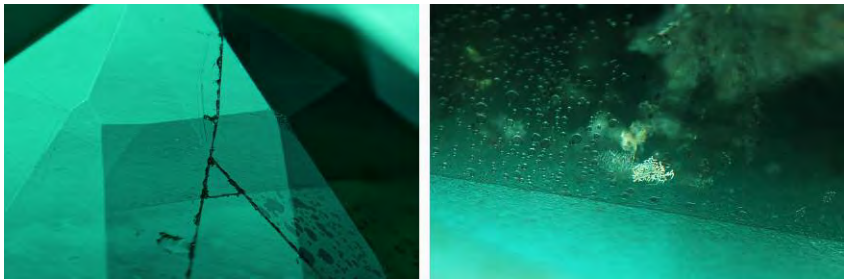
Figure 3. Left: All four glass sections of the pavilion assemblage are visible in reflected light. The small triangular segment is a protrusion from the opposite side. Field of view 3.57 mm. Right: Metallic dendritic films supporting the natural provenance of the beryl core. Also visible are planar bubbles within the cement layer. Field of view 2.90 mm.
