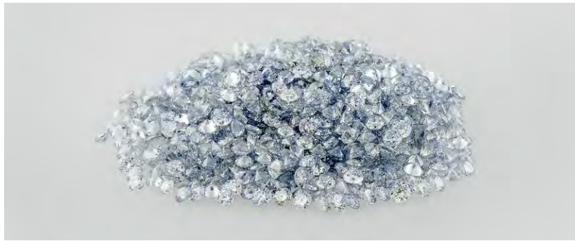
Figure 8. Out of a parcel of 1,102 diamond melee received at GIA's New York lab for testing, 1,092 were identified as HPHT synthetic melee.
