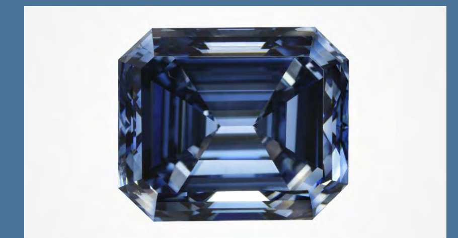
This 10.08 ct deep blue, type IIb synthetic diamond is the largest HPHT-grown blue synthetic seen at GIA. It was grown by New Diamond Technology, Inc. in Russia and is colored by boron impurities.
