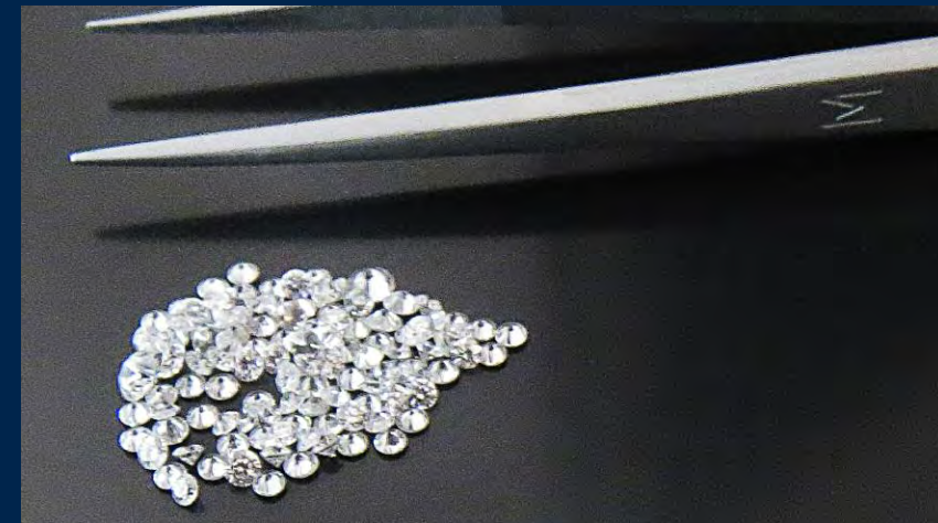
Faceted CVD synthetic diamond melee like these are often 0.01 to 0.03 ct and near colorless.
