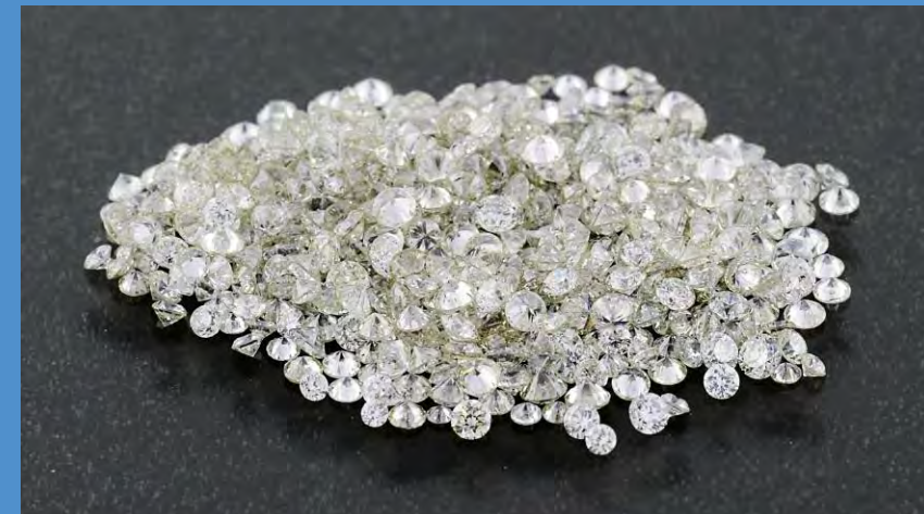
Tens of carats of near-colorless HPHT synthetics are grown in single runs and faceted into melee gems like these.
