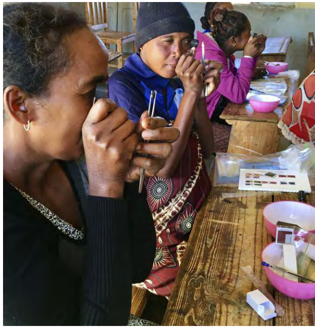
Figure 20. The women miners in Madagascar use the gem testing kit, which includes tweezers, a bowl, a loupe, a dichroscope, and a scoop. Photo courtesy of Lynda Lawson.
