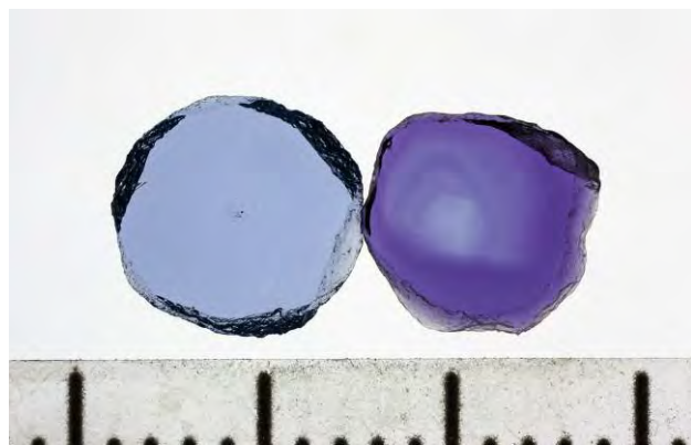
Figure 13. The blue Yogo tablet on the left shows a uniform color, while the purple Yogo tablet on the right shows diffuse angular purple color zoning. Photo by Nathan Renfro (scale is in mm).
