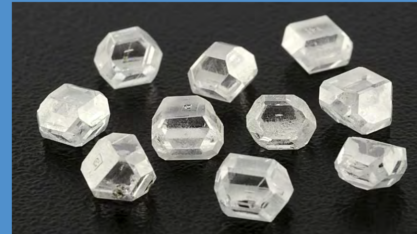
Cubo-octahedral near-colorless HPHT synthetic diamond crystals are commonly grown up to a few carats in size.
