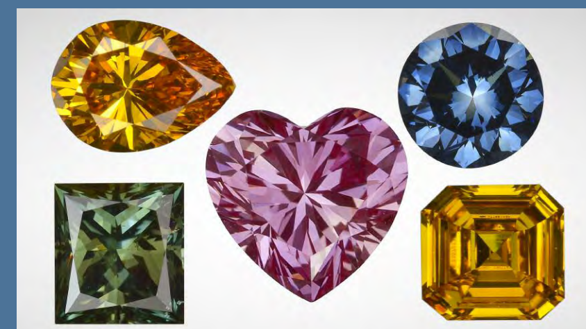
HPHT synthetics can be irradiated to green, potentially followed by annealing to turn them pink to red. They can also be grown with boron to create blue color or HPHT annealed to orange.
