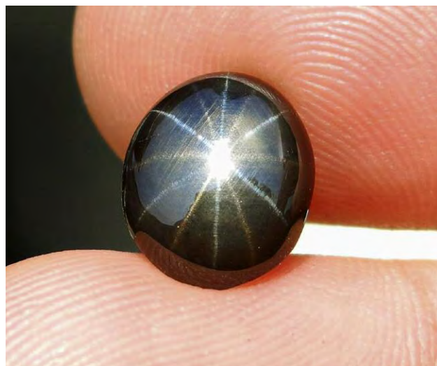
Figure 9. A 12-rayed black star sapphire, weighing 3.6 ct, with one set of golden rays and another set of silver rays producing two different-colored stars. Photo by Simon Bruce-Lockhart.
