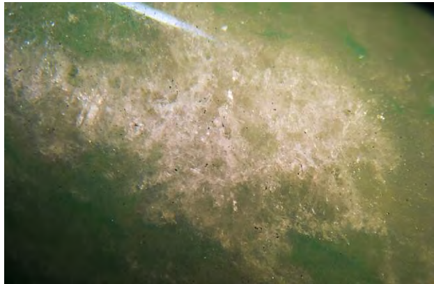
Figure 34. Microscopic observation revealed obvious acid etching marks, coarse pits, and cobweb-like surface fissures. Photo by Lai Tai-An Gem Lab; field of view 4.6 mm.
