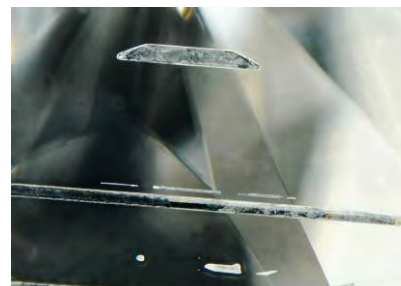
Figure 30. The metallic flux inclusions present in the synthetic diamond. Several rod-shaped structures can be seen, as well as an inclusion with a trapezoidal shape. Field of view 4.79 mm.
