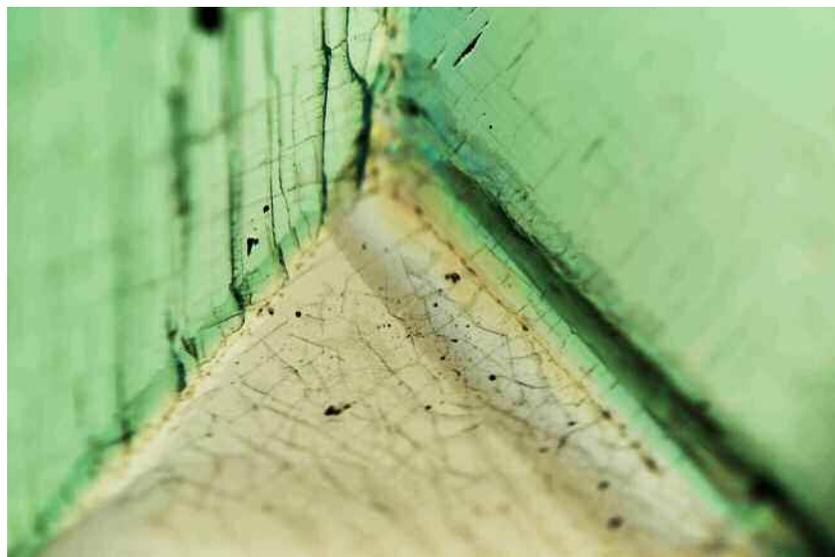
Figure 15. A thin layer of synthetic emerald deposited on a near-colorless beryl seed, a type of synthetic emerald first marketed by Johann Lechleitner in the early 1960s. Field of view 3.57 mm.
