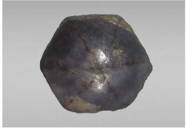
Figure 11. This 7.2 ct sapphire with a trapiche-like pattern clearly displays the host's hexagonal symmetry (11.6 × 8.0 mm). Photo by Svetlana Buravleva.
