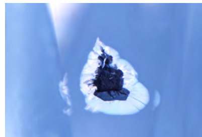
Figure 21. The large graphite crystal and its radiating tension halo, viewed from the side through the pavilion. Field of view 1.42 mm.
