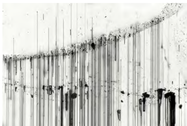
Figure 5. Two-phase inclusions and parallel tubes in a colorless beryllonite are the result of growth blockages created by tiny crystal inclusions, shown in diffused transmitted lighting. Photomicrograph by Jonathan Muyal; field of view 2.88 mm.
