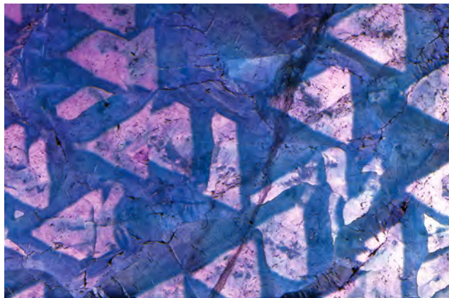
Figure 13. Left: Using diffused transmitted light, contrasting pink and blue color zoning is seen. Right: Viewing the tourmaline through crossed polarizers and looking perpendicular to the polished plate, interference colors were clearly visible. Photomicrographs by Nathan Renfro; field of view 23.95 mm.
