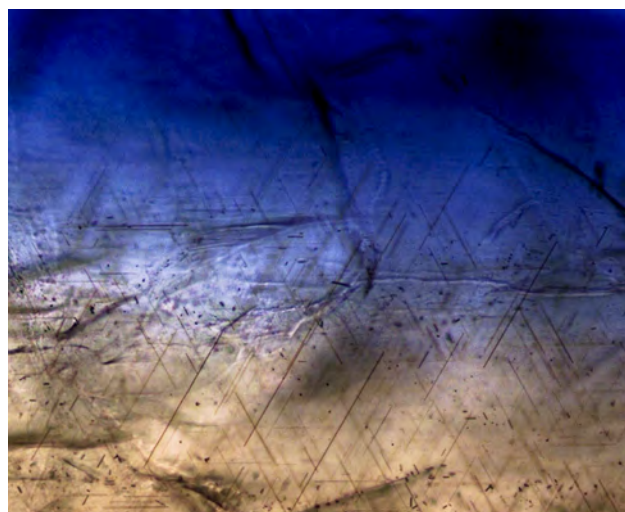
Figure 13. An example of oriented rutile needles in the Sutura sapphires. Photomicrograph by Svetlana Buravleva; field of view 0.55 mm.
