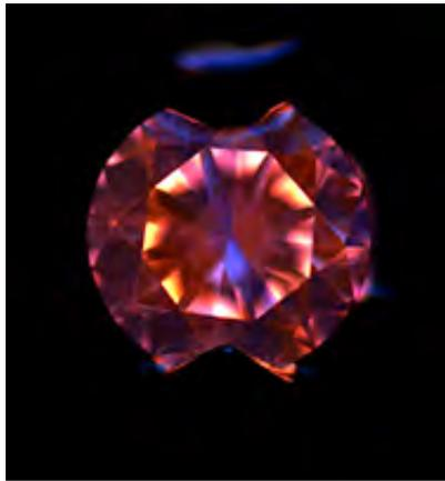
Figure 17. DiamondView imaging showed strong orange fluorescence with small irregular areas of blue fluorescence, a typical feature of as-grown CVD synthetic diamond.
