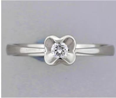
Figure 15. One of the round-cut melee mounted in this ring was identified as a CVD synthetic diamond.
