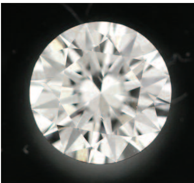
Figure 1. Emissions from the silicon-vacancy defect at 736.6 and 736.9 nm were detected in this 0.40 ct type IaB natural diamond.
