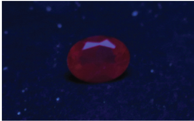
Figure 29. The synthetic spinel displayed red fluorescence under short-wave UV. Photo by Pragati Verma.
