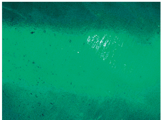
Figure 12. Slightly undulating growth zones under the table and crown were reminiscent of Russian hydrothermal synthetic emerald. Photomicrograph by Alexandre Droux; magnified 80 \times .
