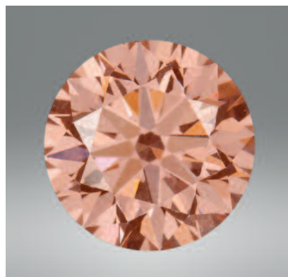
Figure 19. This 1.04 ct round was identified as a CVD synthetic diamond. Its Fancy Vivid pinkish orange color was introduced through post-growth irradiation and annealing.
