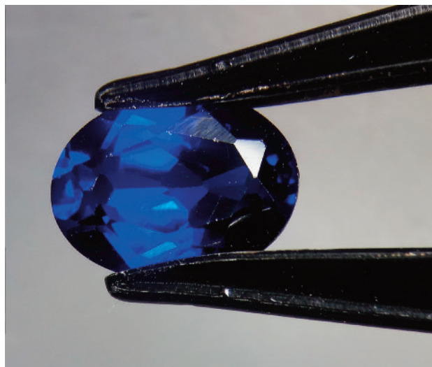
Figure 27. This 1.44 ct synthetic spinel was grown by the Verneuil process but displayed the short-wave UV reaction of a flux-grown sample. Photo by Pragati Verma.
