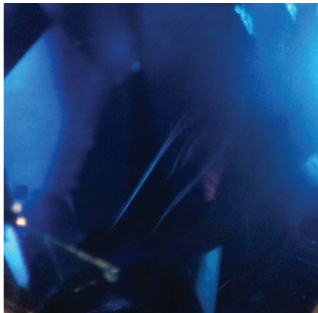
Figure 28. Series of dotted inclusions were seen in some areas of the synthetic spinel. The dots were so concentrated that it was difficult to distinguish them individually. Photomicrograph by Pragati Verma; magnified 25 \times .
