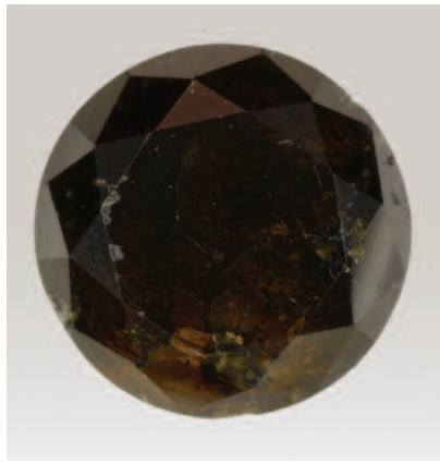
Figure 24. This 1.51 ct Fancy Black nano-polycrystalline diamond (NPD) synthetic, submitted undisclosed, was larger and showed much better transparency than a previously detected NPD synthetic.
