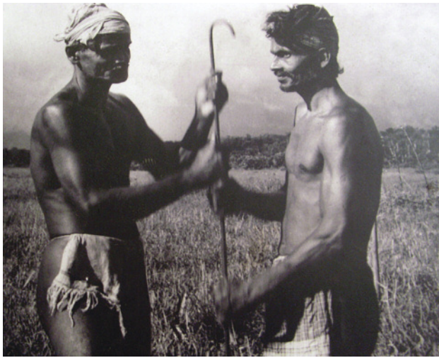
Figure 11. The traditional method of prospecting in Sri Lanka involves driving a steel rod into the ground and examining it for scratches and marks from quartz and corundum. Photo courtesy of Janka Hemachandra.
