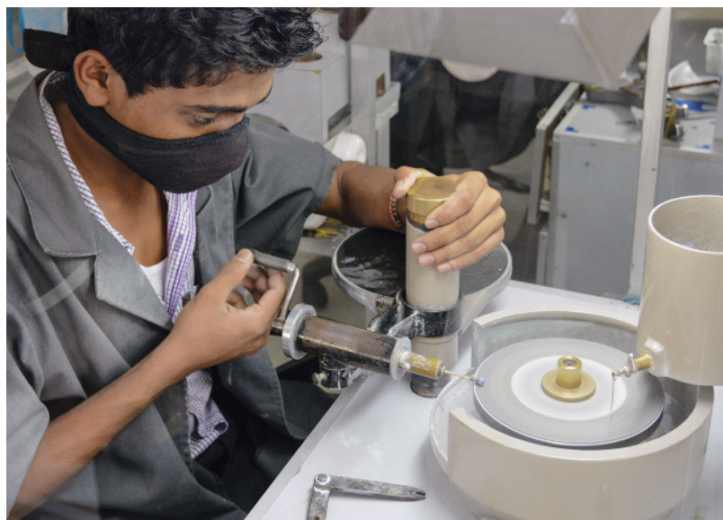
Figure 19. The girdle outline of this sapphire is being cut to precise calibrated measurements for jewelry manufacture. Photo by Andrew Lucas; courtesy of Precision Lapidaries.
