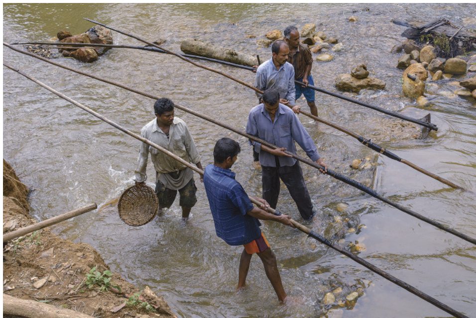
Figure 17. River mining near Balangoda involves constant dragging with mammoties to scoop out the illam for washing. Photo by Andrew Lucas.
