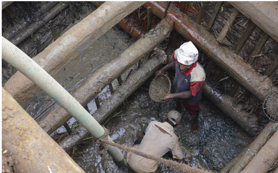
Figure 13. These miners are pumping out rain-water and removing gravel with baskets. Foliage in the wooden structure keeps the pit walls from collapsing during heavy rains. Photo by Andrew Lucas.
