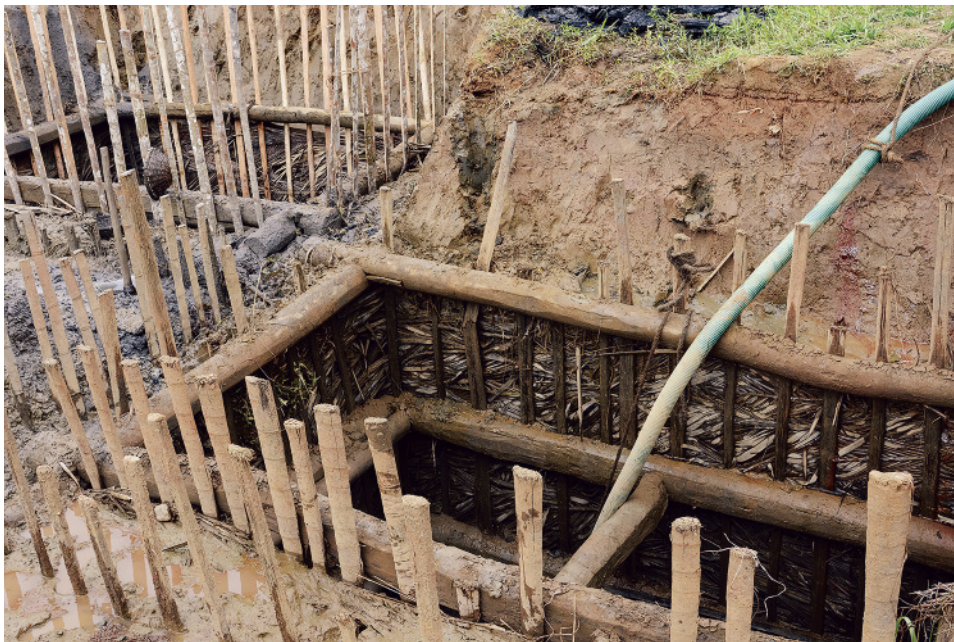
Figure 12. The classic two by four meter pits are seen throughout the mining areas of Sri Lanka. These pits are near Balangoda. Photo by Andrew Lucas.
