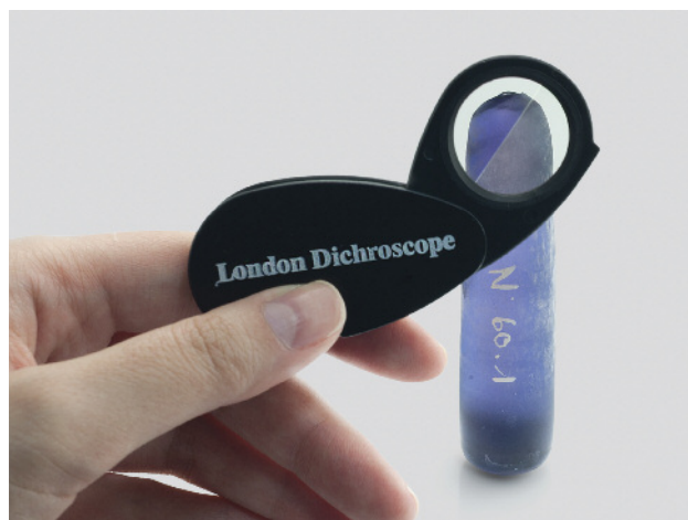
Figure 11. Pleochroism in a Verneuil-grown half-boule of synthetic sapphire, as viewed with a polaroid-plate dichroscope. In Verneuil-grown synthetic corundum, the optic axis always lies in the plane of the split. Photo by Wimon Manerotkul.
