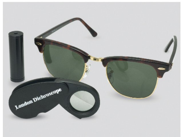
Figure 14. Three tools for observing pleochroism: the calcite dichroscope, the polaroid-plate dichroscope, and polaroid sunglasses. Polaroid sunglasses make an effective field tool, as simply rotating a pleochroic gem in front of them allows one to observe the different colors (albeit one color at a time). A polariscope with the polarizer and analyzer in parallel position can perform the same function. Photo by Wimon Manorotkul.
