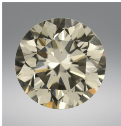
Figure 11. This 1.50 ct Fancy Dark gray CVD synthetic diamond was unusual for its combination of color grade and large size.
