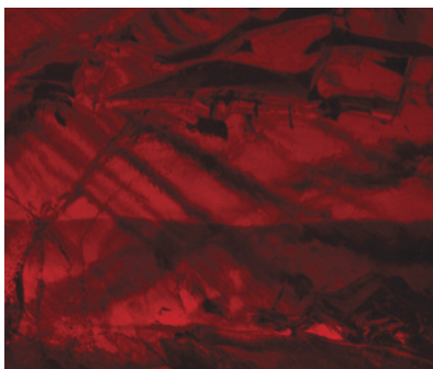
Figure 20. A dark grayish reaction zone was observed between the flame-fusion core and the flux overgrowth. Image width 15.67 mm.
