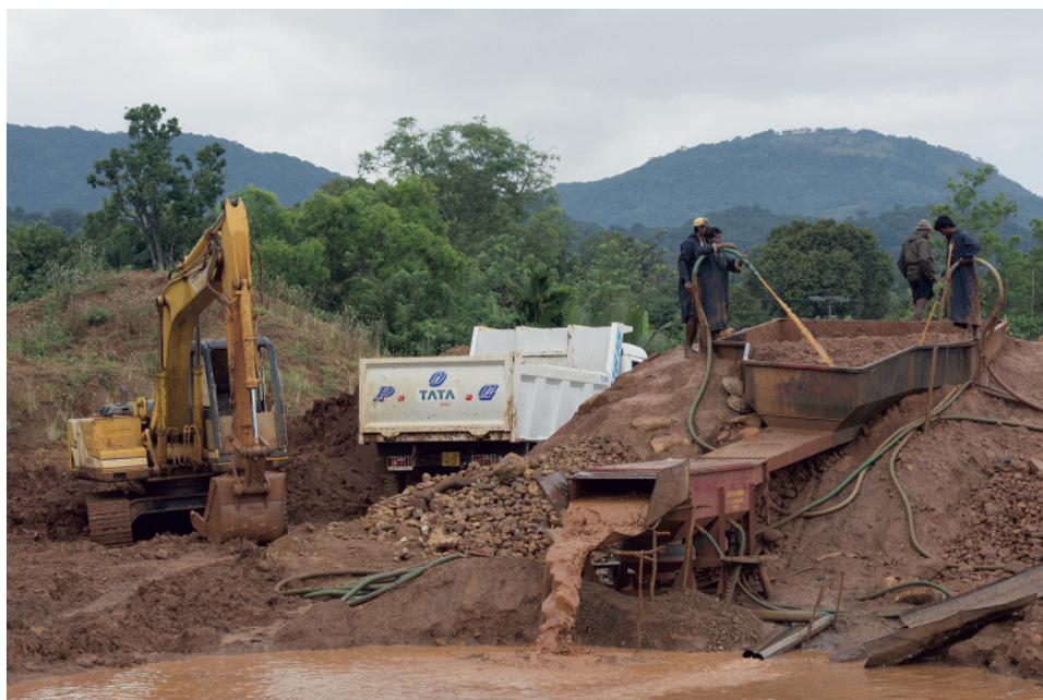
Figure 15. Mechanized mining in Sri Lanka usually includes washing the illam. Trucks move the gravel, which backhoes load into a sluice for washing. Photo by Andrew Lucas.
