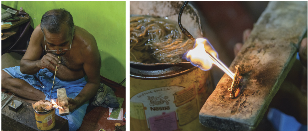
Figure 28. This jeweler preferred the traditional blowpipe for soldering 22K gold jewelry. His ability to control the direction and intensity of the flame was remarkable. Photos by Andrew Lucas.
