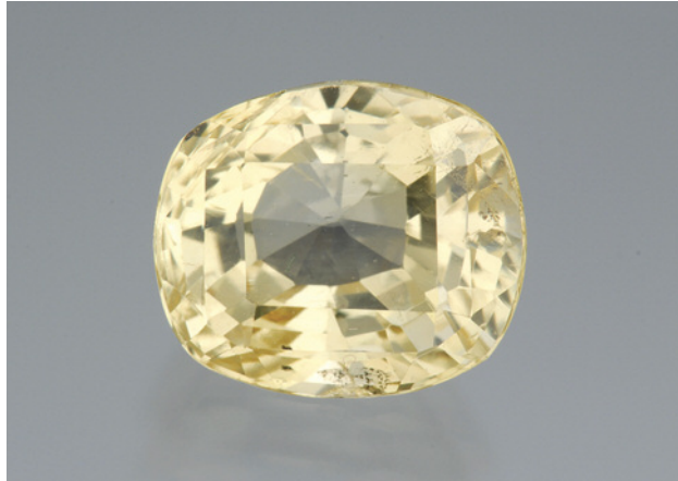
Figure 21. This 6.76 ct “mine cut” sapphire has been oriented by a Sri Lankan cutter primarily for weight retention. It can be recut to meet global standards of proportion and symmetry. Photo by Robert Weldon.
