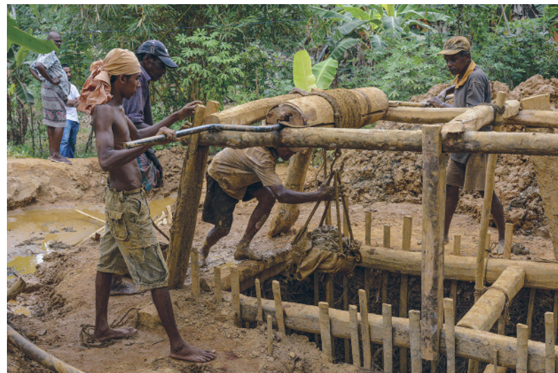
Figure 14. At this pit in Ratnapura, miners haul the overburden and gravel to the surface in buckets by a hand-powered winch. Photo by Andrew Lucas.
