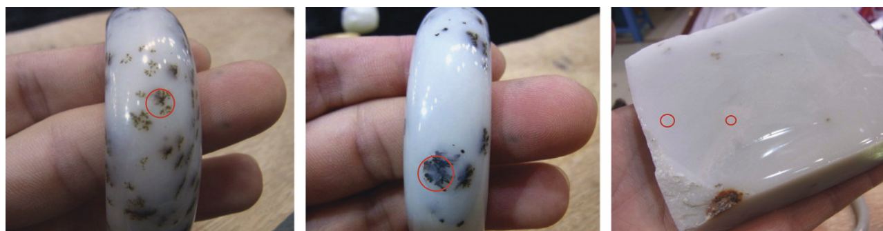
Figure 5. In these photos of the three nephrite samples, the red circles represent the testing points. The two bangles display a dendritic pattern, while the slab contains a band pattern. Photos by Yiming Chen.
