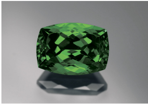
Figure 13. The color of this 7 ct tsavorite garnet is darker on the ends than in the center, but not due to pleochroism—garnet is singly refractive. Instead, this is an illustration of the Beer-Lambert law, where longer light paths result in greater absorption. Photo by Wimon Manorotkul.
