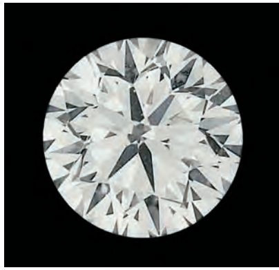
Figure 6. This 0.70 ct, D-color natural round brilliant displayed the cuboctahedral growth structure of an HPHT-grown synthetic diamond.
