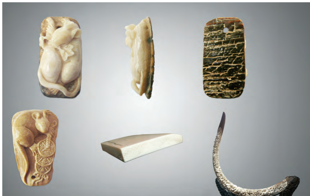
Figure 2. These three fossil ivory specimens are from mammoth tusks (bottom right). On the top row, sample M1 is composed of the weakly weathered white layer, the semi-weathered brown middle layer, and the strongly weathered black surface layer. Sample M2 (bottom left) shows the semi-weathered brown middle layer of fossil ivory. M3 (bottom middle) is only of the weakly weathered white inner layer. Photos by Zuowei Yin.
