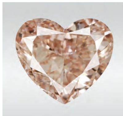
Figure 5. This 1.53 ct diamond was color graded as Fancy Intense pinkish orange. Spectroscopic analysis revealed it was type IIa and dominated by an approximately 550 nm band absorption, which usually introduces a pink-red color in natural diamonds rather than orange.
