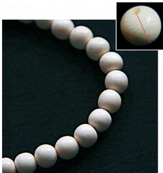
Figure 1. Modern elephant ivory samples were taken from a necklace, including the bead in the inset photo (magnified 20×). The red line indicates where the bead was cut for SEM analysis. Schreger lines can be observed on the bead. Photos by Zuowei Yin.
