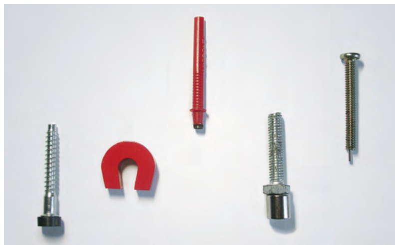
Figure 2. Five magnets of different sizes and strengths were compared in testing HPHT-grown synthetic diamonds for magnetic response. Left to right: a 1/2 in. diameter ferrite disc wand, a 1 in. wide alnico horseshoe magnet, a 1/2 in. diameter Hanneman wand, a 1/2 in. diameter N52 neodymium wand, and a 1/16 in. diameter N52 neodymium pinpoint wand. Photo by K. Feral.
