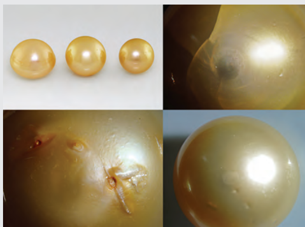
Figure A-1. These three reportedly heat-treated cultured pearls (top left) show various surface characteristics: even light yellow color with no obvious color concentration (top right), patchy yellow color with obvious orangy concentrations observed at blemishes (bottom left), and even yellow color with no obvious concentration (bottom right).
