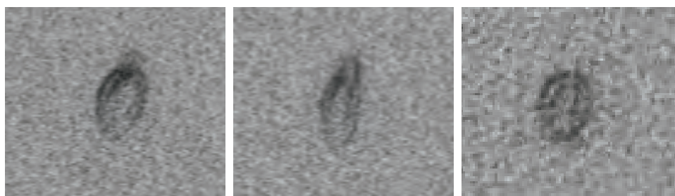
Figure 29. These micro-CT images show (left to right) X-, Y-, and Z-direction slices of pearl 1WU, zoomed center.
