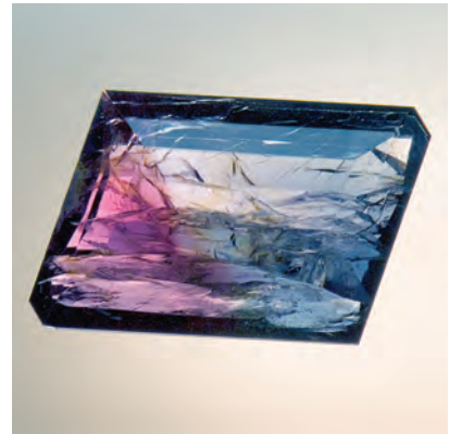
Figure 13. This 14.60 ct gem was identified as a bicolored spinel. Its blue and red zones were caused by the presence of iron and chromium, respectively.
