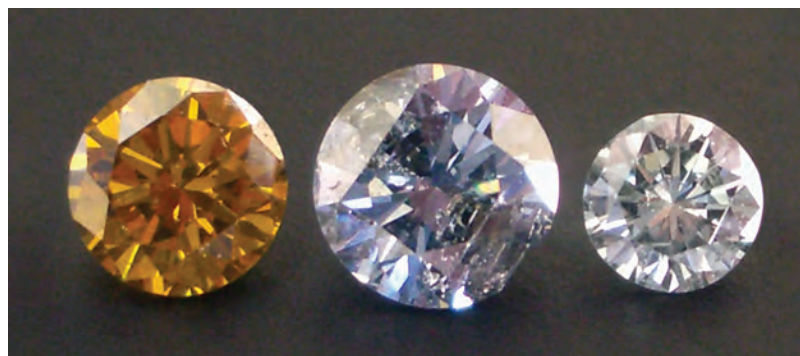
Figure 4. Magnetic attraction was observed in all three of these faceted HPHT synthetic diamonds, but only the 0.22 ct blue and 0.08 ct colorless samples were picked up by a magnet. Flotation was required to detect the weak magnetic attraction of the yellow 0.16 ct synthetic. Photo by K. Feral.
