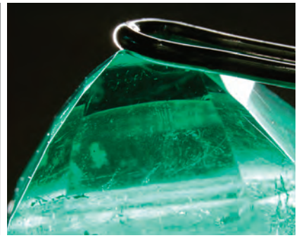
Figure 10. In this 9.96 \times 9.56 \times 7.32 mm polymer-beryl assemblage (left), an inclusion-free region with increasing thickness from the girdle to the culet was easily visible under darkfield illumination at 20\times magnification (right).
