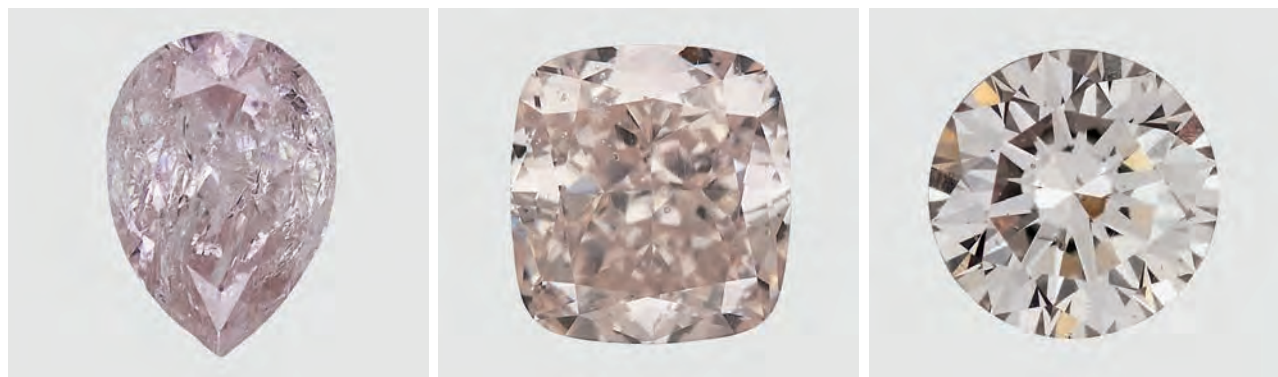
Figure 4. These three natural-color pink diamonds showed a UV-Vis absorption peak at 478 nm, a feature normally associated with yellow “cape” diamonds. From left to right, they consist of a 0.35 ct Fancy Light pink, a 1.16 ct Fancy Light pink, and a 0.80 ct Faint pink.
