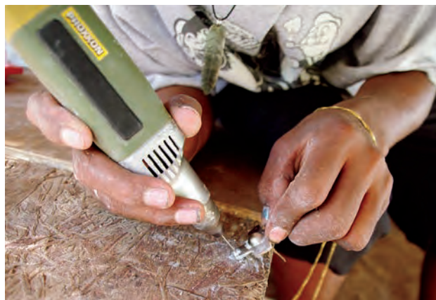
Figure 12. In a workshop on Pakin Island, local youths are taught how to drill shells containing cultured blister pearls so that they can be processed into jewelry. Photo by L. Cartier.
