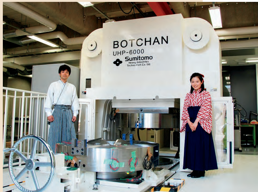
Figure 3. The GRC's large-volume, multi-anvil press uses a 6,000-tonne hydraulic ram to synthesize NPD rods up to 1 cm long. The two young GRC staff members are wearing traditional costumes from a famous Japanese novel set in Matsuyama, the city where the facility is located. Photo courtesy of T. Irifune.
