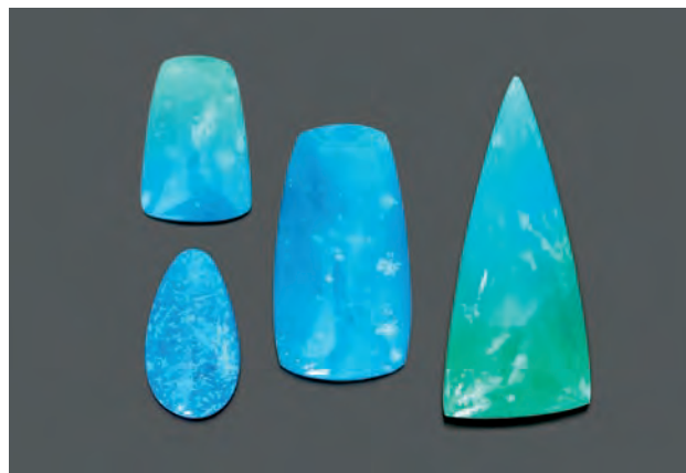
Figure 26. These partially devitrified glass samples (10.55–31.99 ct) were sold as opalized hemimorphite. The largest sample is a gift of Brad Payne; GIA Collection no. 38519. Photo by Brad Payne.
