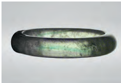
Figure 11. This 58.3 g (70.70 × 12.93 mm) polymer-impregnated jadeite bangle showed a prominent green band caused by an optical flash effect.
