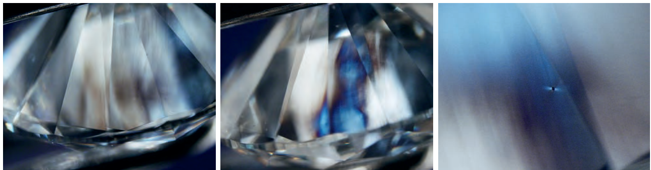
Figure 3. Relatively weak anomalous double refraction was seen when viewing these synthetic diamonds with crossed polarizers, showing low-order gray and blue interference colors with irregular, linear, or occasionally “tatami” type patterns (left and center, image widths 3.3 and 3.1 mm, respectively). Petal-shaped regions of birefringence with characteristic symmetrical patterns were sometimes observed around small black inclusions (right, image width 0.9 mm). Photomicrographs by W. Wang.
