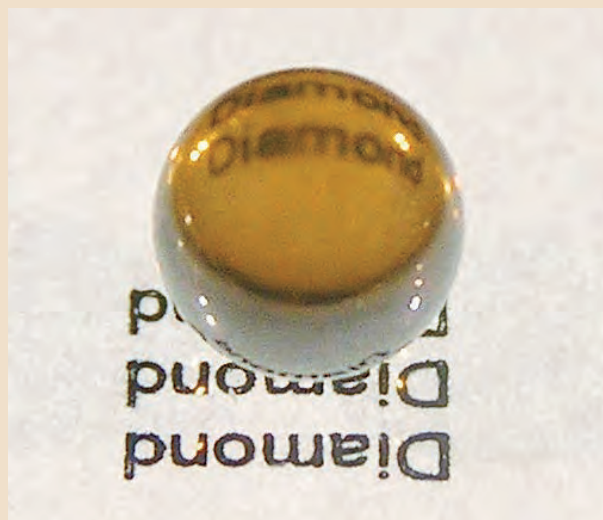
Figure 1. As this photo demonstrates, NPD is completely transparent. When placed over text on a piece of paper, the 5.09 mm sphere reverses and transmits the letters so that they are clearly legible. Photo by E. A. Skalwold.
