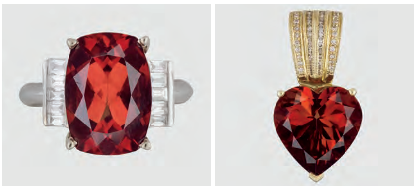
Figure 8. These two orangy red gems (left—10.90 mm wide, and right—15.30 mm wide) were identified as plagioclase (andesine-labradorite). The origin of their color—natural or induced by copper diffusion—could not be determined.
