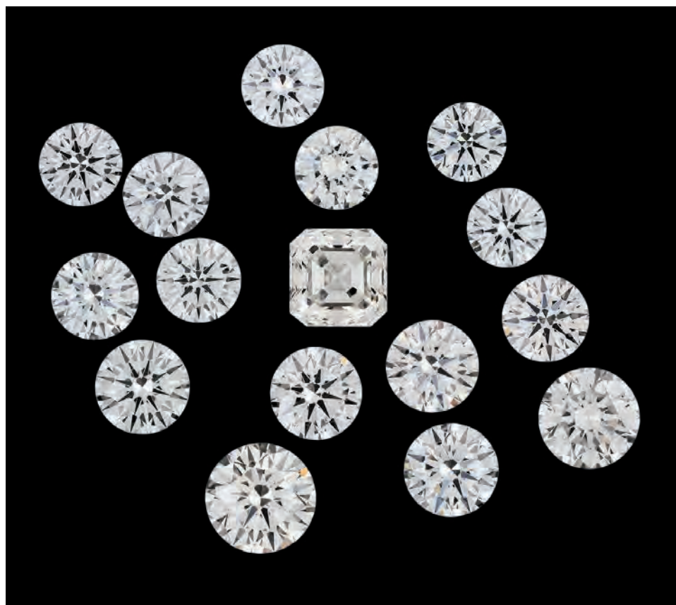
Figure 1. These faceted CVD synthetic diamond samples (0.24–0.90 ct) obtained from Gemesis Corp. were examined in this study. Color grades are mainly in the range of colorless to near-colorless, and clarity is dominantly in VVS or better categories. These features are comparable to top-quality natural counterparts. Composite photo by Jian Xin (Jae) Liao.
