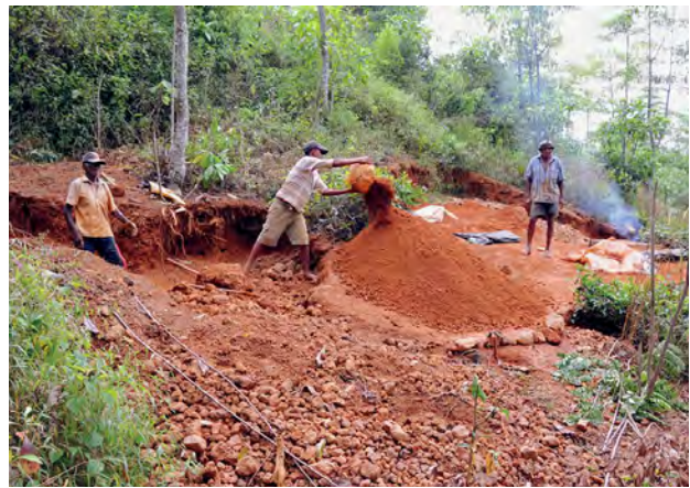
Figure 39. Artisanal hillside mining in Sri Lanka involves digging shallow pits to reach gem-bearing horizons, as shown here near Balangoda, about 35 km east of Ratnapura. Photo by V. Pardieu.
