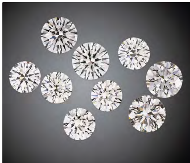
Figure 1. Colorless gem-quality CVD-grown synthetic diamonds such as these (0.22–0.31 ct) are now commercially available, making proper identification important. Photo by Robert Weldon.
