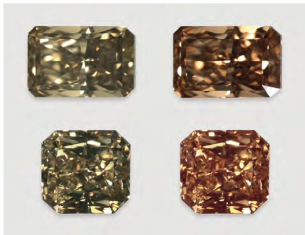
Figure 1. These 1.22 ct (top) and 3.01 ct (bottom) greenish brown type Ib diamonds, seen under daylight-equivalent illumination (left), become distinctly orangy brown under incandescent light (right). Photos by T. Hainschwang.
