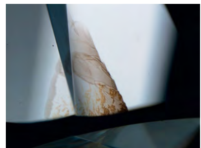
Figure 13. The brown coloration confined to the cleavage area of this diamond resulted from the interaction of radioactive fluids in the post-growth environment. Magnified 20×.
