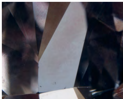
Figure 10. A pink coating on the diamond's pavilion facets was clearly visible with magnification (here, 40×).
