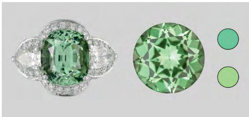
Figure 23. The 12.80-mm-long sapphire on the left was identified as natural, with its color due to a high iron content. The 2.07 ct gem on the right is a cobalt-bearing synthetic sapphire. For comparison, color coordinates (far right) were calculated for optical spectra reported in Müller and Günthard (1966) for Verneuil synthetic sapphire containing Co 3+ (ordinary ray, top; extraordinary ray, bottom).
