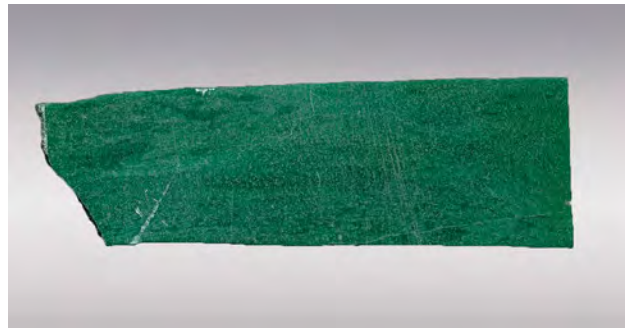
Figure 13. This polished slab (~32 mm long), resembling jadeite or nephrite, proved to be a rock composed of fuchsite, albite, and sphene. Photo by R. Navone.
