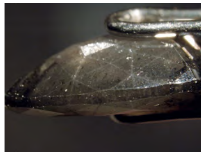
Figure 6. In reflected light, the 1.29 ct diamond displays a distinctly lighter color along the facet junctions. Magnified 30×.
