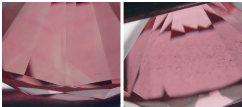
Figure 18. In diffused light, the 0.47 ct pink synthetic diamond displayed strong, uneven color zoning along growth sectors (left, magnified 45×). The 0.63 ct sample only showed subtle color zoning (right, 35×).
