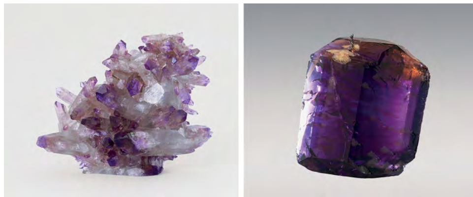
Figure 2. These \text{K}_2\text{CO}_3 -grown synthetic amethysts include an unusual Russian prismatic cluster (left; 10 cm tall) and a crystal weighing more than 1 kg (right; 15 cm tall). The vast majority of synthetic amethyst in the gem market is \text{K}_2\text{CO}_3 grown. Photos by Franck Notari.
