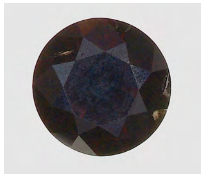
Figure 3. The black color of this 0.85 ct diamond is attributed to very strong plastic deformation.
