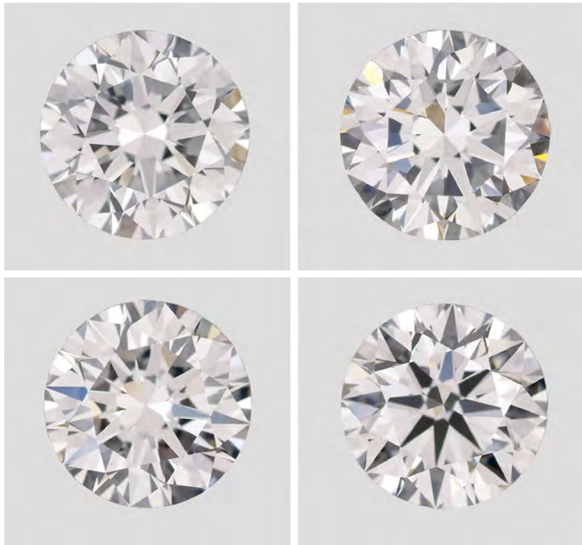
Figure 12. Shown here after HPHT treatment (E–F color, 1.74–2.57 ct), these type IIa diamonds originally had color grades of J–M. This demonstrates that HPHT annealing is being used to make subtle color improvements in such diamonds.
