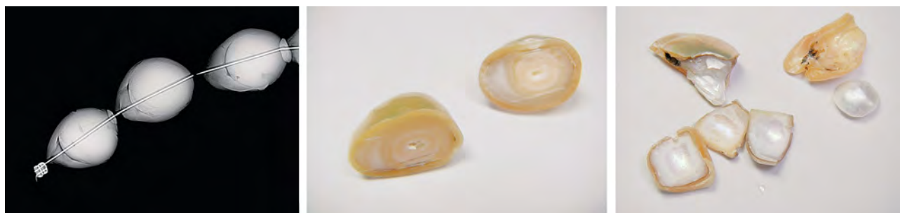
Figure 26. The X-radiograph of the cultured pearls (left) revealed off-round beads displaying concentric growth structures that were clearly visible when one sample was cut in half (center, 15.7 × 12.5 mm). When another sample was broken apart (right, originally 17 × 12 mm), a baroque freshwater cultured pearl bead was exposed. Photos by E. Strack.
