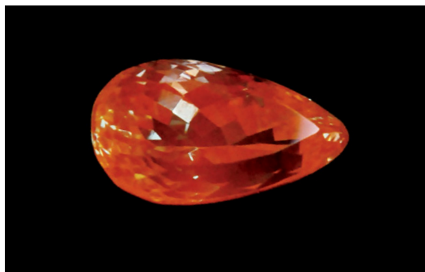
Figure 32. The heat generated by a fiber-optic lamp caused the spodumene to thermoluminesce bright orange. The original green color returned within three minutes after the stone was removed from the lamp. Photo by G. Choudhary.
