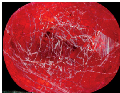
Figure 19. This ~6 ct lead glass-filled ruby appears to have been damaged by immersion in jeweler's pickling solution.
