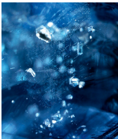
Figure 22. At 50× magnification, needles, crystals, and secondary fluid inclusions can be seen inside the included sapphire crystal.
