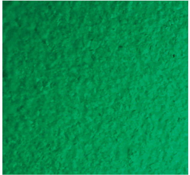
Figure 44. The glass specimen in figure 43 displays homogeneous colorless crystals throughout, giving it an aggregate structure. Photomicrograph by G. Choudhary; magnified 60 \times .
