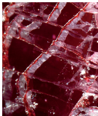
Figure 20. A red substance applied at the surface of the fractures may have been intended to disguise the damage to the ruby. Field of view ~1.1 mm.
