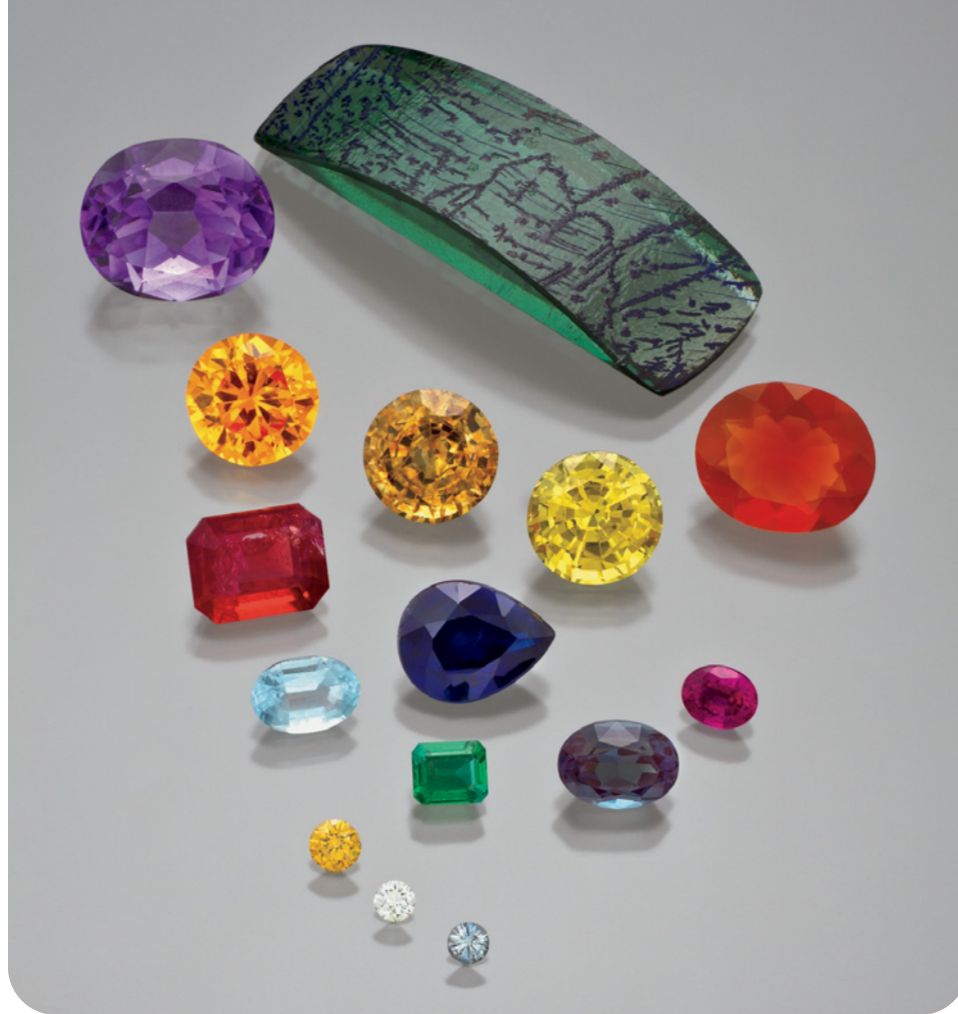
Figure 1. Consisting of synthetic alexandrite, amethyst, beryl, corundum, diamond, and fire opal, this collection represents some of the interesting and unusual synthetic gem materials encountered in the decade of the 2000s. The three smallest stones are synthetic diamonds weighing 0.06–0.14 ct. Photo by Robert Weldon.
