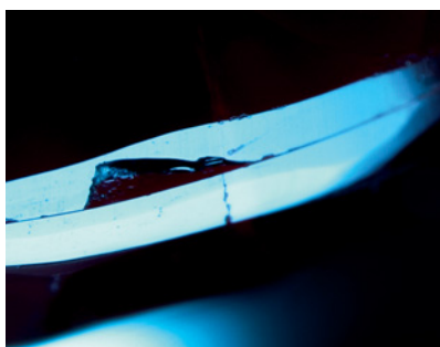
Figure 24. In reflected light, the separation plane between crown and pavilion is obvious. Magnified 40×.
