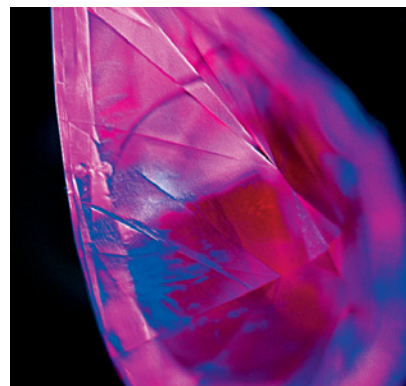
Figure 11. When exposed to the strong short-wave UV radiation of the DiamondView, the 1.05 ct CVD synthetic diamond displays strong pink fluorescence with irregular areas of blue.
