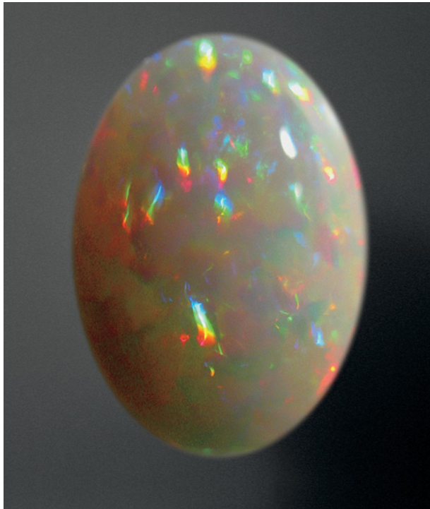
Figure 16. The diffraction of light by opal usually produces patches of pure spectral colors. On rare occasions, such as this 9.51 ct cabochon, we observed these colors diffracted from millimeter-size areas, forming small rainbows. Photo by F. Mazzero.
