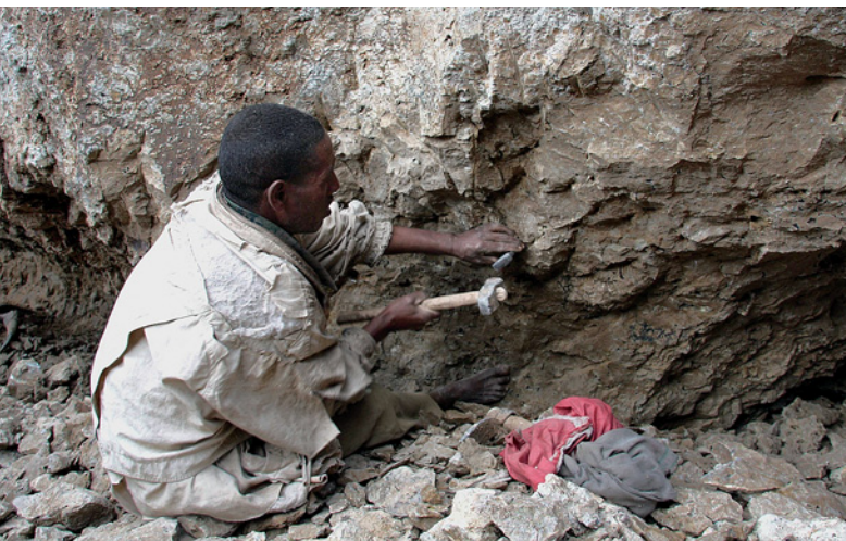
Figure 8. Miners at Wegel Tena often use rudimentary tools, such as the hammer and chisel shown here, to extract the opal from the exposed seam along the flank of the canyon. Photo by Thomas Cenki.
