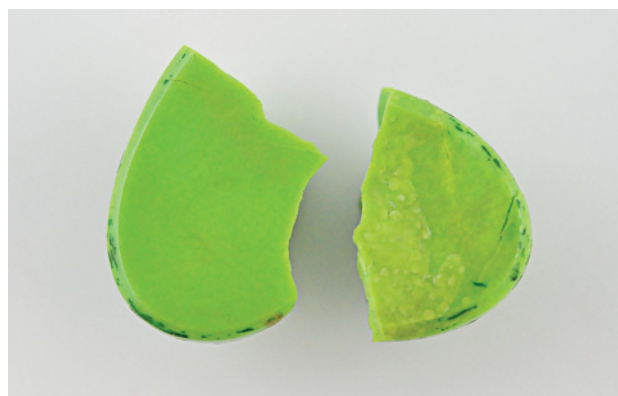
Figure 8. An 8.90 ct unveined yellow-green turquoise was broken and the portion on the right immersed in acetone for 48 hours, resulting in a duller luster and patchy loss of color. Photo by G. Choudhary.
