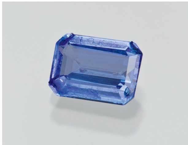
Figure 29. This 1.87 ct tanzanite was mounted in a ring with a colored adhesive. Residual adhesive is still present on some of the crown facets, particularly at the corners. Photo by Robert Weldon.
