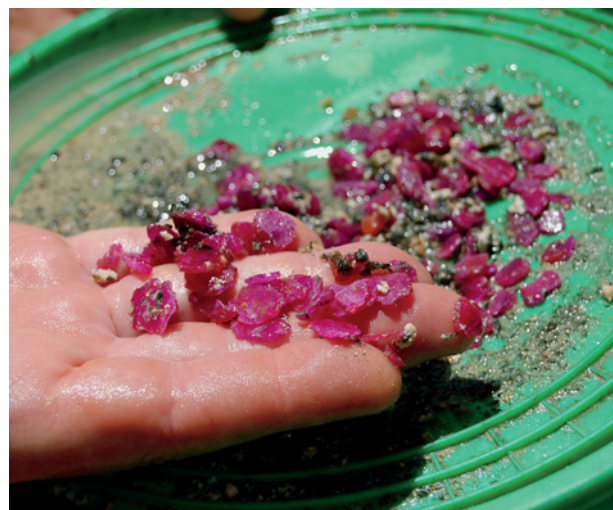
Figure 12. These ruby samples were washed from a 1 kg concentration of corundum and mica that was excavated from eluvial material at Montepuez. Photo by L. W. Snee.
