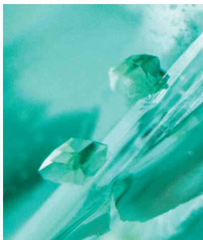
Figure 12. Synthetic diopside crystals decorate an elongated colorless rod of synthetic wollastonite in a piece of manufactured glass. Magnified 70 \times .
