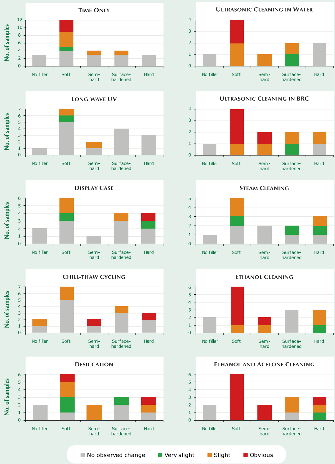
Figure 18. The observed changes in the filled emeralds varied dramatically (from none to obvious) depending on the viscosity of the filler and the type of durability test. Generally, cleaning the filled emeralds led to much more noticeable differences in their appearance than the exposure tests.
