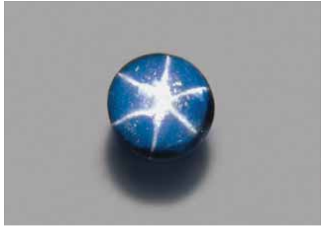
Figure 29. This 4.63 ct cabochon proved to be a synthetic star sapphire with hexagonal zoning in its core, which initially suggested natural origin. Photo by G. Choudhary.
