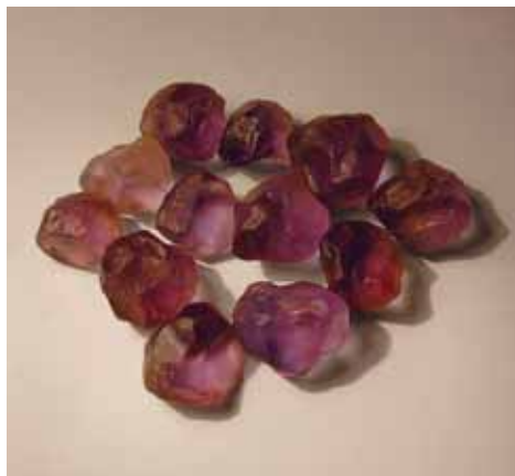
Figure 12. Some of the fluorite from Ethiopia (here, 21.0 g total weight) shows a color change from blue or grayish blue in sunlight to purple or reddish purple in incandescent light. Photos by M. Macri.
