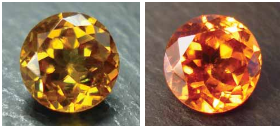
Figure 5. This unusual 2.09 ct bastnäsite shows a distinct color change, from brownish yellow in daylight/fluorescent light (left) to orange in incandescent light (right). Photos © Scott Davies.
