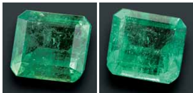
Figure 12. A 1.49 ct emerald filled with Gematrat (no. 5356; left, after filling) showed a slight change following 30 minutes of ultrasonic cleaning in BCR (right), with feathers somewhat emptied out.
