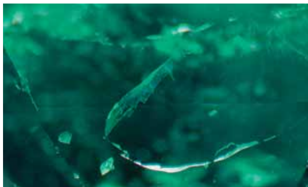
Figure 20. Delamination, or separation of the filler in fissures from the host emerald, makes this fissure in a Gematrat-filled emerald (no. 4816) more obvious after chill-thaw testing. Photomicrograph by Shane F. McClure, magnified 25×.
