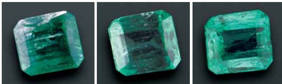
Figure 8. A 0.27 ct emerald (no. 4505; left, before filling), which was filled with a mixture of cedarwood oil and Canada balsam (center), had an obvious appearance change after five chill-thaw cycles (right): A glassy feather on the pavilion was visible through the crown.
