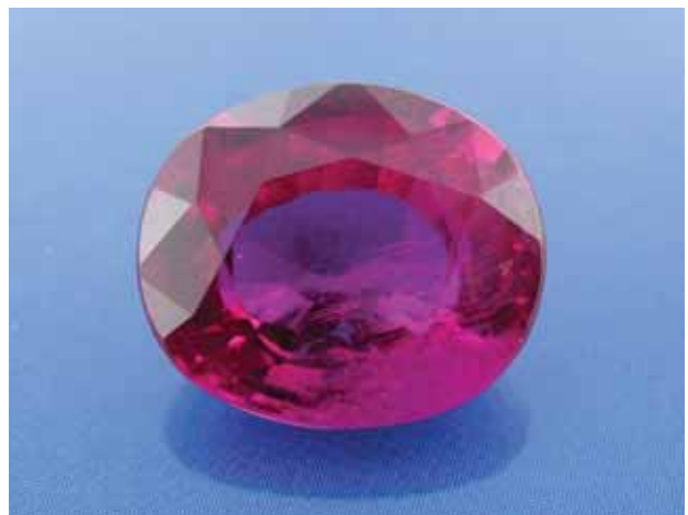
Figure 25. This 10.12 ct sample proved to be a heat-treated Kashan flux-grown synthetic ruby. Photo by S. Singbamroong, © Dubai Gemstone Laboratory.
