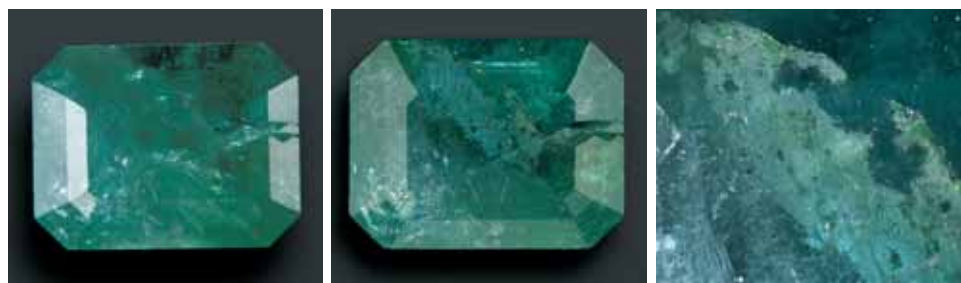
Figure 4. A 1.48 ct emerald filled with Araldite 6010 (no. 4584; left, immediately after filling) showed a very slight change with time (center): a cloudy band throughout the stone that became more evident (right; magnified 15×).
