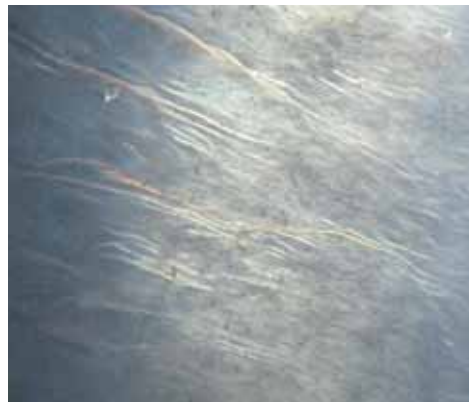
Figure 30. The central hexagonal core was visible when the synthetic star sapphire was observed with magnification and immersion (left). A wavy stress pattern was present in the area surrounding the core (left and right). Photos by G. Choudhary; magnified 30x (right).
