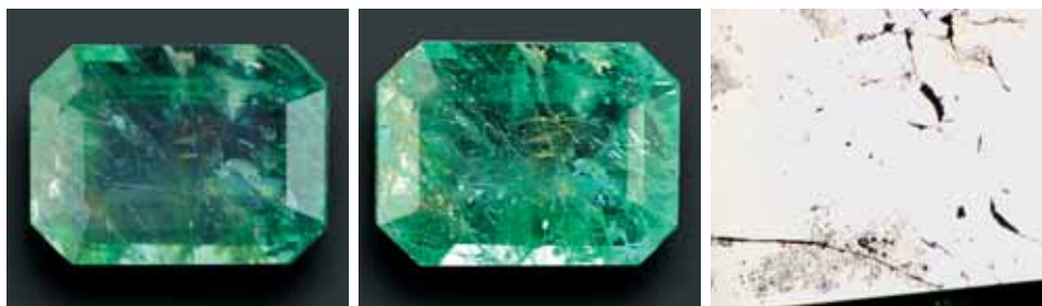
Figure 11. A 1.09 ct emerald filled with cedarwood oil (no. 4576; left) showed an obvious change after 30 minutes of soaking in water in an ultrasonic cleaner (center). Examination with 30× magnification and reflected light shows the raised material leaking from the dark fissures (right).
