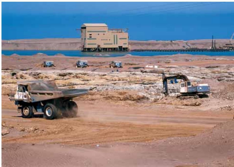
Figure 16. Namibia's beach mines, despite their relatively small production by weight, have long been an important contributor to the world market because of the very high value of the diamonds they produce. The diamonds are recovered from crevices in the bedrock after the overlying sand has been removed, as shown here in 2005. Photo by Robert Weldon.
