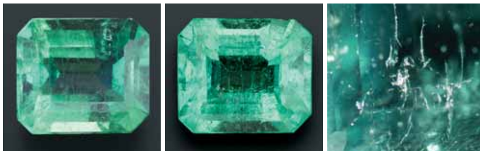
Figure 9. A 0.47 ct Gematrat-filled emerald (no. 4816; left, after filling) showed obvious changes after five chill-thaw cycles (center). The photomicrograph (magnified 40×) shows that some of the fissures have opened up and become more extensive.
