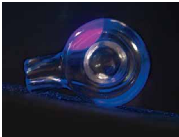
Figure 24. The zone containing the whitish bands exhibited strong pinkish purple fluorescence to short-wave UV radiation (upper left in this photo), and the edge of this zone fluoresced blue. Photo by G. Choudhary.
