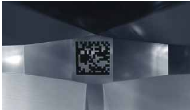
Figure 1. This simulated data matrix bar code on the girdle facet of a diamond reads “PhotoScribe.” The data matrix measures 80 \times 80 \mu\text{m} ; the same inscription using letters would require about 10 times the space. Courtesy of PhotoScribe Technologies, New York City; magnified 130\times .
