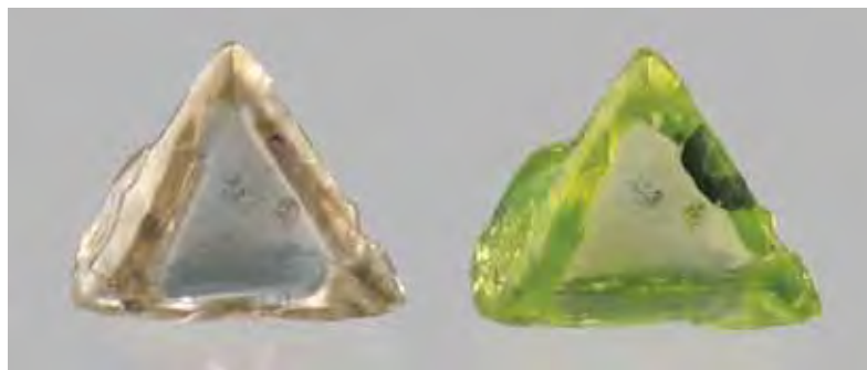
Figure 1. Some brown type Ia diamonds, such as this 1.07 ct crystal fragment (left, before treatment), can be transformed to yellow to green with HPHT processing (right, after treatment). Photo by Elizabeth Schrader.
