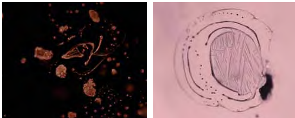
Figure 12. At 1850°C, melt aureoles, drip-like trails, and discoid fractures were common. The variation in color in these inclusions is caused by the different colors of the host sapphires. Photomicrographs by W. Wang; magnified 100× (left [sample no. 56024]) and 55× (right [no. 56025]).
