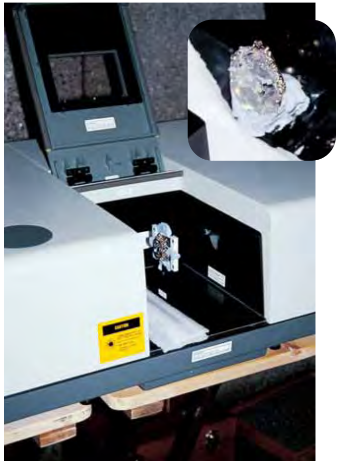
Figure 9. The Cullinan II diamond, still in its basket setting, is positioned with Blu Tack in the beam of the Nicolet 510 FTIR to measure its infrared spectrum. The inset provides a closer view of Cullinan II in the sample chamber. Photos by K. Scarratt.
