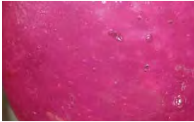
Figure 41. With magnification, numerous gas bubbles are apparent in the glassy substance filling fractures, twin planes, and cavities in this ruby bead. Photomicrograph by H. A. Hänni, © SSEF Swiss Gemmological Institute; magnified 15x.
