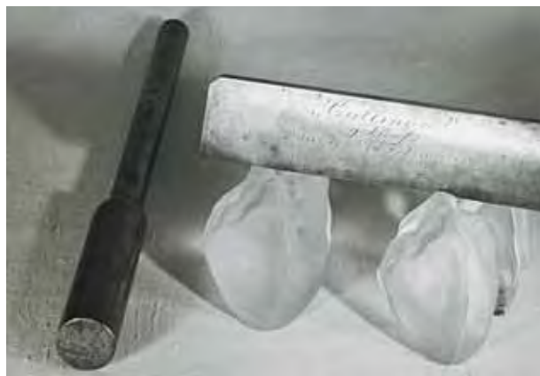
Figure 5. The hammer and knife used to cleave the Cullinan diamond. The knife is seen here spanning two models of the rough Cullinan. Photo by Alan Jobbins.
