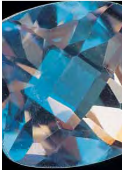
Figure 21. When the triplet in figure 20 is viewed through the crown, the separation layer along the girdle can be seen to be the cause of the blue “adularescence” in this assembled stone. Note the scratches in the color layer. Magnified 10x.
