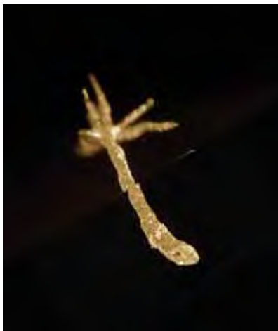
Figure 13. Resembling a palm tree, this unusual etch channel was discovered in a 2.33 ct round brilliant diamond. Magnified 80 \times .
