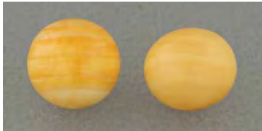
Figure 17. This sphere and ovoid (158.69 and 142.43 ct, respectively) were submitted for identification as possible Melo "pearls." They proved to be dyed shell, as evidenced by the prominent banded structure.
