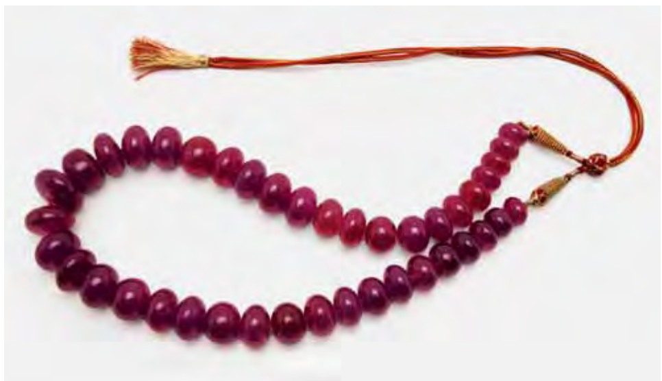
Figure 40. All of the ruby rondelles in this necklace (13–23 mm in diameter) proved to be lead-glass filled. Photo by H. A. Hänni, © SSEF Swiss Gemmological Institute.
