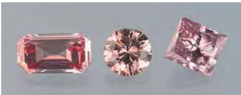
Figure 10. The intense pink color of these three diamonds (0.70–1.05 ct) proved to be the result of a surface coating.
