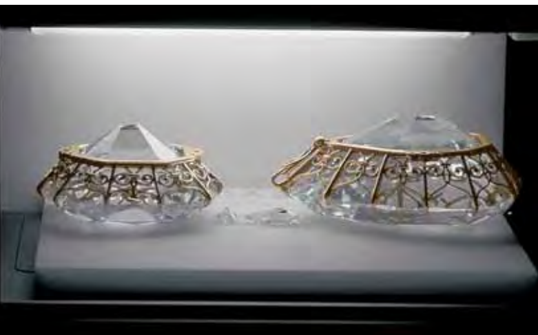
Figure 11. Cullinan I and Cullinan II, both in their basket settings, are being compared with masterstones and other diamonds of known color using a standard viewing environment. The pear-shaped diamond in the foreground had previously been color graded as “D”. Photo by Alan Jobbins
