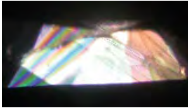
Figure 39. Plato lines are seen when the synthetic sapphire is viewed between crossed polarizers in the optic-axis direction while immersed in bromoform. This feature is strongly indicative of Verneuil synthetic sapphires. Photomicrograph by G. Choudhary; magnified 40 \times .
