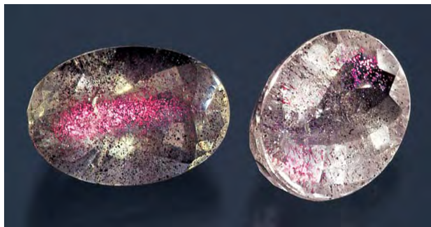
Figure 13. Covellite inclusions are responsible for the “hot pink” schiller in these two samples of smoky and near-colorless quartz (18.81 and 18.00 ct).
