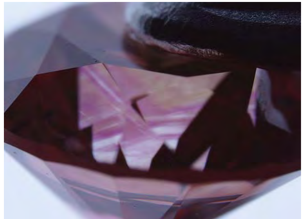
Figure 12. A few diamonds contained distinct pink-to-red zones in some areas, with brown and near-colorless zones in others. Photomicrograph by C. P. Smith; magnified 28×.
