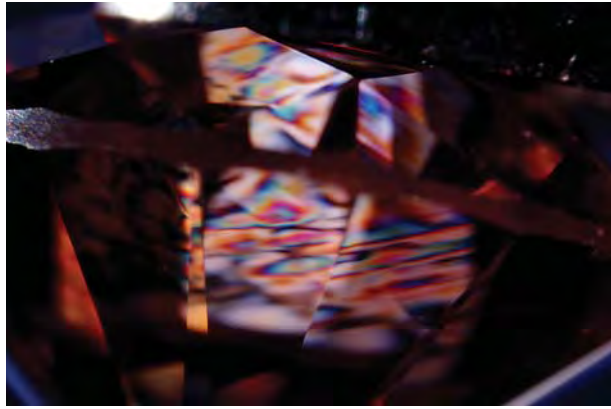
Figure 9. A few of the samples exhibited a higher degree of strain, in a mottled or “cellular” pattern, similar to that seen in natural-color natural diamonds in this color range (but not encountered in synthetic diamonds). Photomicrograph by C. P. Smith; magnified 32×.
