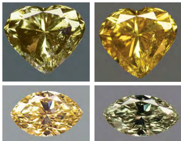
Figure 2. These images show typical color changes seen in chameleon diamonds of the Classic (top, 0.83 ct) and Reverse (bottom, 1.09 ct) types. The left images show the stable color, while the unstable color is on the right. Photos by T. Hainschwang.
