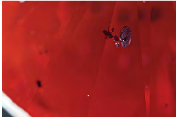
Figure 5. Graphitization was also evident along internal stress fractures. Typically, these stress fractures displayed a narrow, highly reflective fringe along the outermost extension of the fracture that was probably induced by the expansion pressure created when the walls of the stress fractures converted to graphite. Photomicrograph by C. P. Smith; magnified 58×.
