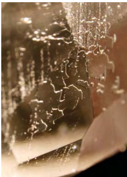
Figure 18. In addition to areas of channels and grooves, the middle stone in figure 16 also showed thin, uneven crystalline layers on its surface. These layers are transparent (left) but slightly rough, and therefore scatter light and have a white appearance when viewed at certain angles (right). Magnified 20 \times (left), 15 \times (right).
