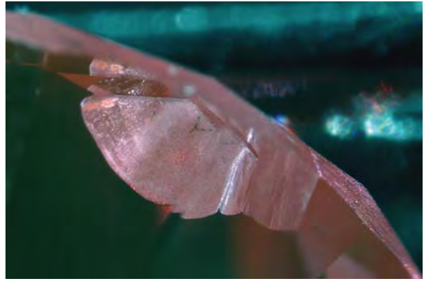
Figure 6. Cleavages that reached the surface exhibited distinct etching along their full extent. Such etching is also evidence of HPHT treatment. Photomicrograph by C. P. Smith; magnified 52×.
