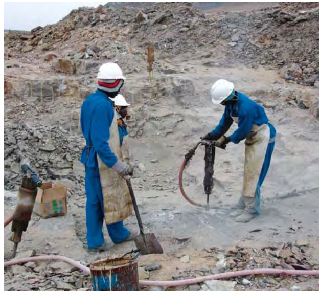
Figure 4. Mining for amethyst geodes at the Sarusas mine in northwestern Namibia employs pneumatic drills to make holes in hard areas of the basalt, which are then filled with an expansion compound to help fracture the rock. Courtesy of Kristall Galerie.
