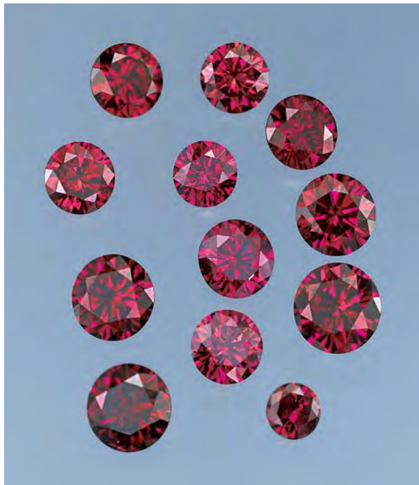
Figure 2. This group of 12 stones (0.14–0.65 ct) represents the range of colors Lucent Diamonds is marketing as “Imperial Red Diamonds.” These treated-color natural-origin diamonds have been produced by a new treatment method, which involves HPHT annealing, irradiation, and low-pressure annealing at relatively lower temperatures. Photo © Harold & Erica Van Pelt.
