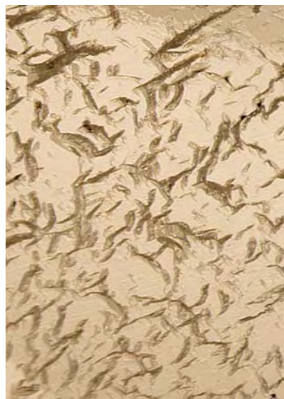
Figure 17. The unusual surface texture—numerous small, very shallow, irregular grooves and channels—almost completely covered the stone on the far left in figure 16. Magnified 112 \times .
