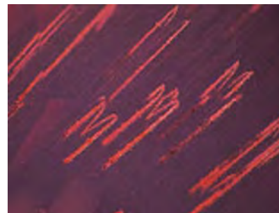
Figure 16. Laboratory staff members had never before observed the unusual "M"-shaped etch tubes seen in the spinel in figure 15. Magnified 10×.
