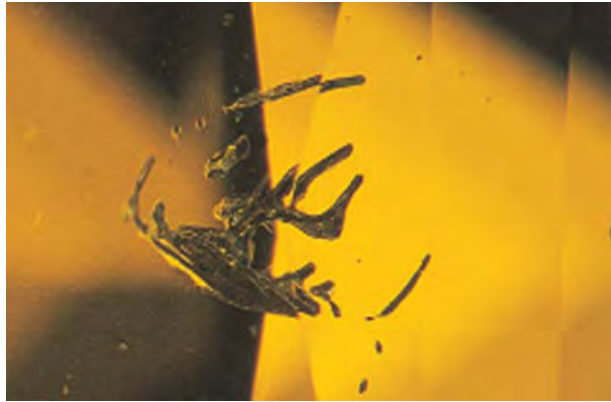
Figure 7. Metallic inclusions are another key identifying feature of laboratory-grown diamonds. They appear black and opaque in transmitted light, and gray and metallic in reflected light. They can display a wide variety of shapes, as shown in this 0.62 ct sample. Photomicrograph by J. E. Shigley; magnified 40 \times .
