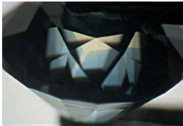
Figure 29. All of the type IIb and mixed type IIb + Ib samples we examined for this study displayed color zoning following the cubo-octahedral habit of the crystals, which is very characteristic of synthetic diamonds. This sample shows blue and yellow color zoning following a distinctly unnatural pattern. While most of the samples in this study showed some kind of unnatural zoning, the patterns in these types were by far the most pronounced. Photomicrograph by Shane F. McClure; magnified 28x.
