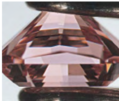
Figure 26. Shown here are two examples of color zoning seen in the pink synthetic diamonds (0.41 and 0.33 ct). The zoning appears as orangy pink and purplish pink areas separated by sharp boundaries (known as planar graining) that are often perpendicular to the table (left), but may occur at an angle to this facet (right). This color zoning is best seen by observing close to the girdle plane of the sample. Photomicrographs by J. E. Shigley.
