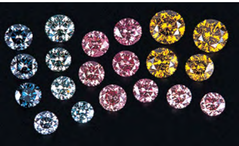
Figure 2. These blue, green, pink, and yellow laboratory-grown faceted diamonds (0.13–1.34 ct) are representative of the faceted material examined for this study. Photo by Maha Tannous.
