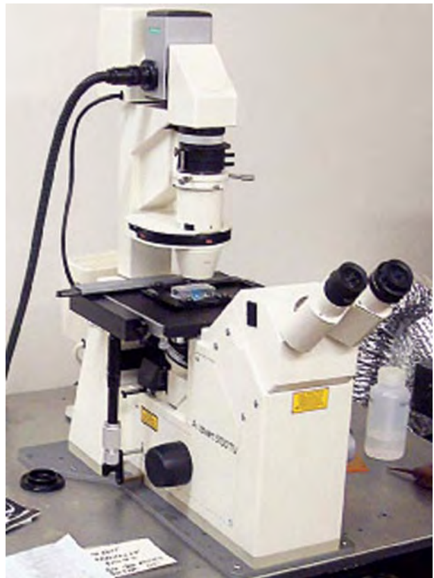
Figure 14. This confocal microscope system is being used to fingerprint a diamond by recording the relative positions of its inclusions. The blue light in the center is a sample diamond being illuminated by the microscope's laser. Courtesy of University of British Columbia Bioimaging Facility.
