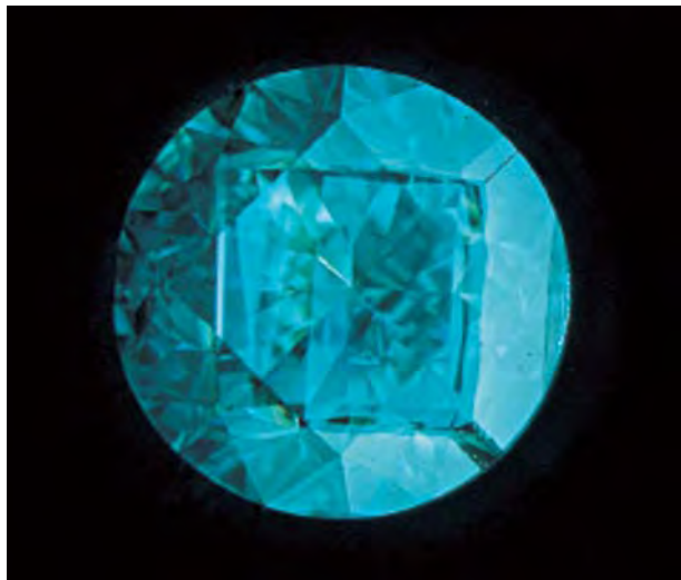
Figure 22. The cathodoluminescence of this 0.31 ct grayish green sample displays the distinctive arrangement of internal growth sectors identifying it as a lab-grown diamond. Photo by S. Muhlmeister and C. M. Breeding.
