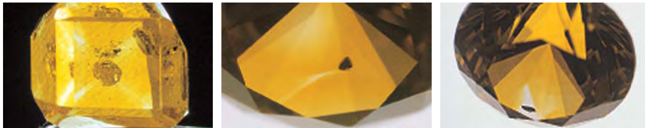
Figure 4. All the synthetic diamonds showed color zoning related to growth sectors. The yellow crystal (0.63 ct) on the far left exhibits a cross-shaped pattern of four narrow colorless zones that point toward the cube faces at the corners of the crystal; the gray area near the middle represents the seed location on which the original crystal grew. The 0.47 ct orangy yellow sample in the center has a prominent metallic inclusion, as well as color zoning due to the uneven distribution of nitrogen between growth sectors. Yellow sectors contain nitrogen, while colorless sectors contain little if any of this impurity element. The 0.57 ct sample on the far right displays similar yellow and colorless growth sectors, which are diagnostic of many laboratory-grown diamonds. Photomicrographs by J. E. Shigley; magnified 15 \times , 20 \times , and 20 \times .
