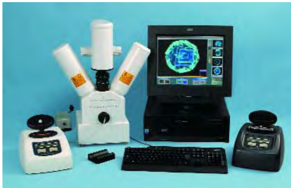
Figure 6. The Diamond Trading Company's Diamond Verification Instruments are effective for identifying both HPHT-grown and CVD synthetics. From left to right, this picture shows the DiamondSure, DiamondView, and DiamondPlus instruments. Photo by C. Alderman.
