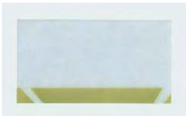
Figure 14. Color zoning is obvious in this polished cross-sectional slice through a CVD synthetic diamond layer on its HPHT-grown synthetic substrate (left). Although predominantly yellowish green, the type Ib HPHT-grown substrate has two sectors with less color. The sample is 6 mm long, and CVD growth beyond the edges of the substrate has been removed. In a DiamondView image of the same slice (right), the CVD layer shows the orange to orangy red luminescence typically seen for N-doped samples, as well as the characteristic striations (the circular pattern is from the vacuum holder). These striations are a result of different uptake of defects on the risers and terraces of steps on the growth surface. Photos by A. Taylor.
