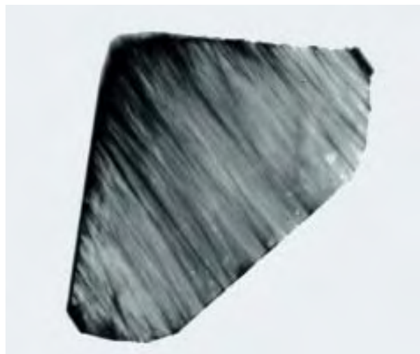
Figure 9. The columnar texture is also evident in this X-ray section topograph of a faceted CVD synthetic (girdle diameter 5.5 mm), in which a cross-sectional slice parallel to the growth direction was sampled by the X-ray beam.
