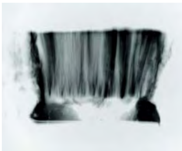
Figure 8. In this X-ray section topograph of a 2-mm-thick layer of CVD synthetic diamond on a type Ib HPHT-grown synthetic substrate, a cross-sectional slice parallel to the growth direction has been sampled. The columnar texture is caused by dislocations and is typical of CVD synthetic diamond, but it is not always seen in such an extreme form. The interface between the substrate and the CVD layer is clearly evident from the abrupt change in contrast. Features such as these in X-ray topographs may be used as evidence to support identification.
