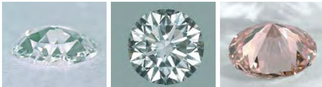
Figure 4. High-purity CVD material is colorless, as illustrated by the 0.44 ct ( D-SI_1 ) rose cut and 0.82 ct ( E-VVS_1 ) round brilliant shown here (left and center), but it is technically more difficult to grow than brown material, such as the 0.85 ct pinkish brown ( VVS_1 ) round brilliant on the right. For relatively thin layers of CVD synthetic diamond, flat cuts give the highest yield, but the ability to grow thicker layers makes brilliant cuts more feasible. Photos by M. Crowder and P. Martineau.
