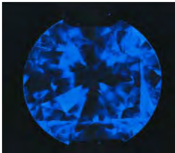
Figure 21. DiamondView images of this 0.30 ct high-purity CVD synthetic round brilliant did not show orange luminescence. The blue luminescence emanates from bundles of dislocations in arrangements not seen in natural diamond. High-purity CVD synthetics of this kind are not initially expected to be produced commercially. Photo by P. Martineau.
