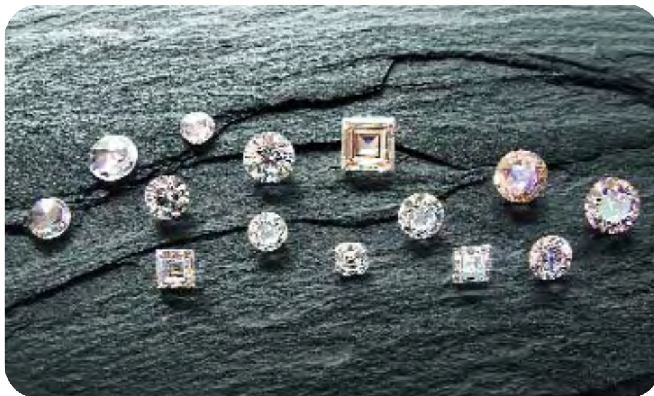
Figure 1. These faceted CVD synthetics (0.21–1.04 ct) range from colorless to brown. Diamond Trading Company faceted CVD synthetics are not commercially available; they have been produced solely for research and education. Photo by M. Crowder.
