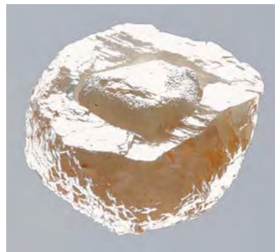
Figure 7. After the dark brown material at the interfaces was removed by boiling the diamond in acid, it became clear that the inner core was an octahedral diamond crystal, most of which was spatially separated from the overgrowth layer. Analyses showed that the inner core and the outside overgrowth have very different physical and chemical properties.
