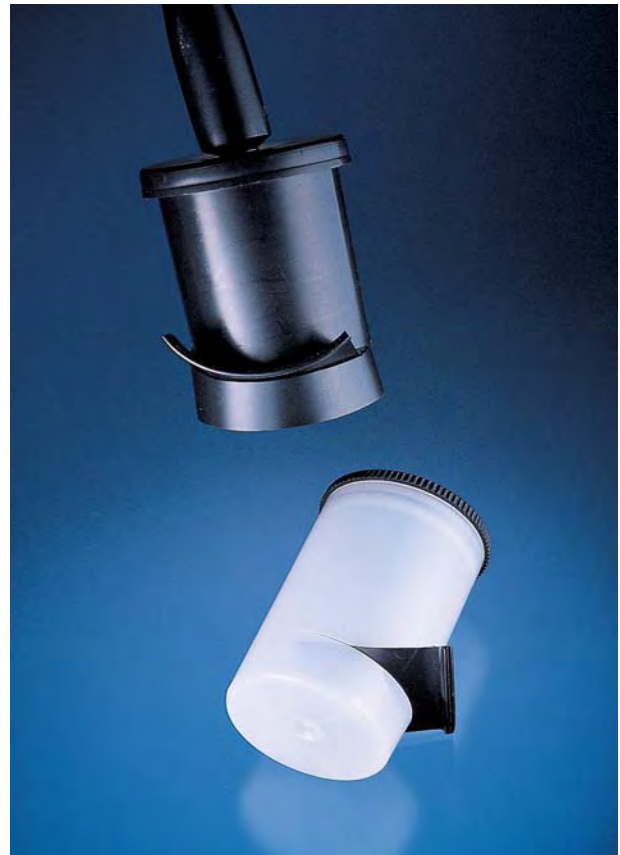
Figure 30. Simple light shields for blocking hot spots produced by fiber-optic illuminators can be manufactured from plastic film canisters. The translucent white light shield provides diffused fiber-optic illumination, while the one constructed from an opaque black film canister provides intense direct fiber-optic lighting. Photo by Maha Tannous.
