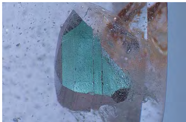
Figure 19. Diffused transmitted light is an excellent way to observe color in transparent-to-translucent mineral inclusions. The green color of this fluorite inclusion in topaz is clearly seen with this technique. Magnified 7 \times .
