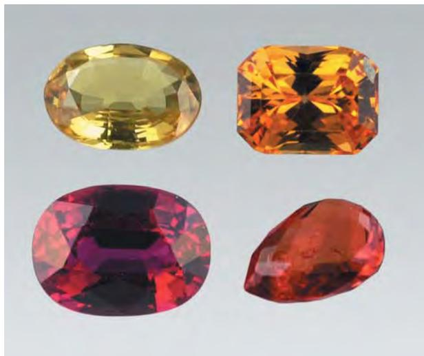
Figure 32. These sapphires were treated by Be diffusion. Shown are a yellow (sample 45035, 1.22 ct) and an orangy red sapphire (sample 45033, 1.54 ct pear shape) that were treated in Thailand, as well as an orange sapphire (sample 48717, 0.86 ct) and ruby (sample 48878, 2.78 ct) that were treated by an unknown source. See table 2 for the chemical analyses of these samples. Photo by Elizabeth Schrader.
