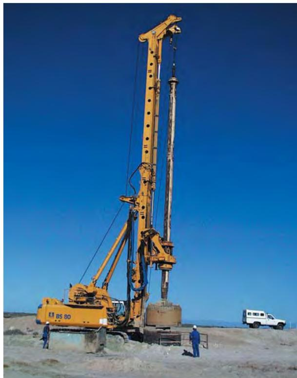
Figure 35. Shown at an on-shore marine diamond deposit in Namibia, this 100-ton rotary drilling rig employs a 2.5-m-diameter bucket, which has a capacity of 5 m<sup>3</sup> or 10 tons and can reach depths to 115 m. Courtesy of Bauer Maschinen.
