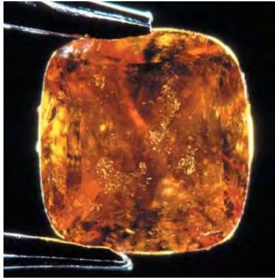
Figure 8. The unpolished surface of this 0.48 ct orange sapphire displayed obvious signs of heat treatment.
