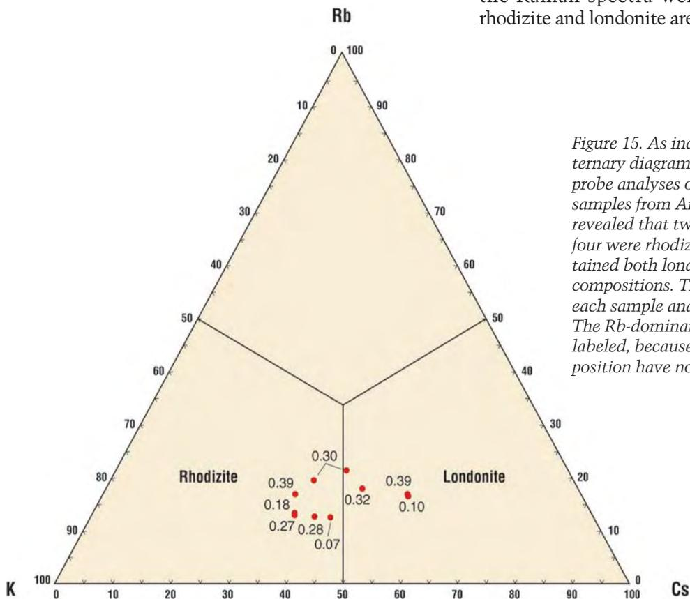
Figure 15. As indicated in this ternary diagram, electron-microprobe analyses of eight faceted samples from Antsongombato revealed that two were londonite, four were rhodizite, and two contained both londonite and rhodizite compositions. The carat weights for each sample analyzed are shown. The Rb-dominant field is not labeled, because stones of this composition have not been recorded.
