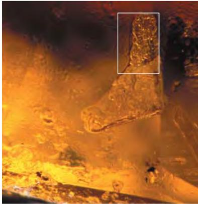
Figure 9. Microscopic examination (at 45 $\times$ ) of the sapphire in figure 8 revealed tabular crystal regrowth after extreme heating.
