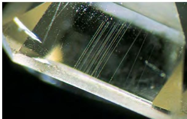
Figure 12. Mineral inclusions were seen in only two of the faceted rhodizite-londonites. One sample contained several colorless chambersite and tiny brownish red columbite inclusions (left). The chambersite inclusions were highly birefringent (right). Photomicrographs by John I. Koivula; magnified 25 $\times$ .
