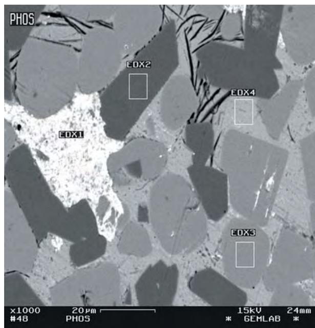
areas (e.g., EDX 1 in figure 25) revealed Pb, Cr, and Sb. The black impurities (as seen in standard viewing conditions) had unusually high contents of Eu and Dy, and appear to be unmelted or exsolved additives of the rare-earth dopant. Some grains (mottled light and dark gray in the BSE-SEM images) had a high content of Zn; the origin and role of this impurity is unclear.
