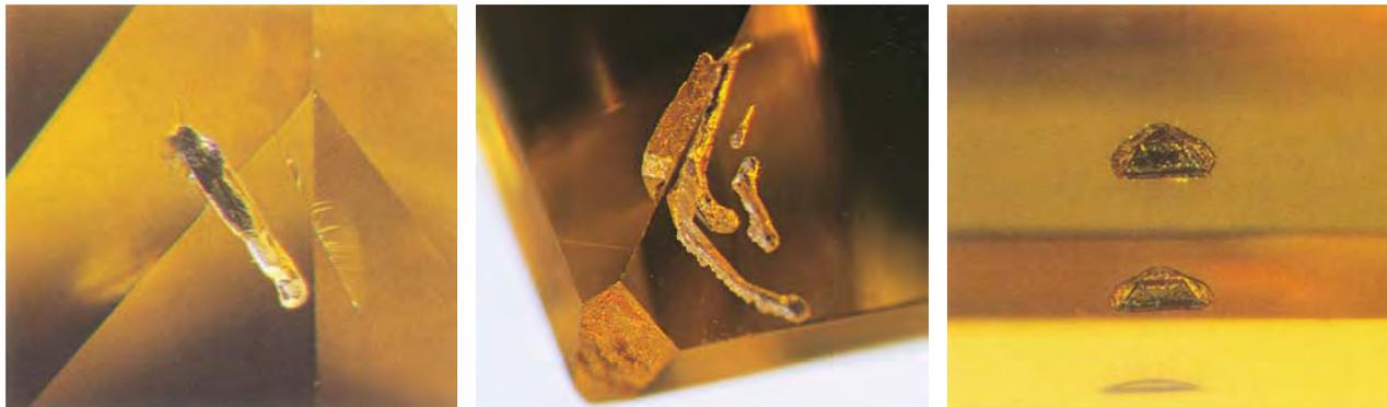
Figure 5. Small metallic inclusions were observed in 10 of the 30 Gemesis laboratory-grown diamonds, three of which are illustrated here. Note in the center image that a small area also shows part of the original crystal surface. The metallic inclusion on the right, seen in direct view and by reflection in two facets, has an equant shape with flat surfaces. Photomicrographs by James Shigley; magnified 75 $\times$ .
