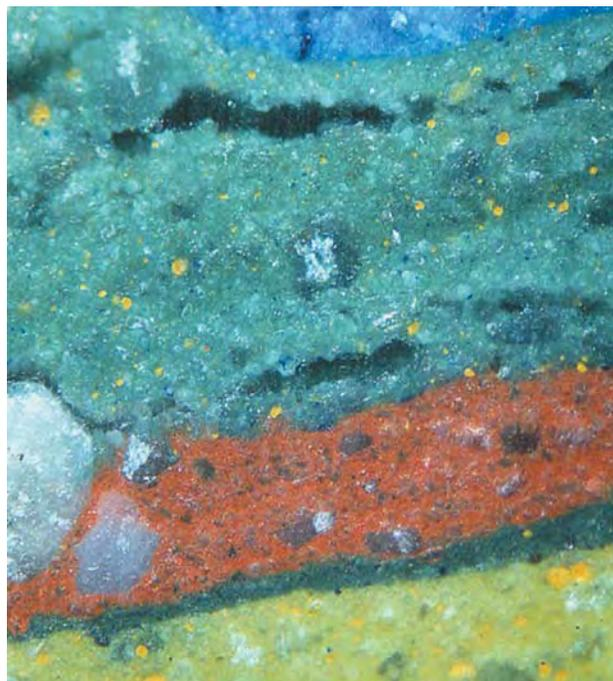
Figure 27. White grains of various sizes are present in all of the color layers of the Rainbow Calsilica, together with smaller grains of blue, green, yellow, and other colors. Photomicrograph by Lore Kiefert; magnified 50×.
