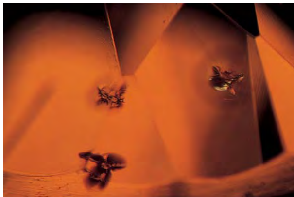
Figure 20. These three minute colorless crystals surrounded by tension fractures appear to be zircon, but they could not be identified by Raman analysis due to their size and position within the stone. Photomicrograph by John I. Koivula; magnified 20 \times .
