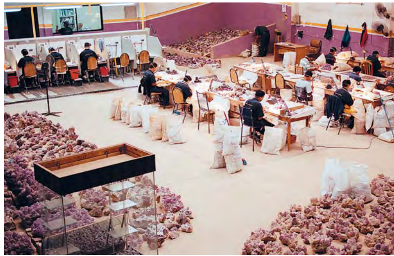
Figure 13. At a processing facility in Santa Cruz, Bolivia, mine-run material from the Anahí mine is washed, cobbled (center and right side), sawn, and pre-formed (left side). Courtesy of Ramiro Rivero.
