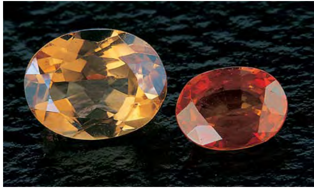
Figure 9. Russian gem treaters are experimenting with surface-coloring technologies using a high-temperature process in the presence of cobalt and other metals and their oxides. This 1.17 ct reddish orange sapphire and 2.62 ct orangy yellow topaz were treated in this fashion. Courtesy of Vladimir S. Balitsky; photo by Maha Tannous.
