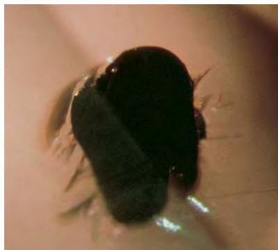
Figure 10. Tabular graphite crystals were identified in a few Bekily garnets, some surrounded by tension cracks. Magnified 50×.
