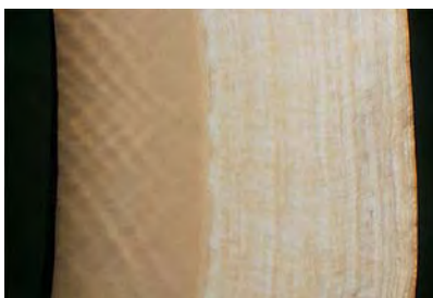
Figure 12. This sample slab of mammoth ivory clearly shows the engine-turned effect in the darker internal layer of the tusk. The outer layer is cementum. Magnified 10×.
