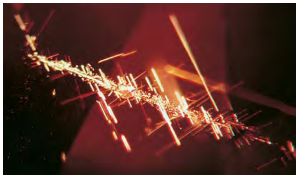
Figure 15. In some samples, mineral inclusions—identified as quartz—were found at the center or tip of rutile needles. Magnified 120 \times .
