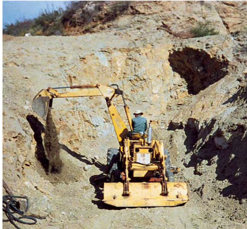
Figure 10. Most of the spessartine production from Ramona came from the Spessartite mine, which was expanded with a backhoe. The pegmatite is dipping into the open cut from the right side. Courtesy of Louis Spaulding Jr.
