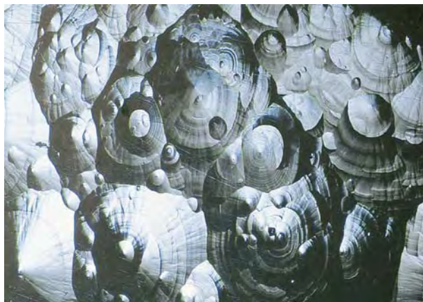
Figure 22. Conspicuous growth hillocks were observed on the as-grown surfaces of the synthetic topaz crystals. Photomicrograph by Taijin Lu; magnified 50×.
