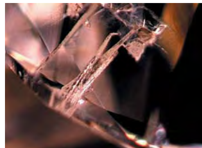
Figure 6. The entry point on the crown best illustrates the fact that these cavities are the result of multiple laser drillings. Note the minute feathers extending off these tubes, which give them a “hairy” appearance. Magnified 100×.
