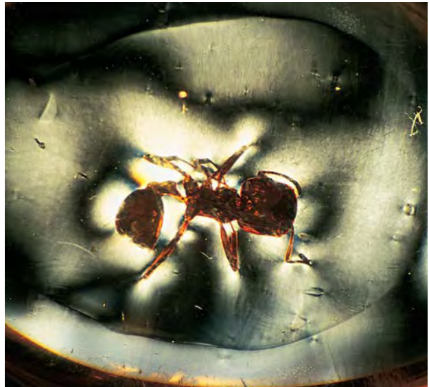
Figure 31. Magnification and polarized light reveal the zone of encapsulation and the strain pattern that developed when this 7-mm-long ant was encased in liquid plastic that subsequently solidified. Photomicrograph by John I. Koivula.
