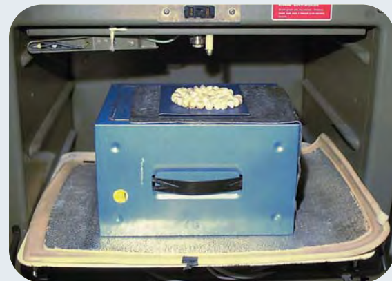
Figure A-3. The samples (here, a baroque strand ranging from 12.0 × 9.15 to 15.20 × 11.15 mm) are placed on the film immediately below the X-ray beam in the Faxitron unit. Photo by E. Schrader.
