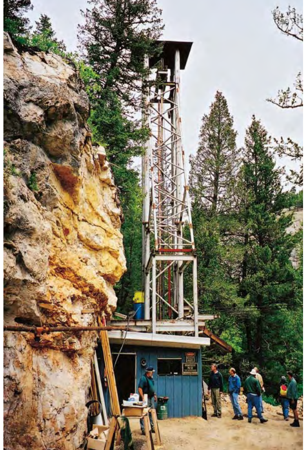
Figure 26. Many improvements have been made at the Vortex sapphire mine at Yogo Gulch, Montana, over the last several years, including this new steel head frame. Photo by K. A. Mychaluk.
