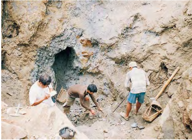
Figure 7. Miners follow the dark-colored amber-bearing horizon in search of Burmite at the Noiye Bum mine, near Tanai, Kachin State, Myanmar. The open-pit area at this mine measures 30 × 120 m. Photo by R. D. Cruickshank.
