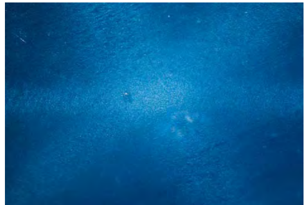
Figure 3. This very fine, unnatural-looking silk (similar in appearance to the silk found in flame-fusion synthetic star rubies or sapphires) is typically seen in a star created by diffusion treatment. Photomicrograph by John I. Koivula; magnified 40×.
