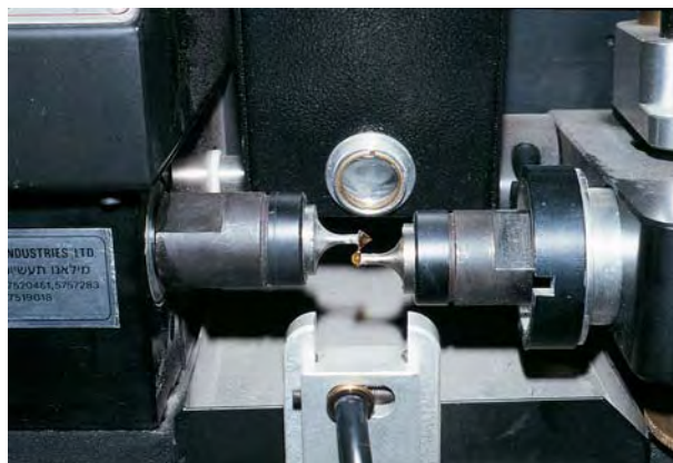
Figure 3. Automatic bruting machines were one of the many innovations in planning and cutting diamond rough in the 1990s. Photo by James E. Shigley.
