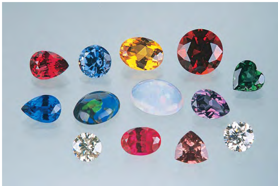
Figure 1. Numerous synthetics and simulants were either introduced or, in most cases, gained or maintained a strong commercial presence during the 1990s. These include, from the top (left to right): Row 1—1.09 ct flux-grown synthetic red spinel, 1.14 ct Czochralski-pulled synthetic blue sapphire, 1.29 ct synthetic citrine, 1.81 ct synthetic red beryl, 0.96 ct Tairus hydrothermal synthetic emerald; row 2—0.83 ct flux-grown synthetic blue spinel, 1.02 ct black and 1.48 ct white Gilson synthetic opal, 0.73 ct hydrothermal synthetic amethyst; row 3—0.43 ct synthetic moissanite, 1.15 ct Tairus hydrothermal synthetic ruby, 0.66 ct Czochralski-pulled synthetic alexandrite, 0.58 ct De Beers experimental synthetic diamond. Photo by Maha Tannous.
