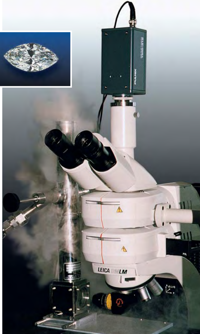
Figure 1. At the end of the 1990s, Raman spectrometry became an important technique for detecting HPHT-processed type IIa diamonds, such as this 0.45 ct E-color GE POL diamond (inset). Photoluminescence spectra (below) obtained with this technique show features—particularly the ratio of the 575 to the 637 nm peak—that can be used to separate the vast majority of HPHT-processed from untreated type IIa diamonds. To achieve high-resolution spectra, the diamonds are cryogenically cooled in a specially designed sample chamber using liquid nitrogen (left). A laser beam is focused through the optical microscope, and a mirror is used to deflect the beam into the sample chamber. Photos by Elizabeth Schrader (inset) and Joe Duffy (left).
