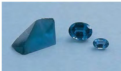
Figure 10. Tairus marketed Russian hydrothermal synthetic sapphires in a broad range of colors that were produced by different trace-element dopants. Left = greenish blue samples, colored by Ni^{2+} and Ni^{3+} (the rough sample is 9.99 ct); center = synthetic ruby (2.17 ct) and pink sapphires, colored by Cr^{3+} ; and right = yellow synthetic sapphires, colored by Ni^{3+} (the largest is 4.74 ct). Photos by M. Glas.
