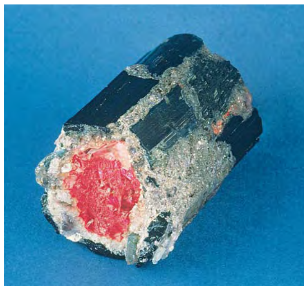
Figure 34. This 667 ct imitation watermelon tourmaline crystal is made up of a complex assembly of several materials; only portions of the outermost surface are tourmaline. Photo by Maha Tannous.
