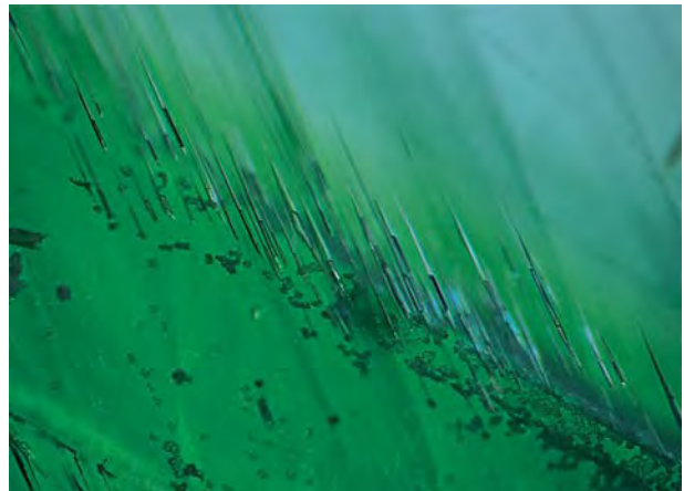
Figure 16. This dense pattern of nailhead spicules and chrysoberyl crystals, usually located near the seed plate, is typical of that seen in the hydrothermal synthetic emeralds produced in Guilin, China. Photomicrograph by John I. Koivula; magnified 30×.
