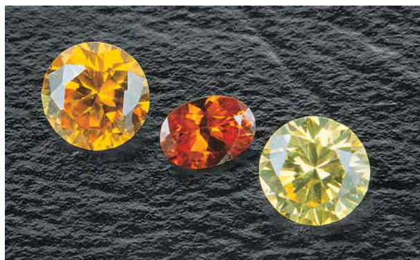
Figure 27. These synthetic zincites (1.35–3.26 ct) were fashioned from material that was an accidental by-product of an industrial kiln process used to produce zinc-based paint in Silesia, Poland. Photo by Maha Tannous.
