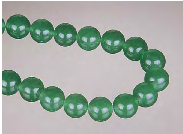
Figure 16. Quartzite dyed green to imitate jadeite, as illustrated by these 8 mm beads, was commonly seen in the 1990s. Photo by Maha Tannous.
