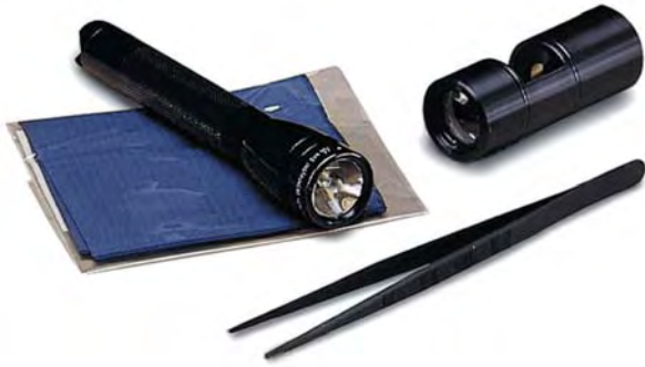
Figure 9. The darkfield loupe, shown here with a flashlight and tweezers, was developed by GIA GEM Instruments to help gemologists see small inclusions.
