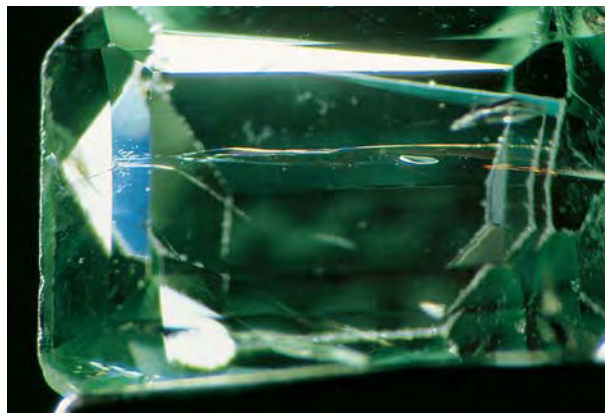
Figure 19. The flash effect is one feature that can be used to identify if an emerald has been filled. The two most common colors, orange and blue, are seen in this stone in a fracture that is otherwise almost invisible. Photomicrograph by Maha Tannous; magnified 15 \times .
