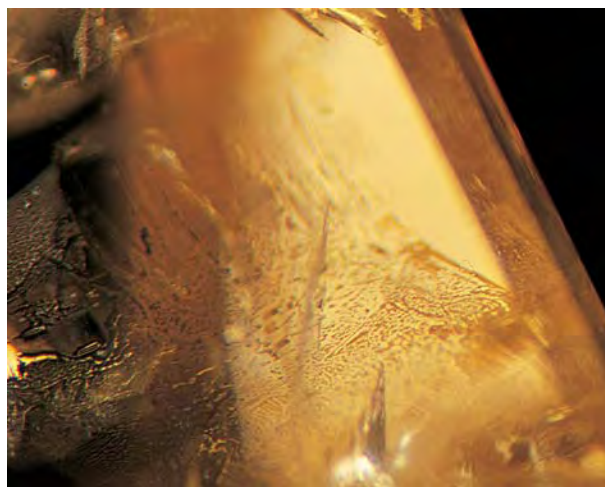
Figure 11. The faceted fresnoites contained numerous partially healed fractures, which are useful in separating them from nearly flawless Czochralski-pulled synthetics. Photomicrograph by John I. Koivula; magnified 15 \times .
