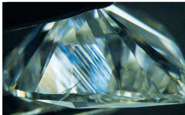
Figure 6. Prior to HPHT processing (left), we observed a banded strain pattern parallel to octahedral growth planes that showed primarily weak (gray) interference colors when viewed between crossed polarizers. After processing (right), the overall pattern remained the same, but the first-order interference colors were slightly stronger (bluer). Note that such strain patterns and interference colors may also be seen in non-enhanced colorless type IIa diamonds. Photomicrographs by Christopher P. Smith; magnified 20 \times .
