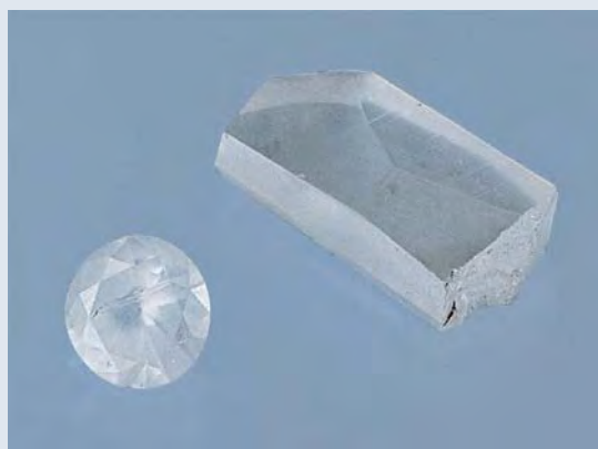
Figure C-1. These type IIa diamonds (1.53 and 0.27 ct) were processed in Russia using an HPHT technique similar to that used by GE. They have a frosted surface because they had not yet been repolished after processing. Photo by Phillip Hitz.
