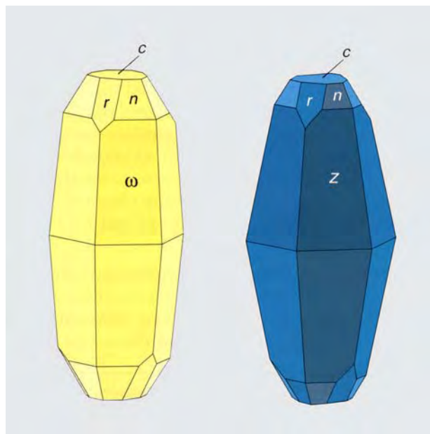
Figure 11. The morphology of Ambondromifehy sapphires is dominated by hexagonal dipyrramids \omega or z combined with the basal pinacoid c . Additional hexagonal dipyrramids n as well as rhombohedra r are also occasionally observed.
