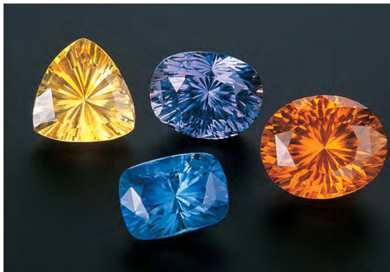
Figure 23. New faceting technology developed by Ohio faceter Richard Homer is being used to intensify the brilliance of sapphires (here, 3.69 to 6.95 ct) by placing concave facets on their pavilions. Courtesy of Schorr Marketing and Sales; photo by Maha Tannous.
