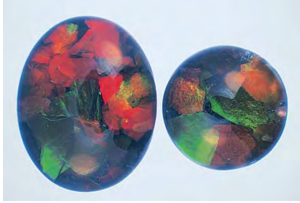
Figure 2. Composed of tiny angular flakes of iridescent ammonite shell encased in a plastic that is sandwiched between a glass cap and a black opaque backing material, these two assembled cabochons make attractive use of otherwise unusable fragments. The oval measures 9.90 \times 7.58 \times 3.59 mm, and the round piece measures 7.01\text{--}7.09 \times 3.08 mm. Photo by John I. Koivula.
