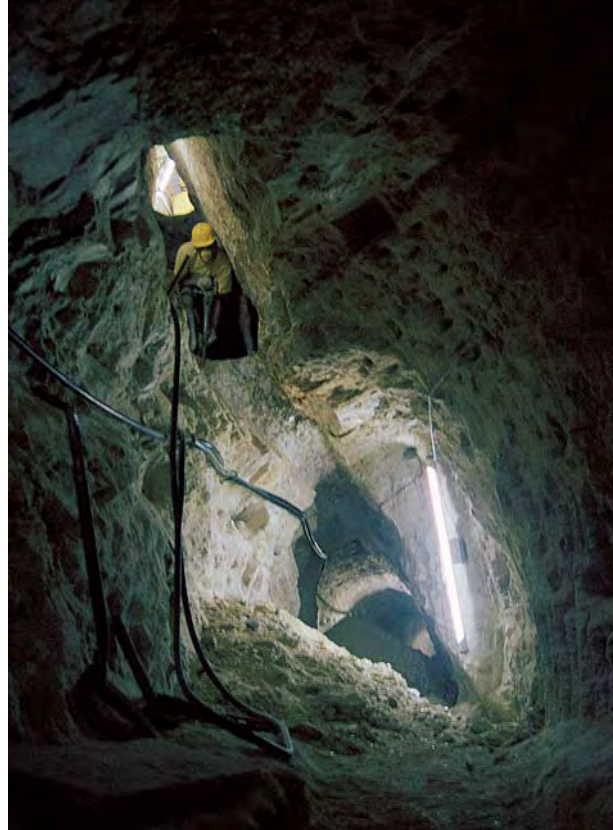
Figure 17. Underground mining has resumed at the historic São José da Batalha tourmaline mine in Paraíba State, Brazil. Here, miners use pneumatic hammers to excavate the 40-cm-wide pegmatite dike. Photo by Brendan Laurs.
