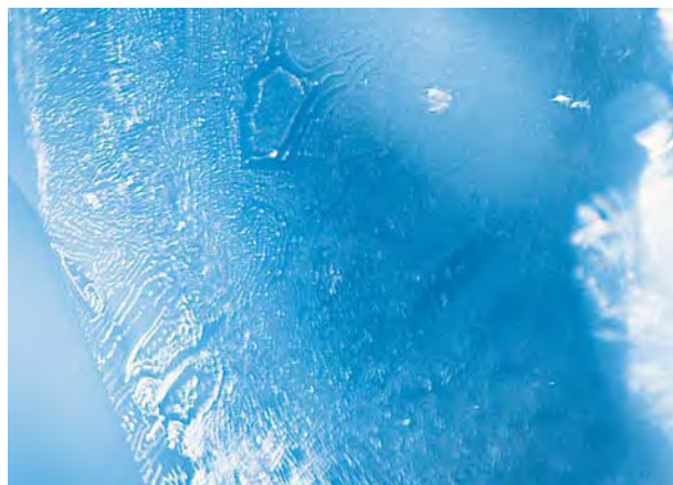
Figure 10. In a number of the haüynes, the partially healed fissures resembled the glass fillings seen in some rubies. Photomicrograph by H. A. Hänni; magnified 30 \leftrightarrow .
