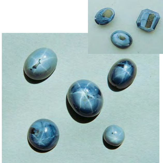
Figure 10. Star sapphires from Ambondromifehy are commonly gray to blue. The largest cabochon here measures 9 \times 10 mm. The sapphires in the inset have been cut to show the unusual cores seen in some of the samples; the faceted stone is 10 \times 11 mm. Photos by M. Glas.
