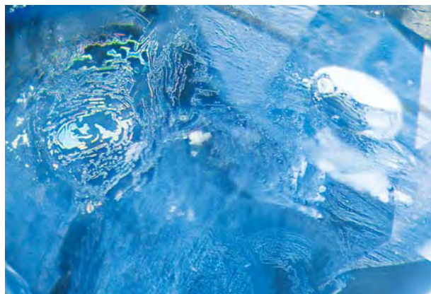
Figure 8. Commonly seen in the haüynes examined were well-formed negative crystals with rosette-like healing fissures (right, within the bright spot) or partially healed fissures with interference colors and a worm-like "fingerprint" structure (on the left). Photomicrograph by H. A. Hänni; magnified 40 \times .
