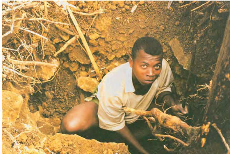
Figure 4. Miners at Ambondromifehy have found that digging around the roots of trees is the easiest way to recover sapphires. Photo by J. Kanis.
