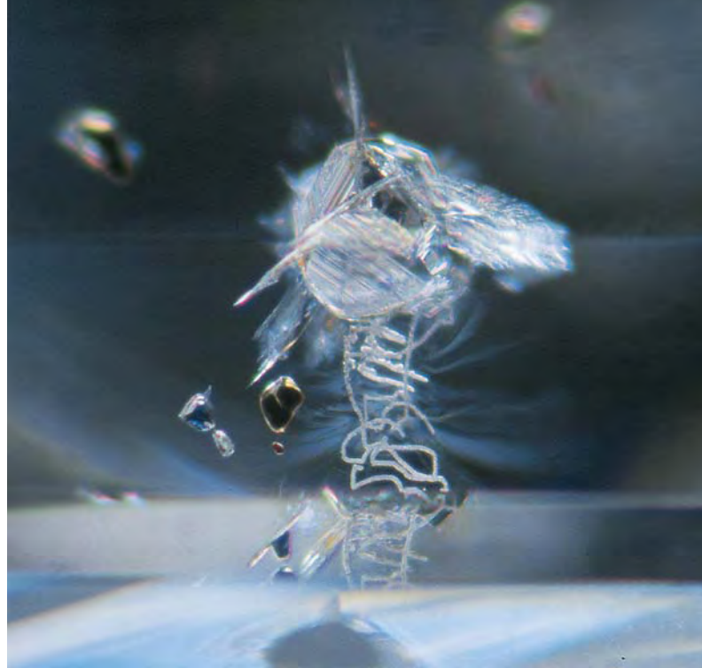
Figure 1. The appearance within feathers of unnatural, irregular, wormhole-like channels provided the first clue that a new laser treatment had entered the market. Photomicrograph by Vincent Cracco; magnified 63 \times .
