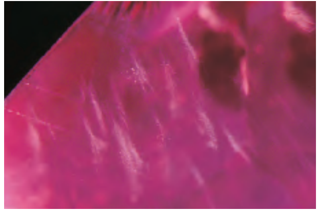
Figure 27. Other distinctive inclusion patterns showed a brush-stroke or more nebulous appearance. Photomicrograph by Christopher P. Smith; magnified 30 \times .
