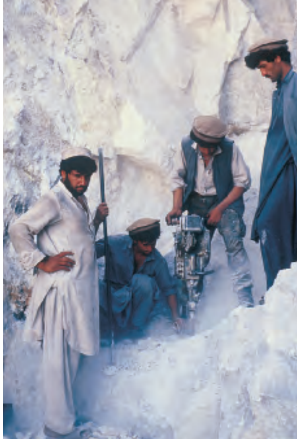
Figure 6. Mining at Jegdalek is small scale. The only mechanized equipment consists of a few pneumatic hand drills. Photo by Gary Bowersox.
