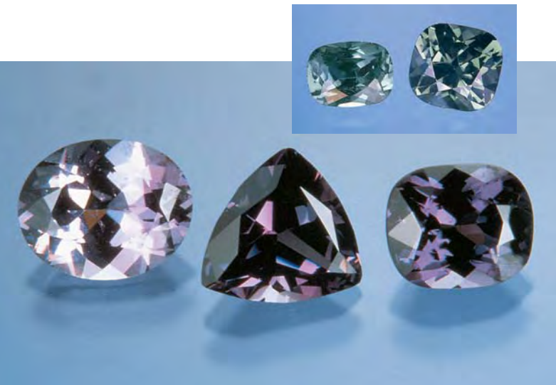
Figure 17. These three violet to purplish violet spinels from Ilakaka, Madagascar, are predominantly colored by iron; the samples weigh 1.30–1.67 ct. Inset: Two bluish green samples (1.21 and 0.78 ct), also colored by iron, represent spinel colors that have been seen only rarely in lots from Ilakaka. Photos by Maha Tannous.
