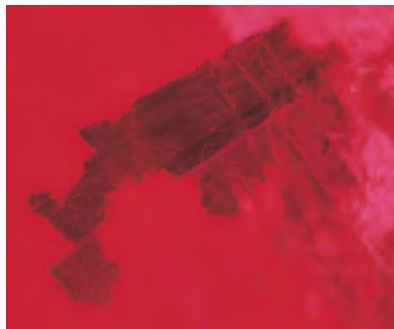
Figure 22. One distinctive inclusion feature in the rubies and fancy-color sapphires from Jegdalek consists of iron sulfide minerals such as pyrite, marcasite, and pyrrhotite that were present along healed fracture planes (left; magnified 20×) and parting planes (right; magnified 15×). Photomicrographs by Christopher P. Smith.
