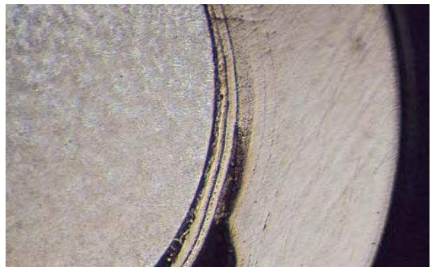
Figure 14. With magnification and reflected light, the two generations of nacre, separated by a gap, are clearly visible in the Kasumiga cultured pearl shown in figure 13. The relatively high manganese content of the outer layer proved that it formed in fresh water rather than salt water. Photo by H. A. Hänni.
