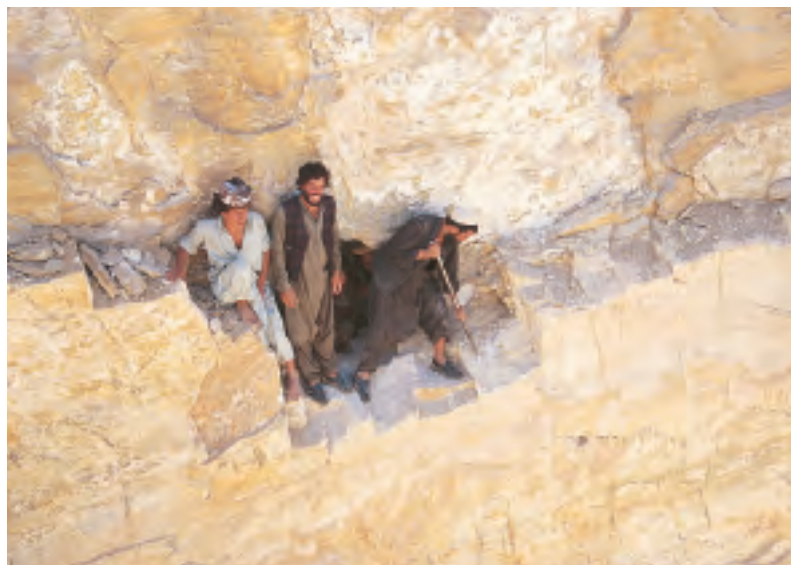
Figure 5. Workers remove marble with prybars to uncover the gem corundum at Jegdalek. Most of the mining techniques used today are the same as those reported by Griesbach in 1892. Photo by Gary Bowersox.
