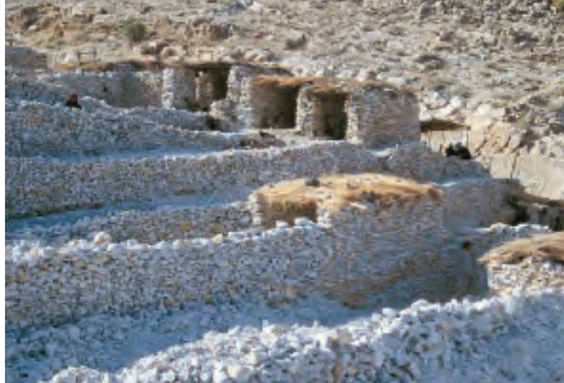
Figure 8. Marble from the trenches is used to build shelters for the miners, where the corundum is sorted. Working conditions are better than in other mines in Afghanistan, as the ruby and sapphire mines are lower in altitude and accessible all year. Photo by Gary Bowersox.
