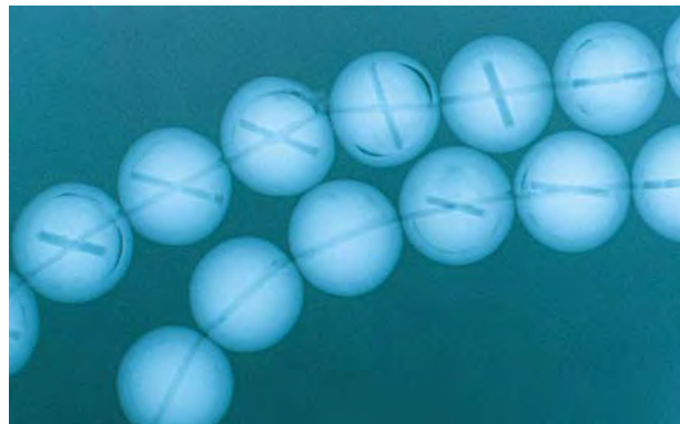
Figure 12. Most of the cultured pearls in this X-radiograph of a strand of Japanese Kasumiga cultured pearls reveal the drill hole through the bead nucleus as an oblique line (the length of which depends on its inclination to the direction of observation) that ends at the thicker nacre layer. X-radiograph by H. A. Hänni.
