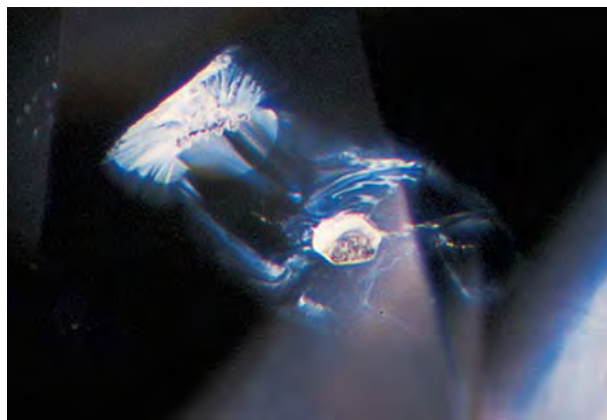
Figure 13. The new laser treatment has extended the feather surrounding the crystal in this stone to reach the surface. The preexisting feather is very transparent in this photo, while the new portion is much more reflective. Photomicrograph by Shane F. McClure; magnified 40 \times .
