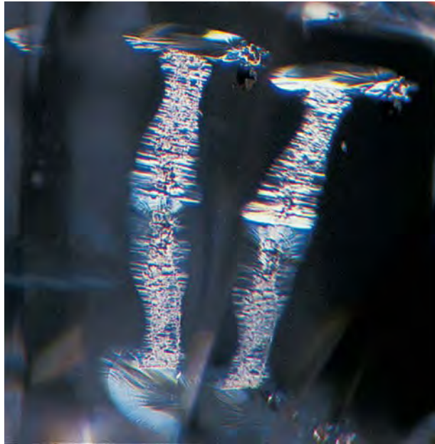
Figure 6. This treatment may be used to produce tiny cleavages that form a step-like progression from the inclusion to the surface of the diamond. In this way, the treater can take the shortest route to the surface, even if that route does not correspond to a cleavage direction. (Note that the single feature is duplicated here in a facet reflection.) Photomicrograph by Shane F. McClure; magnified 40×.
