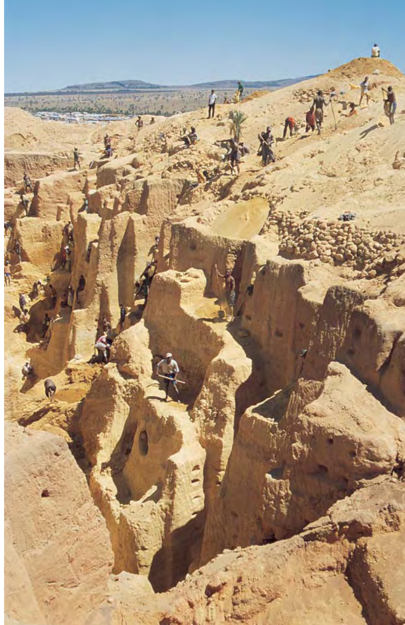
Figure 10. At Ilakaka, Madagascar, miners dig pits through the weathered sandstone to reach the productive gem-bearing conglomerate layers. At the time this photo was taken (December 1999), this was the largest hand-dug excavation at Ilakaka. Photo by Brendan Laurs.
