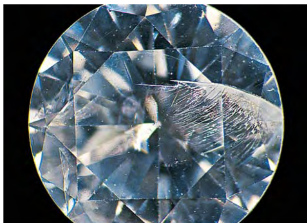
Figure 11. Note the filled break (with a yellow flash effect) along the right edge of this 0.35 ct Oved filled diamond before it was subjected to durability testing (left). After the diamond was heated in a muffle furnace (in air) for 15 minutes at almost 700°C, damage is evident in the filled area (right), as well as in the diamond itself (seen here as small whitish areas on the surface). Photomicrographs by John I. Koivula.
