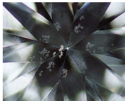
Figure 7. The opaque dendritic cloud seen in this 0.21 ct synthetic blue diamond is reflected in the facets around the lower pavilion. Magnified 63 \times .
