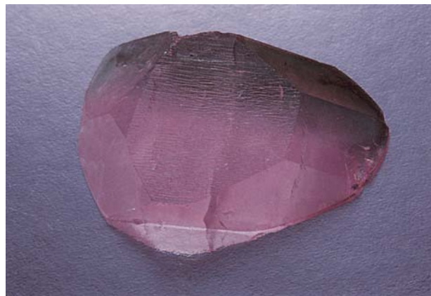
Figure 25. This 43.24 ct hydrothermal synthetic morganite beryl was grown on a seed plate of synthetic emerald; the resulting color combination resembled bicolored tourmaline. Courtesy of Tom Chatham, Chatham Created Gems; photo by Maha Tannous.
