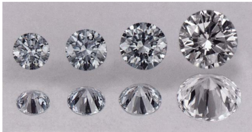
Figure 5. As seen both face-up and through the pavilion, the three synthetic blue diamonds on the left (0.10, 0.14, and 0.21 ct) are considerably paler than most of the synthetic blue diamonds seen in the laboratory to date. Nevertheless, their blue color is clearly evident when compared to the near-colorless diamond on the far right.
