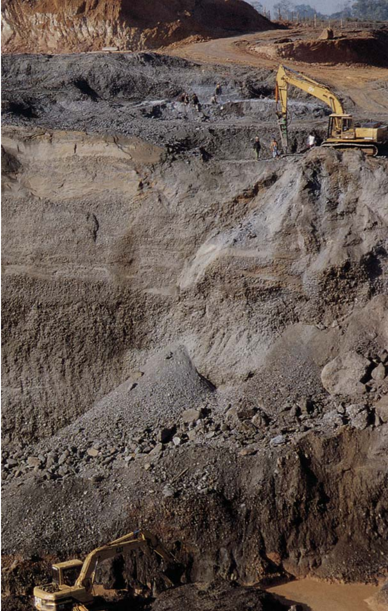
Figure 11. At Nansibon, backhoes are used to work the serpentinite boulder conglomerate in which jadeite boulders occur in narrow horizontal concentrations. Photo by George E. Harlow.
