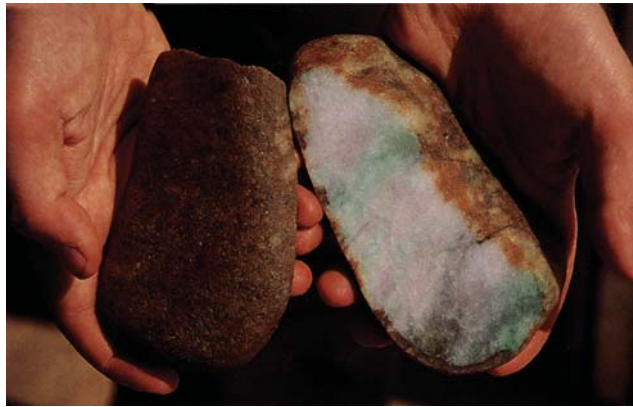
Figure 14. Top left: This jadeite boulder shows the relatively thin skin and potentially good color that is usually associated with “river jade.” Although from the outside this appears to be a normal jadeite boulder, oxidants that entered through cracks on the surface have produced a large area of discoloration. Bottom left: Note the thick yellow “mist” around the jadeite in this boulder of “mountain jade.” Right: A key advantage to jadeite taken from in situ deposits is that the quality of the material is readily apparent. Photos © Richard W. Hughes.
