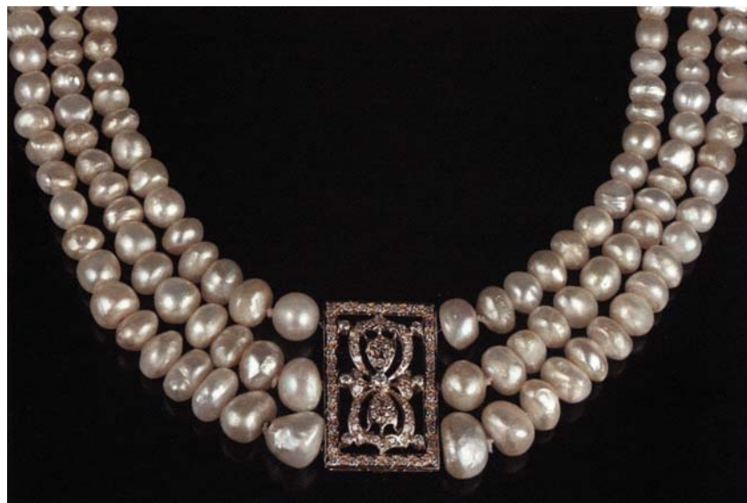
Figure 11. Most of the natural baroque pearls ( 4.30 \times 4.90 mm to 10.89 \times 13.70 mm) in this triple strand show a worn, uneven, near-colorless coating.
