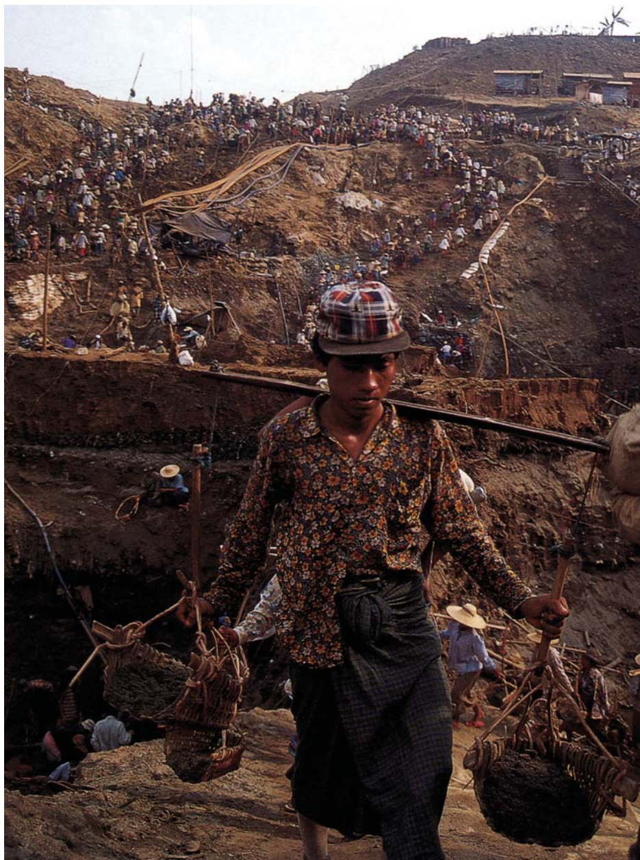
Figure 8. Thousands of workers remove the dirt and gravel at Hpakangyi to reach the Uru conglomerate and its promise of fine jadeite. Using the most rudimentary of carrying devices—two crudely fashioned bamboo buckets—this young miner leads a trail of laborers up the steep path from the bottom of the pit to a truck that will carry the waste to the river. Photo © Richard W. Hughes.
