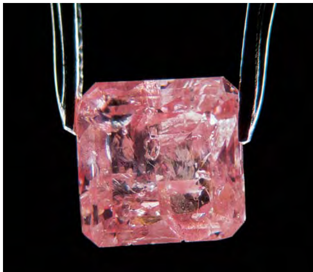
Figure 5. The many white fractures in this 1.39 ct Fancy Intense Pink emerald-cut diamond (left) detract from the color. After the diamond was subjected to several episodes of fracture filling, most of the fractures appeared to be transparent and the stone revealed a highly saturated pink color in the face-up color-grading position (right). However, now that the diamond has been treated, the Gem Trade Laboratory can no longer issue a color grade for it.
