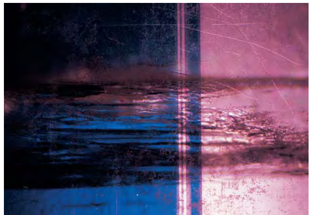
Figure 11. Only slight finger pressure was required to cause a shift in the twin pattern in this block of neodymium penta-phosphate. Photomicrographs by John I. Koivula; polarized light, magnified 10×.
