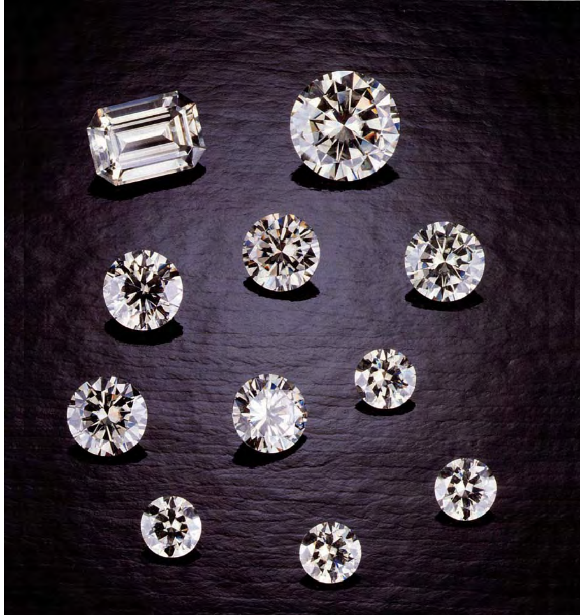
Figure 1. Near-colorless synthetic moissanite is being marketed for jewelry purposes as a diamond imitation. The faceted pieces shown here, weighing from 0.09 to 0.57 ct, illustrate the appearance of this material. Because synthetic moissanite is doubly refractive, one can sometimes see doubling of the back facet junctions even with the unaided eye (particularly noticeable in the large round brilliant in the upper right). Photo © GIA and Tino Hammid.
