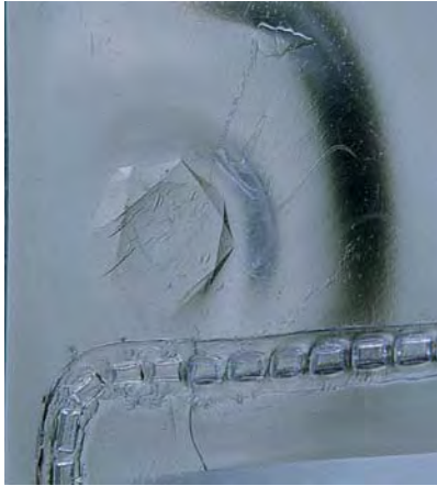
Figure 4. The inside surface of the plastic lid shown in figure 3 carried an impression of the 5.56 mm table of the diamond that had transferred heat to it.
