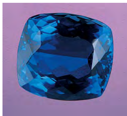
Figure 2. This 16.40 ct highly saturated treated-color violetish blue beryl was being sold as a tanzanite simulant. Unfortunately, this color in beryl is unstable to light and heat.
