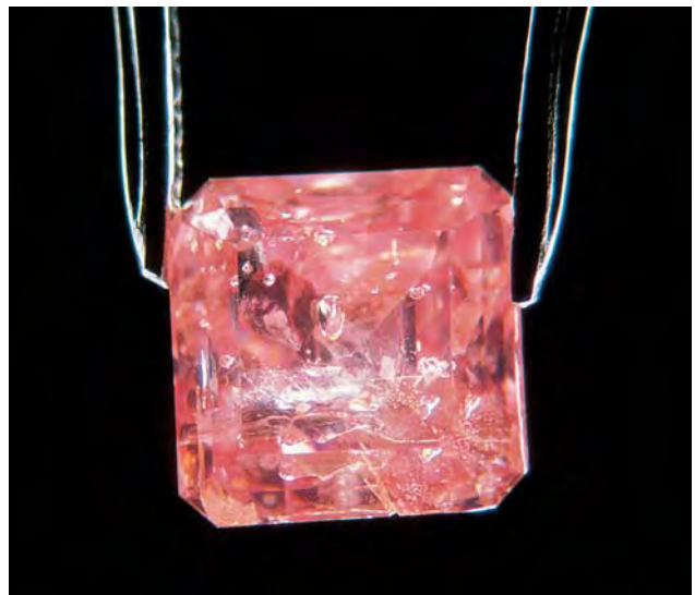
Figure 5. The many white fractures in this 1.39 ct Fancy Intense Pink emerald-cut diamond (left) detract from the color. After the diamond was subjected to several episodes of fracture filling, most of the fractures appeared to be transparent and the stone revealed a highly saturated pink color in the face-up color-grading position (right). However, now that the diamond has been treated, the Gem Trade Laboratory can no longer issue a color grade for it.
