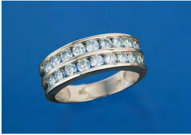
Figure 4. This 14k gold ring contains two rows of faceted light-green synthetic moissanites, which were mounted in wax and then cast in place with no apparent damage to the material. All of the stones reacted as synthetic moissanite on the Model 590 tester. Ring courtesy of C3 Inc.; photo by Maha DeMaggio.
