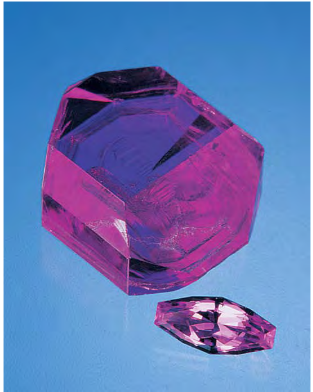
Figure 10. Illustrated here are the largest known crystal (136.89 ct) and the only known cut sample (5.33 ct) of neodymium penta-phosphate. Photo by Maha DeMaggio.
