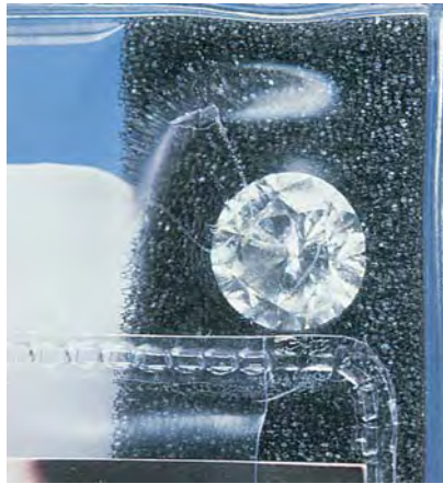
Figure 3. This 2.40 ct round brilliant diamond melted the lid of the plastic box in which it was held and discolored a piece of thermal paper nearby, shown here at the bottom.
