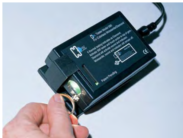
Figure 3. The Colorless Moissanite/Diamond Tester Model 590 was designed and built by C3 Inc. for the sole purpose of rapidly distinguishing synthetic moissanite from diamond only after a stone has been identified as “diamond” on a thermal probe. Photo by Maha DeMaggio.
