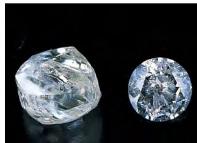
Figure 6. The owner of these two diamonds, a 2.93 ct crystal and a 0.73 ct round brilliant cut diamond, hoped that GTL could explain why the stones had apparently fractured spontaneously during routine storage.
