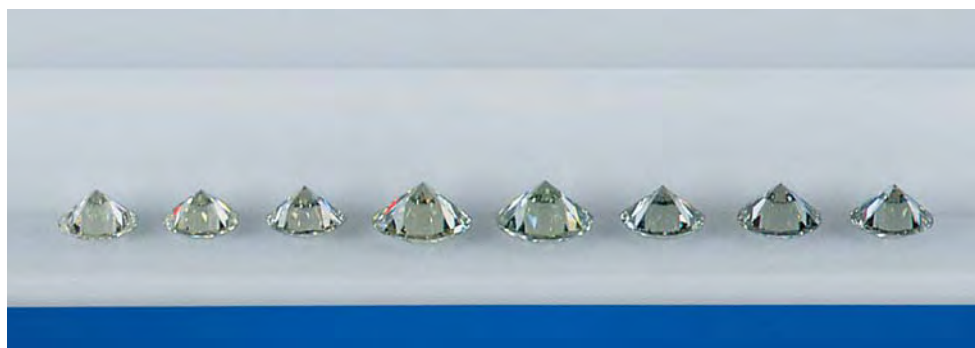
Figure 5. The synthetic moissanites examined at GIA ranged in color from approximately I to U-V on the GIA color-grading scale for diamonds. This range was most evident when the samples were placed table-down and viewed side-by-side in a white plastic tray, as illustrated here. All of the stones had a somewhat gray, green, or yellow appearance. The two largest samples shown here are 1.12 and 1.05 ct. Photo by Shane F. McClure.
