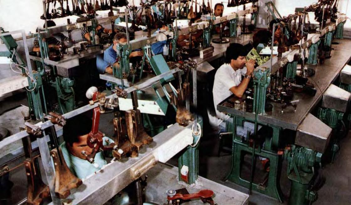
Figure 20. Polishers use a wide variety of tongs (shown here in the foreground and hanging on the central bars), depending on the facets being polished, the shape of the stone, and the like.
