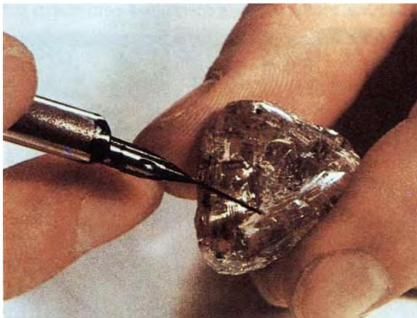
ences, such as in the number, visibility, position, and size of internal features (inclusions, fractures, etc.), as these features would appear in the final faceted stone. The uneven surface of the rough diamond often makes internal features difficult to see. The manufacturer must envision the shape and orientation of the stone within the rough crystal, and judge where these internal features may be located and how visible they will be, or whether any or all can be removed by cutting.
