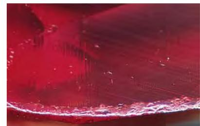
pavilion was doubly refractive, fluoresced moderate red to both long- and short-wave UV radiation, and revealed both curved striae and small gas bubbles with magnification (again, see figure 15). The absorption spectrum, which could only be observed for the doublet as a whole, was typical for ruby. These properties identified the pavilion as synthetic ruby.
