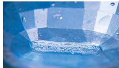
be distinct, both sapphirine and serendibite are so rare that we did not have reference spectra or even reference stones to which we could compare the spectrum we took. An EDXRF chemical analysis showed silicon, aluminum, magnesium, calcium, iron, and minor amounts of titanium, which is consistent with the chemical formula for serendibite. X-ray diffraction analysis proved conclusively that the gem was serendibite.
