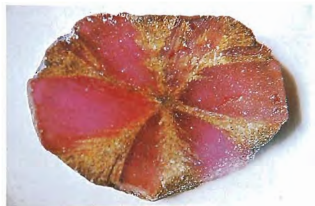
Figure 7. The arms in this 4 × 6 mm trapiche ruby slab “feather out” and widen toward the outer edge of the crystal, almost completely absorbing one of the ruby sectors.
