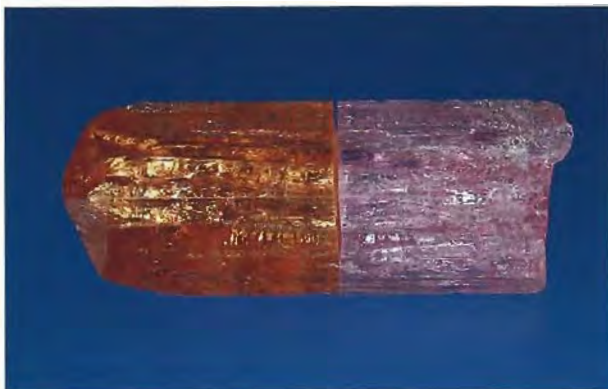
Figure 12. This 97.59 ct Imperial topaz crystal was sawn in half and the bottom was heated to 1050°F, which produced the purplish pink color. Photo by Shane F. McClure.
