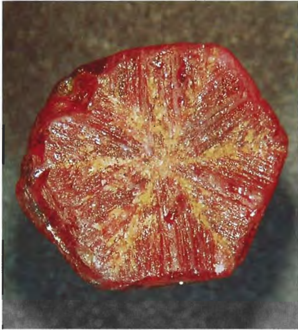
Figure 2. The six-rayed (hexagonal) star in this 7.5-mm-diameter trapiche ruby separates the ruby into six triangular sectors. Note the surface striations oriented perpendicular to the six dipyramidal faces of this crystal, almost parallel to the basal pinacoid.
