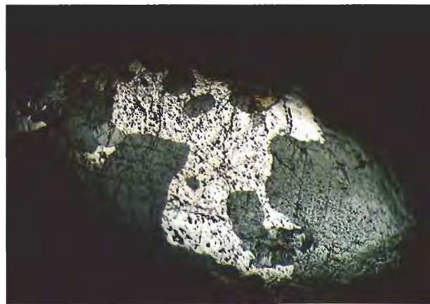
Figure 7. The ilmenite crystal in this black labradorite moonstone cabochon looks white when viewed with low-angle oblique illumination. Photomicrograph by John I. Koivula; magnified 20 \times .
