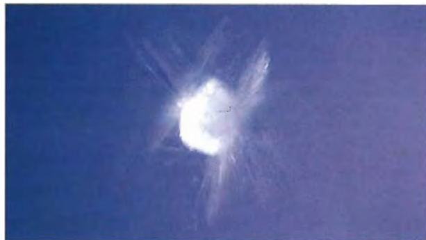
Figure 9. Various crystal phases were seen in this Ca-phosphate glass. Magnified 100 \times .
