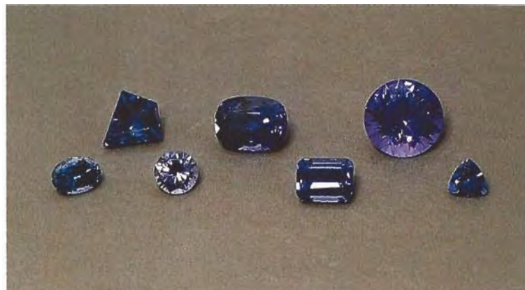
Figure 1. Several manufactured materials have appeared on the gem market as tanzanite imitations. A number of these are shown here together with two natural tanzanites. From left to right: (top row) two tanzanites (3.03 ct and 5.89 ct) and a 6.90 ct sample of Ca-phosphate glass; (bottom row) a 1.64 ct synthetic corundum (called Blue Coranite), a 1.99 ct synthetic garnet from Russia, and two samples (2.89 ct and 0.92 ct) of heavy glass (U.M. Tanzanic). Photo by H. A. Hänni.
