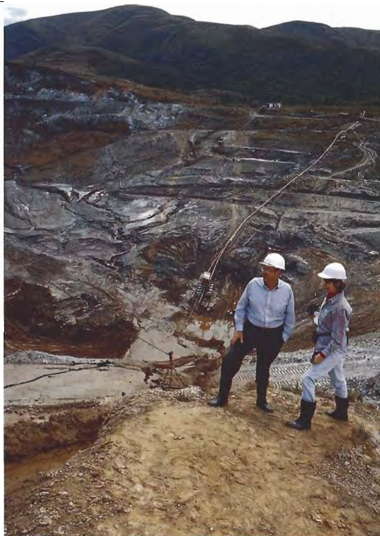
Figure 3. In August 1996, the larger pit at the Capão mine was 30 m deep and approximately 350 m long. Toward the bottom of the pit, a water cannon softens the weathered host material and creates a slurry that is then pumped out of the pit. One of the mine owners, Dr. Wagner Colombarolli, is standing at the upper edge of the pit with one of the authors. Photo by Daniel A. Sauer.
