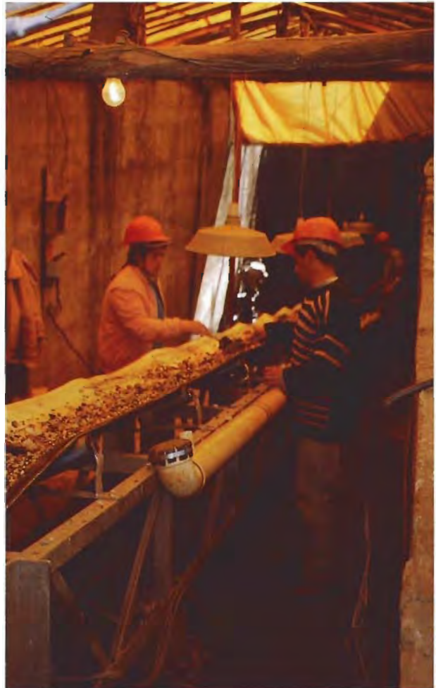
Figure 8. In a shed-like structure behind the main pit, miners manually sort through the concentrate, searching for topaz. Any topaz found is placed in tubes along either side of the conveyor belt. Photo by Daniel A. Sauer.
