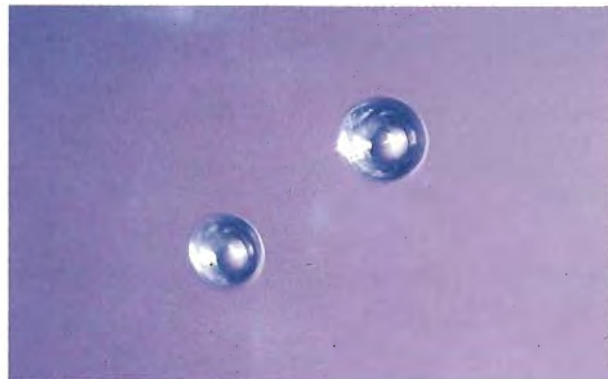
Figure 8. Bubbles help show that this is a Ca-phosphate glass. Note also the needle-like devitrification features on the large bubble. Magnified 100 \times .
