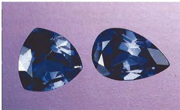
Figure 15. The 4.01 ct modified brilliant pear shape and 3.84 ct triangular modified brilliant shown here are synthetic spinel triplets, imitating tanzanite. Photo by Maha DeMaggio.
