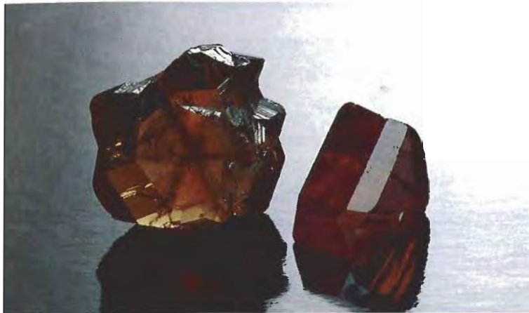
Figure 3. The Russian flux-grown synthetic alexandrite crystals examined were either single crystals (right, 9 × 7 mm) or cyclic pseudohexagonal twins (left, 12 × 11 mm), which are shown here in incandescent light. Photo © GIA and Tino Hammid.
