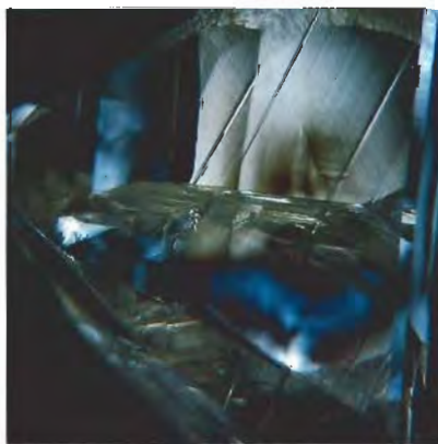
Figure 7. First-order interference colors—shades of blue—seen here in the partly polished 18.15 ct piece were actually present in both halves, indicating the presence of residual strain. Magnified 10 \times .
