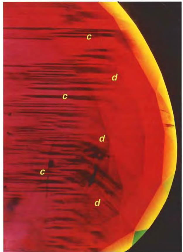
Figure 15. Basal pinacoid c planes dominated the growth structures seen in this 25.55 ct natural ruby, which was reportedly from Burma (Myanmar). The subordinate negative d planes were more prominent during the earlier stages of this gemstone's growth (creating an angle of 141.8 ^\circ ). The dark bands are concentrations of rutile needles oriented parallel to the growth planes. Immersion, magnified 15 \times .
