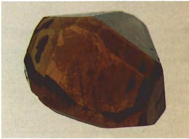
Figure 4. This 3 × 4 mm untwinned synthetic alexandrite single crystal was grown by spontaneous nucleation without crucible contact. (The darkish patches on some crystal faces are the result of carbon coating for microprobe analysis.) Photomicrograph by John I. Koivula.
