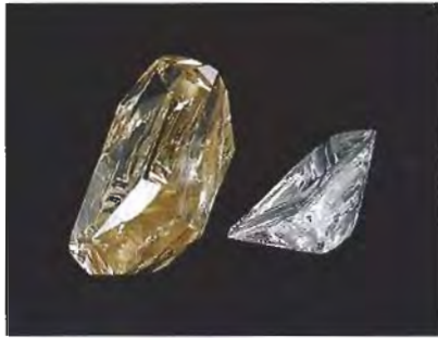
Figure 2. These two pieces are from the same brownish yellow rough diamond. Nearly all the color ended up in the 7.32 ct portion, whereas the 1.35 ct piece is near-colorless.
