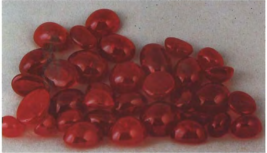
Figure 12. Note the uniformity of color in these cabochons (1-4 ct), all of which proved to be quench-crackled synthetic rubies.
