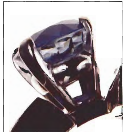
Figure 16. A side view of the stone in figure 15 shows that the color is confined to the crown, but there is no cement plane.
