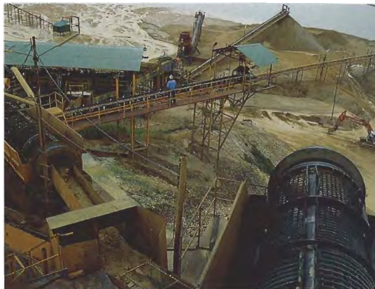
Figure 14. At S.A.P. Mining's modern washing plant near Bo Phloi in Kanchanaburi Province, Thailand, a huge rotating trommel (foreground, right) removes the larger rocks. The gravels then pass through one of two other trommels with smaller mesh sizes, one of which is at left. Photo by Robert C. Kammerling.
