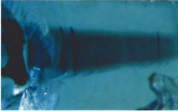
Figure 13. Commonly seen in the Andranondambo sapphire crystals was a central zone with a cone- (as here) or pipe-like appearance. Such central zones are delineated by planes parallel to the basal c face and by repetitive dipyramidal (n,z) faces. These central zones are similar in appearance to those observed in Mong Hsu (Myanmar) rubies. Magnified 60X.
