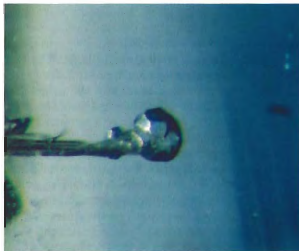
Figure 23. It was not uncommon in the Madagascar sapphires to see minerals like this calcite crystal accompanied by a tube-like inclusion. Magnified 40 \times .
