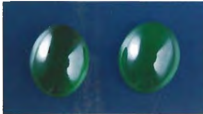
Figure 5. These natural-color jadeite cabochons appeared red when examined with a Chelsea color filter, which could lead a gemologist to falsely suspect that they were dyed.
