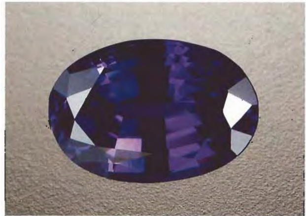
Figure 22. This 7.07 ct tanzanite imitation—which contains yttrium, aluminum, and europium—has a very convincing color. Courtesy of Bill Vance; photo by Maha DeMaggio.
