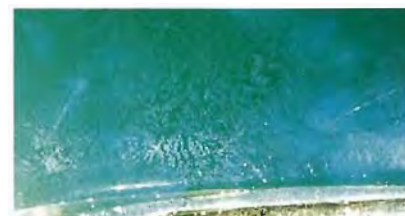
Figure 7. Microscopic examination of the jade imitation in figure 6 revealed the fern-like pattern that results from the devitrification (partial crystallization) of glass. Magnified 20x.
