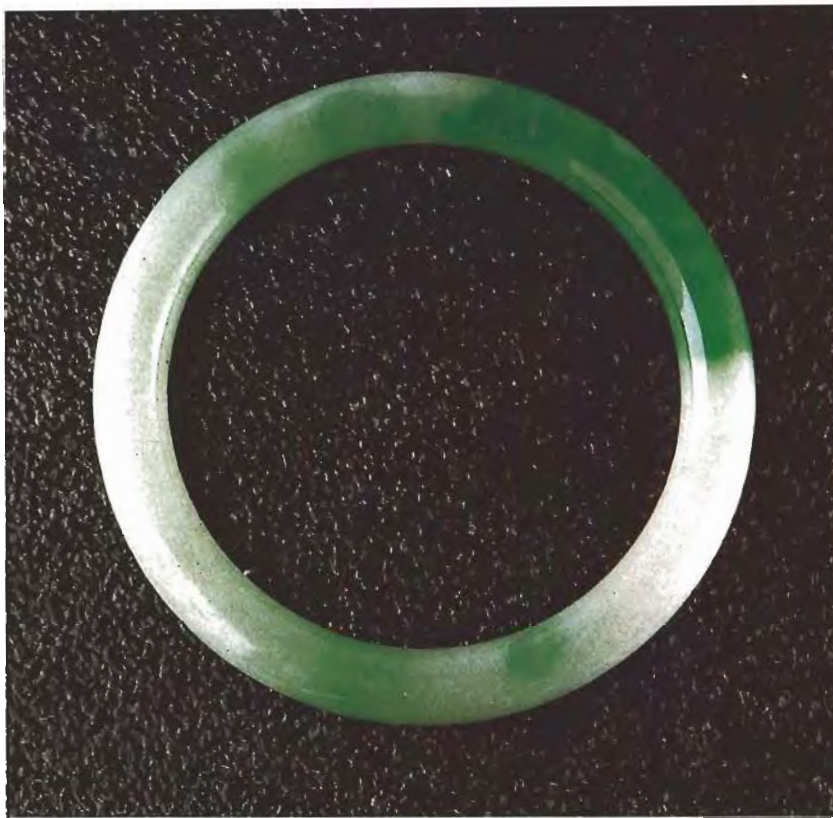
Figure 6. Characteristic surface features indicated, and IR spectroscopy proved, that this jadeite bangle bracelet had been bleached and polymer impregnated.
