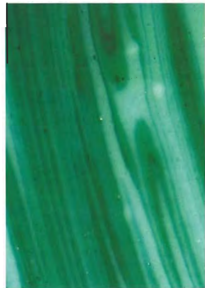
Figure 8. Banding can be seen in this 9 × 11 mm segment of a necklace. The swirled appearance of one of the bands helped identify the material as a malachite imitation. Magnified 10×.
