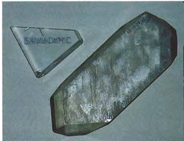
Figure 15. The Russian State Enterprise VNIISIMS also synthesizes calcite hydrothermally for technical applications. Note the strong doubling through the smaller of the two crystals on the left. Photo by Robert C. Kammerling.
