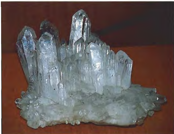
Figure 14. These synthetic quartz crystals have been hydrothermally grown on a natural quartz base (more than 12 inches—30 cm—across). Photo by Robert C. Kammerling.
