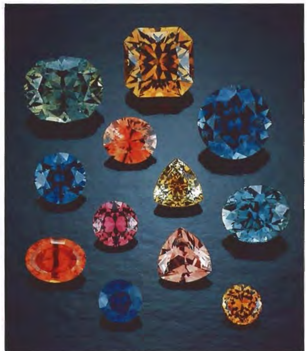
Figure 9. These sapphires (0.66–5.69 ct) are from the Dry Cottonwood Creek, Gem Mountain, and Eldorado Bar alluvial deposits in Montana. All except the pink one have been heat treated by Crystal Research. Courtesy of American Gem Corp.; photo © 1994 Tino Hammid.
