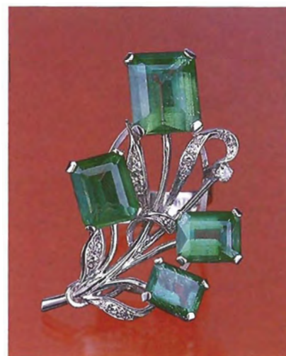
Figure 6. The four green stones in this pin, which range from approximately 8.2 × 6.1 × 3.8 mm to 11.7 × 9.5 × 7.7 mm, are synthetic emerald overgrowths on natural beryl.
