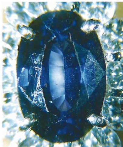
Figure 12. Abraded table facet junctions are readily seen on this approximately 4-ct diffusion-treated sapphire which has been set in a ring with diamonds.
