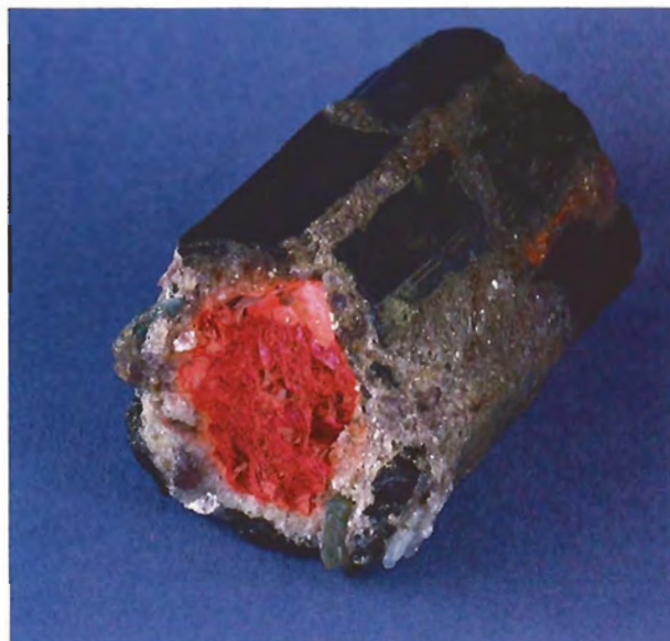
Figure 14. This 667.74-ct imitation watermelon tourmaline "crystal" specimen is actually a complex assembly of several materials. Photo by Maha Smith-DeMaggio.
