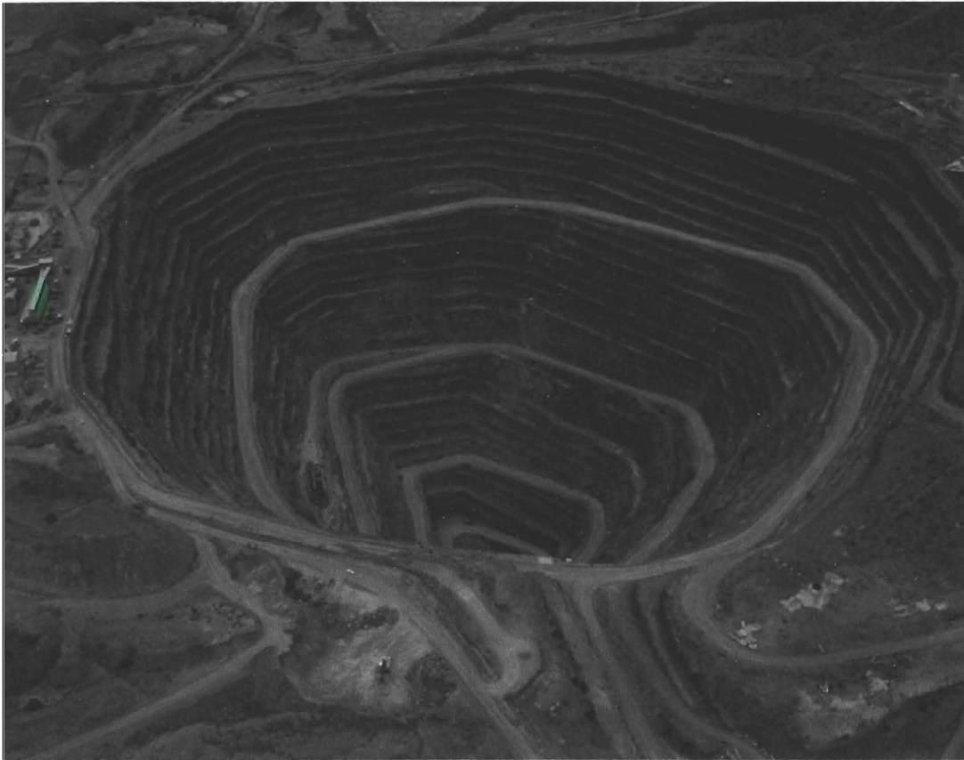
Figure 6. Presently, the Finsch mine is the largest producer of diamonds in South Africa, with production in 1990 of 4,177,572 ct (De Beers Consolidated Mines, 1992), although the rough averaged only 0.03 ct per stone. When the pipe was discovered in 1960, an estimated 1400 m of kimberlite had already been eroded away and the outcrop at the surface was 44.2 acres (17.9 ha). This photo, taken in September 1990, reflects the cone shape characteristic of kimberlite pipes and that the mine is pinching out at depth (present depth approximately 600 m). Note that the area shown here is larger than the original pipe because of the requirements of open-pit mining.
