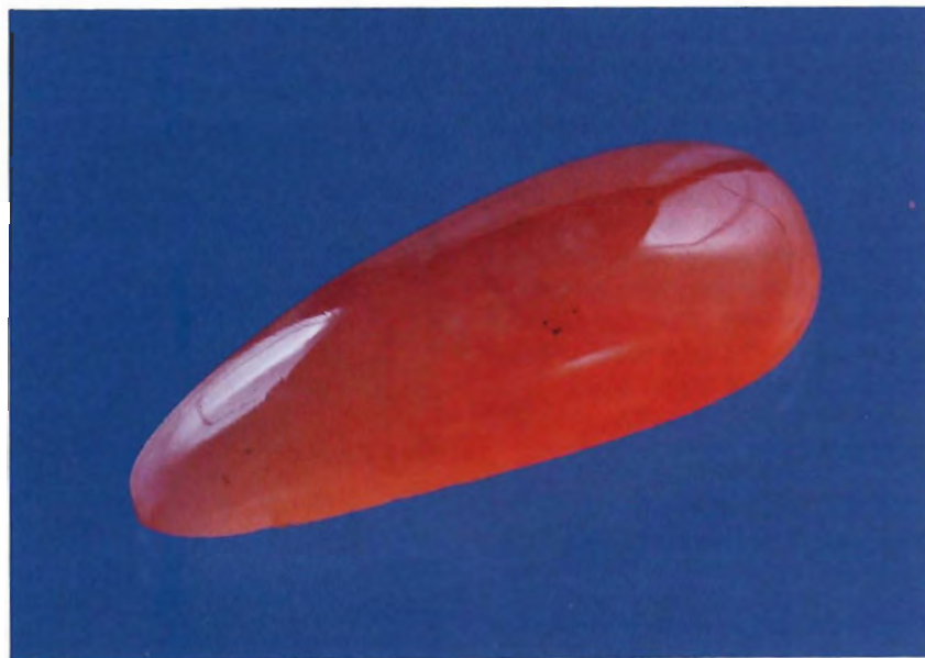
Figure 7. The R.I. and S.G. values of this 8.57-ct hydrogrossular garnet (20.7 × 7.3 × 6.1 mm) are at the low end of the range for this gem species.
