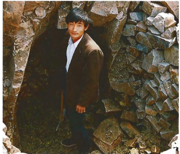
Figure 6. At the digging site at Fangshan (see figure 5), sapphires are concentrated in a xenolith-rich band of unknown thickness (2 m is visible) within the basalt. This was the only in situ operation at the time of the authors' 1989 visit, and was exploited solely for mineral specimens of sapphire in basalt. Mr. Shao Zhixin, a local resident, is shown looking for such specimens.
