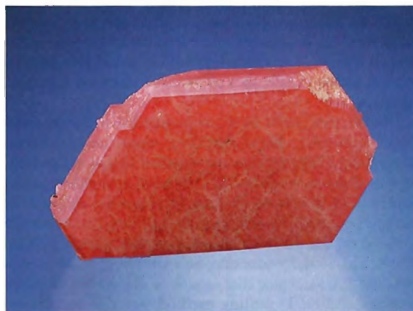
Figure 13. The hydrothermal method was used to synthesize this extremely large (1,930 ct; 95.30 \times 55.05 \times 19.78 mm) ruby crystal in the mid-1960s. Courtesy of Dr. Roch Monchamp; photo by Shane F. McClure.
