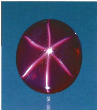
Figure 14. The combination of a high degree of transparency and a reddish purple body color makes this 7.08-ct synthetic star sapphire unusual.
