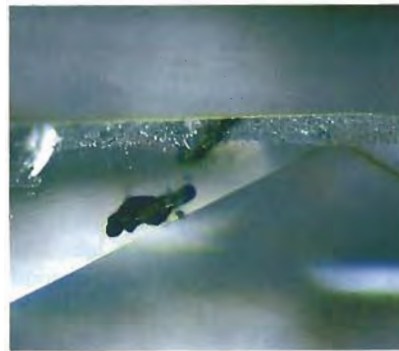
Figure 6. Green stains line the etch cavities that extend into this 0.60-ct marquise-cut diamond and may contribute to its overall color. Magnified 50 \times .
