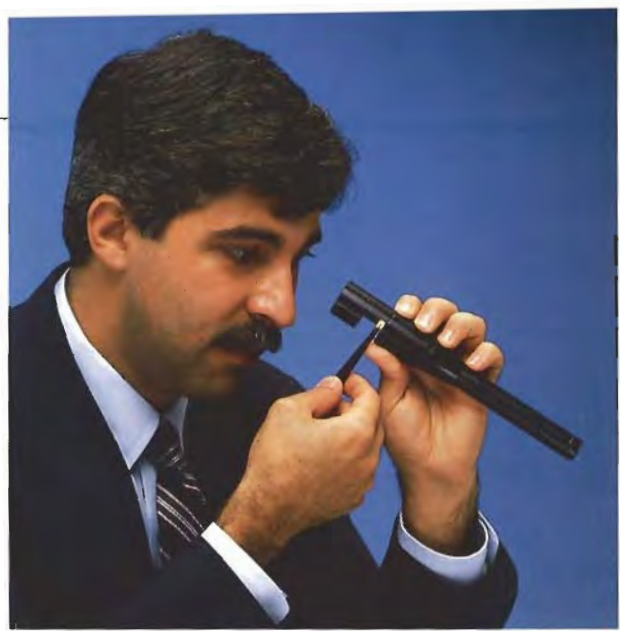
Figure 19. The GIA GEM Instruments' Darkfield Loupe combines true darkfield illumination with a 10× magnifier.
