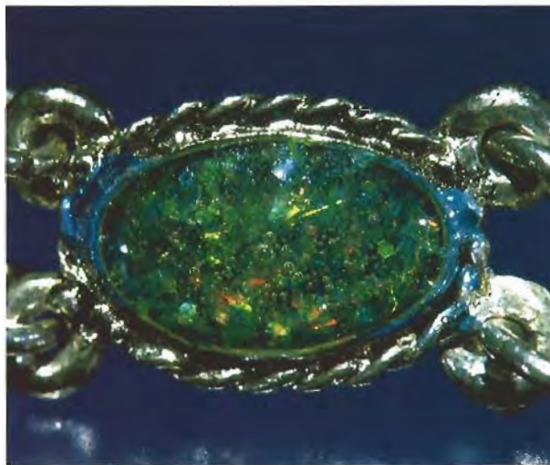
Figure 18. The cabochon seen here in a bracelet from Thailand is a plastic imitation of opal. Note the telltale spherical bubbles. Photo by Maha Smith.
