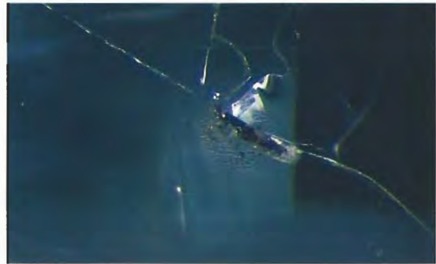
Figure 13. Rapid polishing of the prongs that held this Opticon-treated beryl resulted in abrasion of the hardened Opticon at the surface of the stone. Photomicrograph by John I. Koivula; magnified 50 \times .
