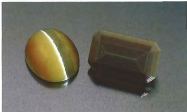
Figure 16. When this 4.13-ct ( 10.70 \times 6.39 \times 6.00 mm) "Fiber Eye" glass was faceted, the optic fibers were oriented perpendicular to the table, so that the back facets appear to be "projected." A typical cabochon is shown for comparison. Photo by Robert Weldon.
