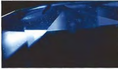
Figure 16. The unusual wisps and veils in this cobalt-colored synthetic spinel appeared to be associated with strain patterns. Magnified 50 \times .
