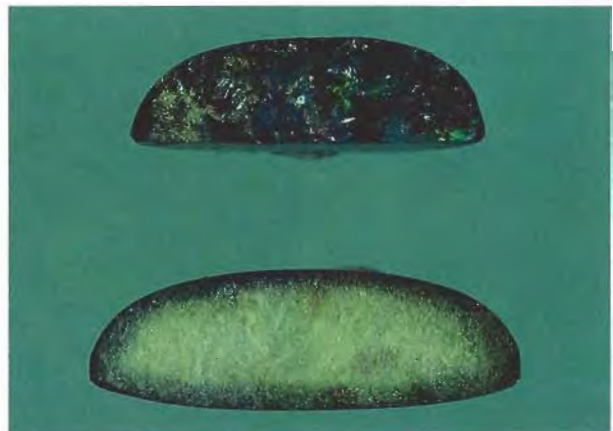
Figure 6. In most cases, the carbon treatment penetrates the matrix opal only at the surface of the prepolished stone. Here, the chipped surface of the cabochon at top reveals the whitish color of the original matrix opal. Cut lengthwise, the cabochon at the bottom graphically illustrates the relatively shallow depth of penetration of the carbon.
