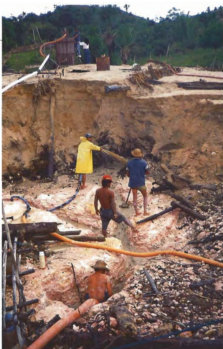
Figure 3. A hydraulic cannon loosens the sediment prior to separation at this alluvial mining operation in northern Brazil. Photo by Patricia Maddison.
