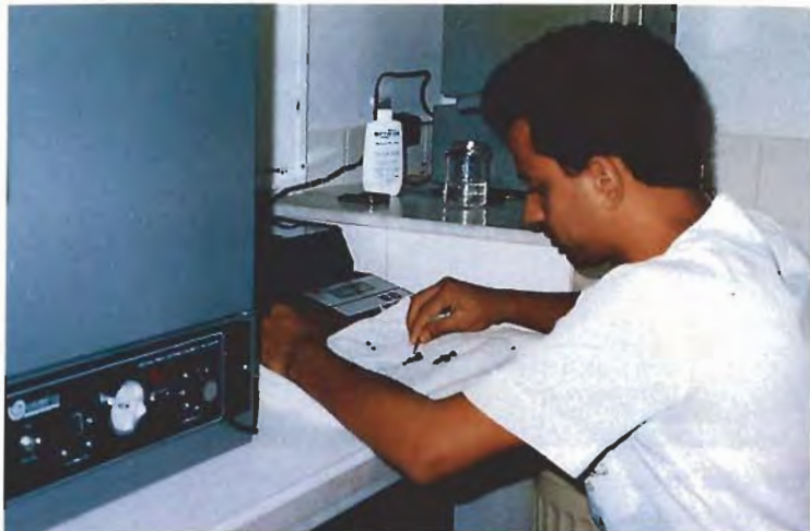
Figure 3. Treatment at Stone World, in Teófilo Otoni, Brazil, begins immediately after cutting. The stones are first cleaned in weak hydrochloric acid, rinsed in water, and—as shown here—examined to make sure that any polishing compound or residual fillers (used on the rough) have been removed. Photo courtesy of Stone World.
