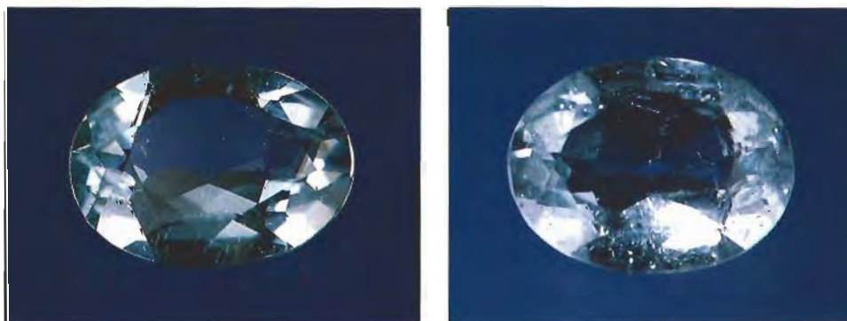
Figure 11. Before steam cleaning, no major fractures were evident in this 2.83-ct Opticon-treated aquamarine (left). Steam cleaning for 15 minutes resulted in partial removal of the Opticon, making the fractures readily apparent (right). Photos by Maha Smith.
