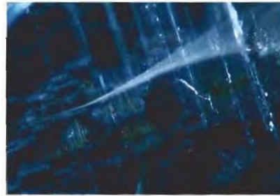
Figure 17. "Internal lightning" reveals damage in a topaz treated by electron irradiation. Magnified 20 \times .
