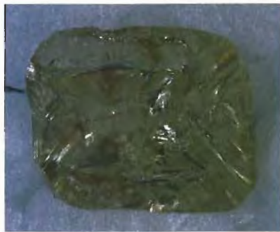
Figure 4. Even after a diamond with what appeared to be a green "skin" was sawed, the green surface color was still prominent. The 6.56-ct piece is shown here.
