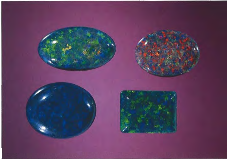
Figure 1. A variety of appearances result from carbon impregnation ("sugar treatment") of Andamooka matrix opal. These treated samples range from 4.73 to 13.69 ct. Photo © GIA and Tino Hammid.
