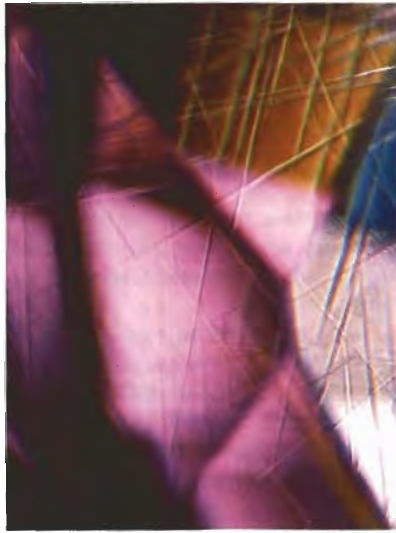
Figure 13. These needle-like inclusions were seen in the spinel shown in figure 12. Magnified 25×.
