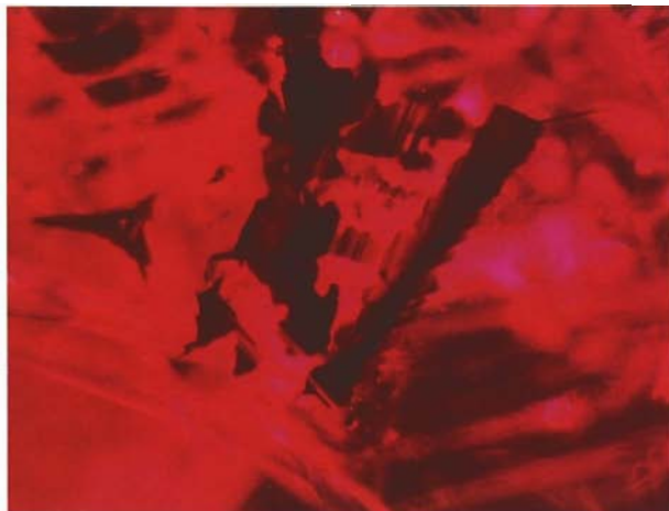
Figure 12. These dark reddish brown inclusions were the only gemological evidence of the flux growth of the synthetic spinel crystal shown in figure 11. Photomicrograph by John I. Koivula; magnified 35×.
