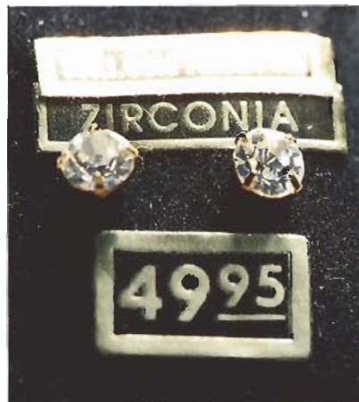
Figure 17. These 5-mm "zirconia" earrings were found to be foil-backed glass.
