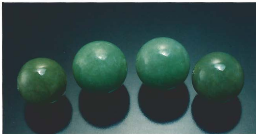
Figure 9. Although all four of these 9-mm jadeite beads were impregnated with plastic, the treatment was more successful on the inner pair than on the outer two.
