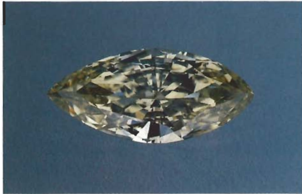
Figure 4. The light yellow tips and near-colorless center give this 0.69-ct marquise-shaped diamond the distinctive appearance of a true bicolor.
