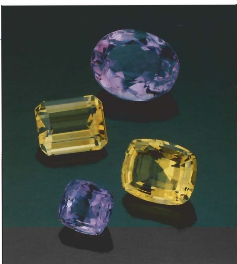
Figure 1. The separation of scapolite (right and bottom) and quartz (top and left), may be difficult to perform using standard gemological testing but is accomplished in a matter of minutes with reflectance infrared spectroscopy. Photo © Tino Hammid.
