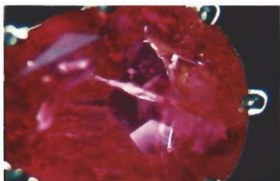
Figure 14. The numerous fractures in this natural ruby (8.60 × 6.20 × 3.80) probably resulted when the stone was heated during a retipping of the prongs. Magnified 10×.
