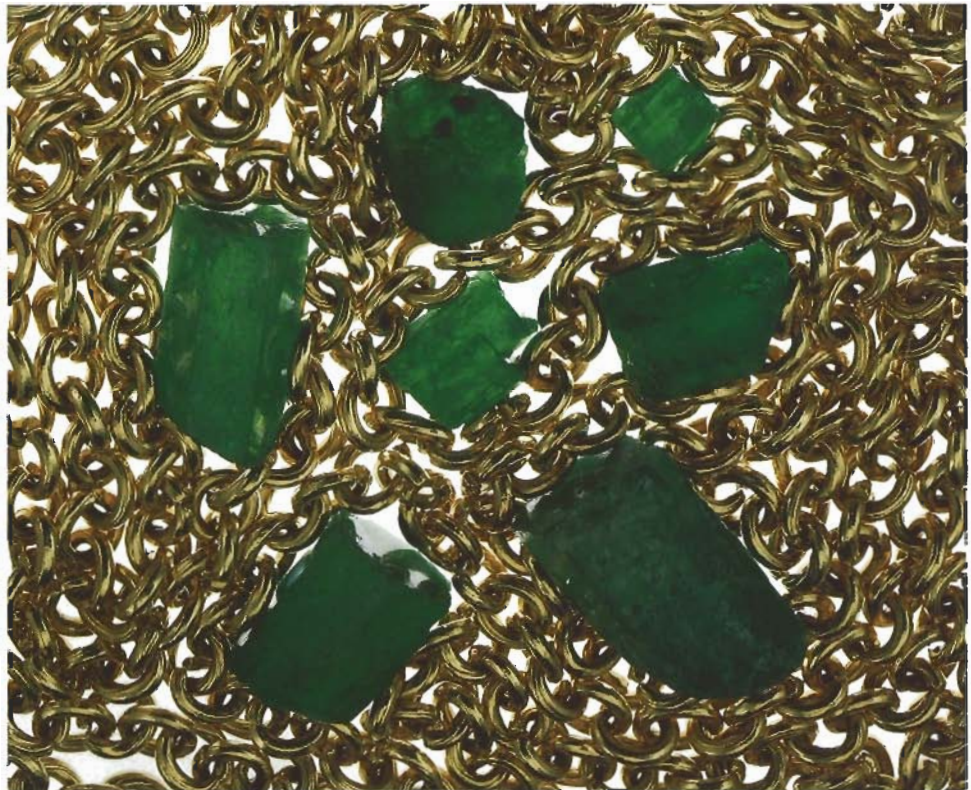
Figure 5. The seven emerald crystals examined (3.69–64.46 ct) ranged from transparent to translucent and from green to slightly bluish green. The chain surrounding the crystals is one of many from the Atocha wreck site. It has been suggested that the chains were worn as jewelry to try to escape taxation; individual links could be removed and used as coinage (Lyon, 1982). Note the draw lines on the links, evidence of the relatively crude technique used. Photo by Shane F. McClure.
