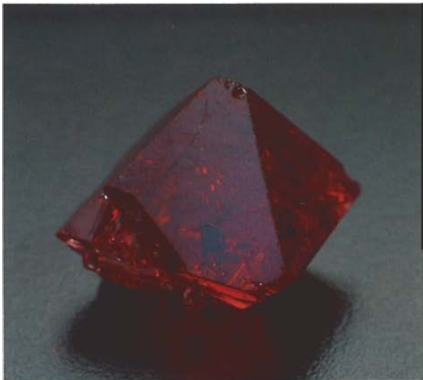
Figure 11. Reportedly manufactured in the Soviet Union, this 17.19-ct synthetic spinel crystal was flux grown. Photo by Robert Weldon.
