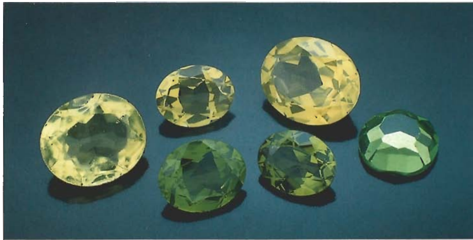
Figure 1. Some of the radioactive stones tested include, from left to right: back— LE_5 (a rhinestone), GR_1 and LE_2 (synthetic spinel-glass triplets); front— GO_1 and GR_2 (synthetic spinel-glass triplets), SW_2 (a chaton). Photo by Robert Weldon.
