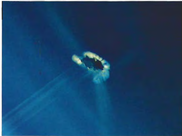
Figure 6. The Penglai blue sapphire shown in figure 4 also contained a small brown crystal surrounded by a tension halo and trailed by a "comet tail." Oblique illumination; magnified 40 \times . Photomicrograph by Robert E. Kane.
