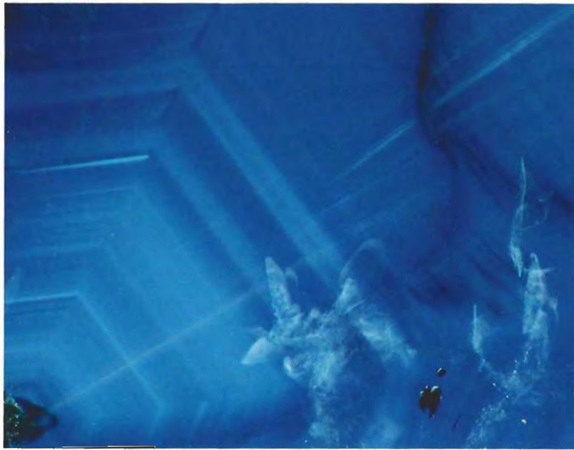
Figure 5. A view of the base of the Penglai blue sapphire crystal shown in figure 4 (after it had been partially polished) reveals prominent angular growth zoning as well as "fingerprints" and stringers of rutile "comet tails." The growth zoning, evidence of the changes that took place in the chemical environment as the sapphire crystal grew, represents a combination of color zoning and varied concentrations of fine particles of rutile. Fiber-optic illumination; magnified 15 \times . Photomicrograph by Robert E. Kane.
