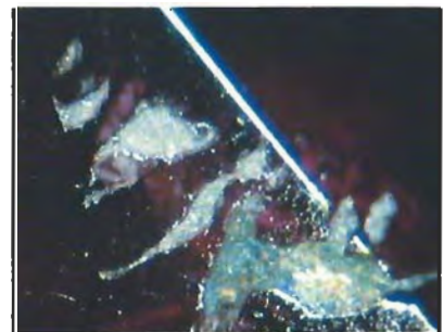
Figure 11. Flux inclusions break the surface of this 2.65-ct synthetic ruby. Magnified 20×.
