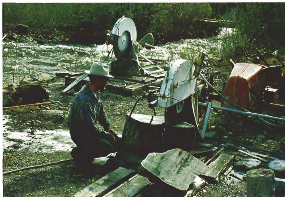
Figure 6. A circular diamond saw is used to cut sections from a nephrite boulder at the Dahl Creek mine. Photo by Mrs. Ivan Stewart.
