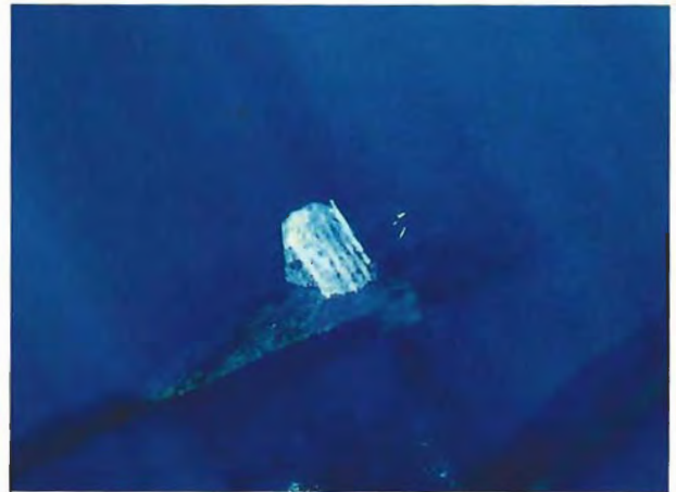
Figure 7. This white crystal, set against a backdrop of dense rutile particles and color zoning, was also observed in the Penglai blue sapphire shown in figure 4. Oblique illumination; magnified 40 \times . Photomicrograph by Robert E. Kane.
