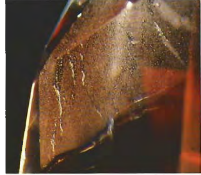
Figure 16. A very fine-grained fingerprint inclusion was observed in one of the triphylite specimens at 35× magnification.
